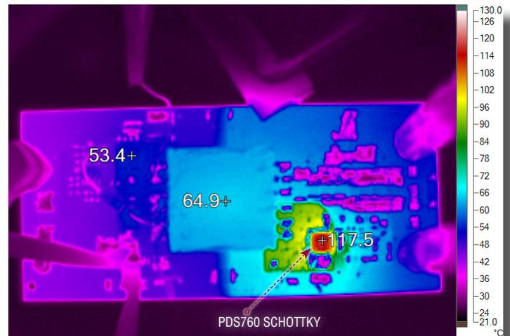
Figure 3. Thermal image at 5V/5A output with diode PDS760
