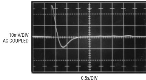
**Figure 2: Optimized gain-bandwidth results in nearly critically damped response with settling in 1.5 seconds**
