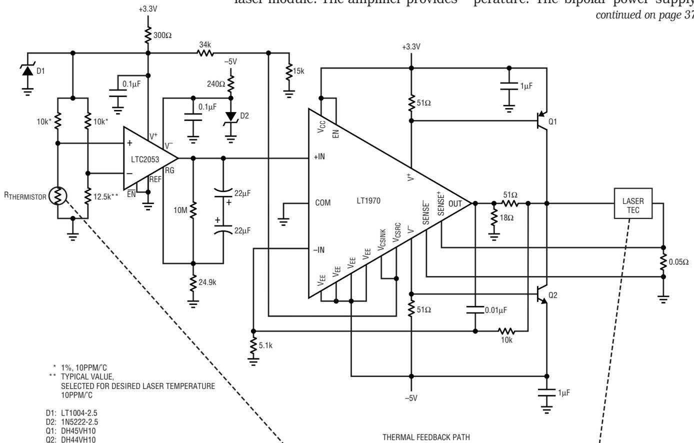
**Figure 1. Two amplifiers form a thermoelectric temperature cooler for a fiber optic laser module. The linear approach eliminates inductors. As low as 0.01°C control stability over a wide ambient temperature swing is achievable.**
