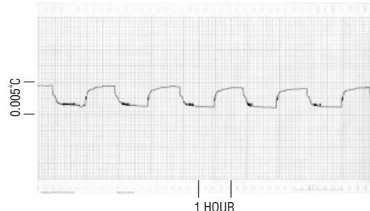
**Figure 3. 10-hour cooling mode stability measured in an environment that steps 20 $^{\circ}$ C above ambient every hour. Data shows the resulting 0.0035 $^{\circ}$ C peak-to-peak variation, indicating a thermal gain of 5700.**
