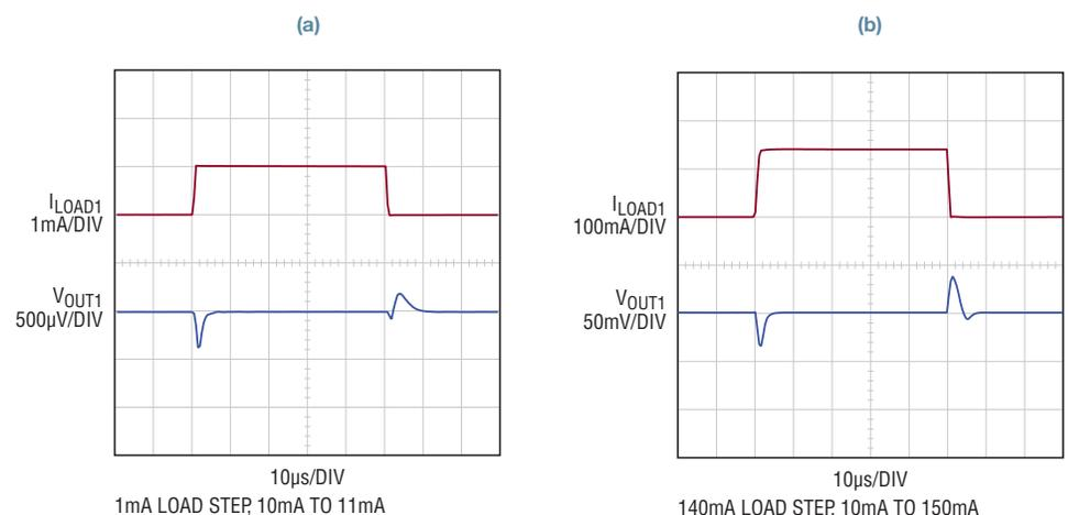
The LT6658 is a precision low noise, low drift regulator featuring the accuracy specifications of a dedicated reference and the power capability of a linear regulator. The LT6658 boasts 10ppm/°C drift and 0.05% initial accuracy, with two outputs that can support 150mA and 50mA, respectively, each with 20mA active sinking capability.
