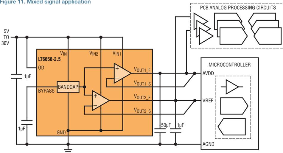
The LT6658 is well suited to industrial environments since it can operate with noisy supply rails and where load glitches due to conversions on one output have little influence on the adjacent output. Moreover, when a load demands current on one output, the adjacent output continues to track.
