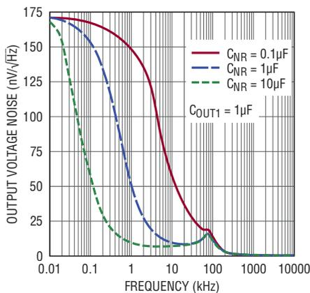
pin. A capacitor on the NR pin forms a low pass filter with an on-chip  $400\Omega$  resistor. A large capacitor lowers the filter frequency and subsequently, the total integrated noise. Figure 8 shows the effect of increasing the values of the capacitor on the NR pin. With a  $10\mu\text{F}$  capacitor the noise rolls off to about  $7\text{nV}/\sqrt{\text{Hz}}$ .
