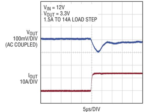
Figure 4. Load transient response of the Figure 2 solution
