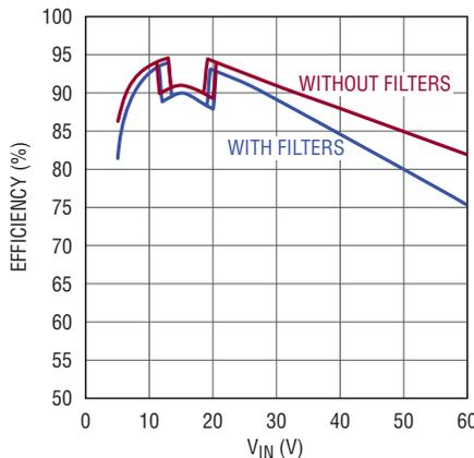
Figure 2. Efficiency of LED driver solution in Figure 1. Measurements made using 16V, 1.5A, demonstration circuit DC2575A LED driver with and without optional EMI components
