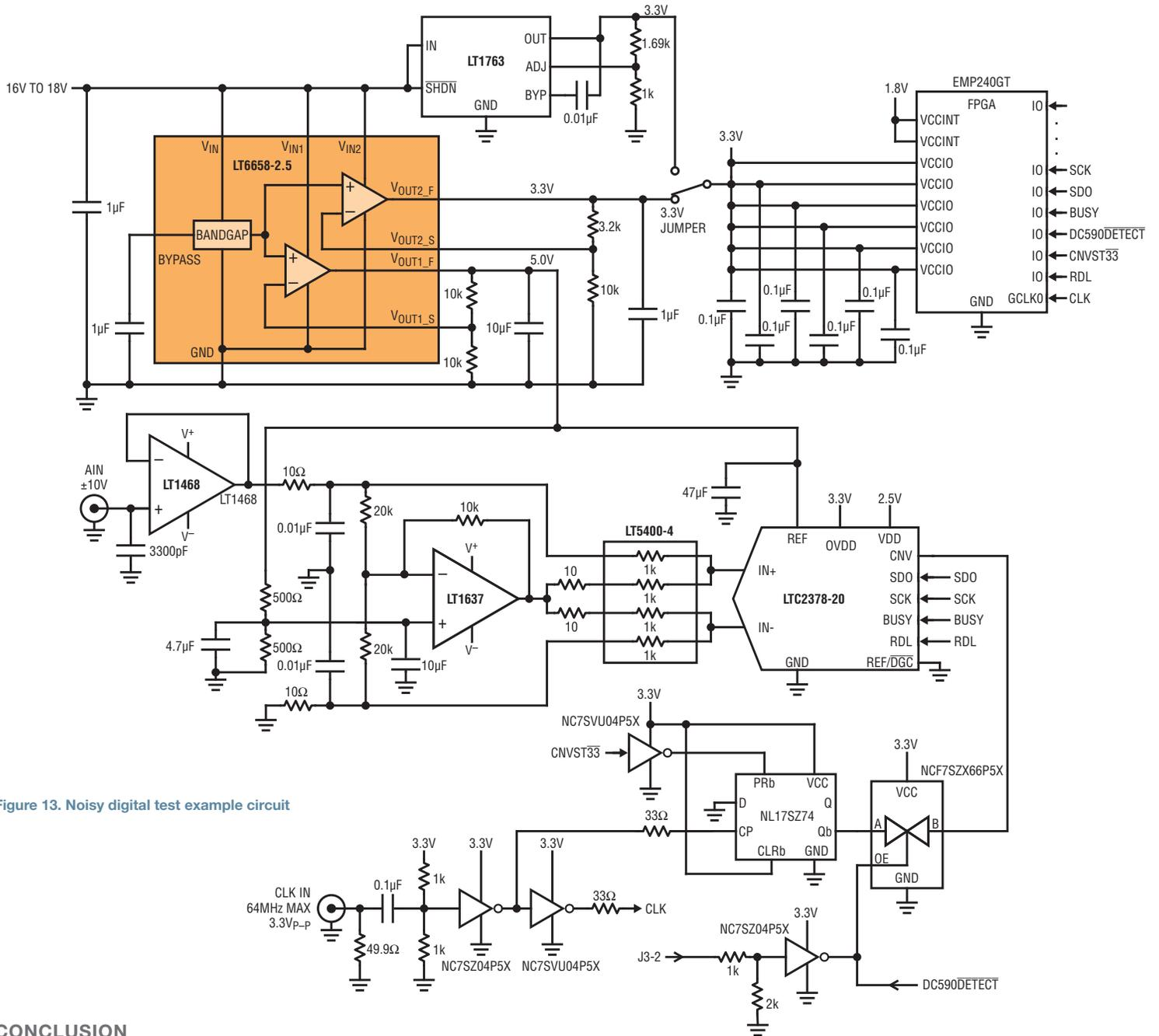
Figure 13. Noisy digital test example circuit
