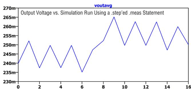
Use LTspice to zero in on worst-case performance by exploring the tolerance limits of components. Here, 16 possible parameter combinations of four resistor values—at their tolerance limits—are simulated and graphed. The effects of tolerance are clearly shown.
