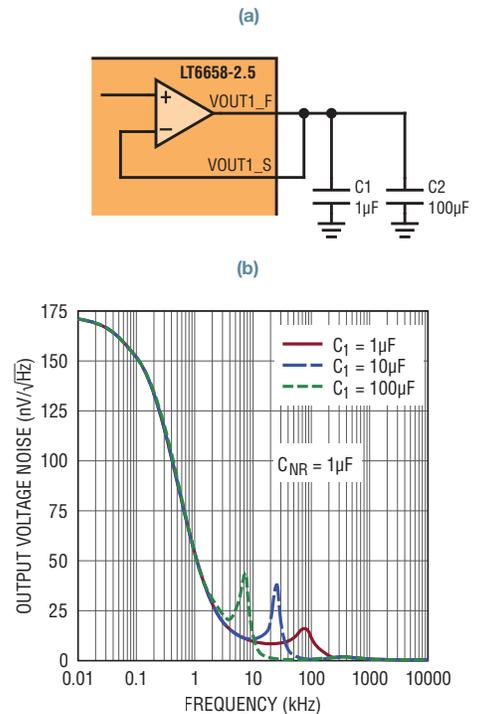
By increasing the output capacitor, the noise can be further reduced. When both the NR and output capacitors are increased, the output noise can be reduced to a few microvolts. The LT6658 is stable with output capacitance between 1 $\mu$ F and 50 $\mu$ F.
