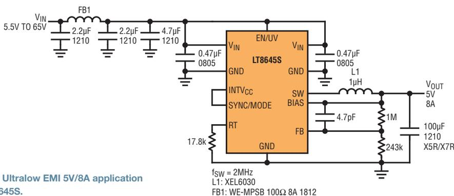
Figure 10. Ultralow EMI 5V/8A application using LT8645S.
