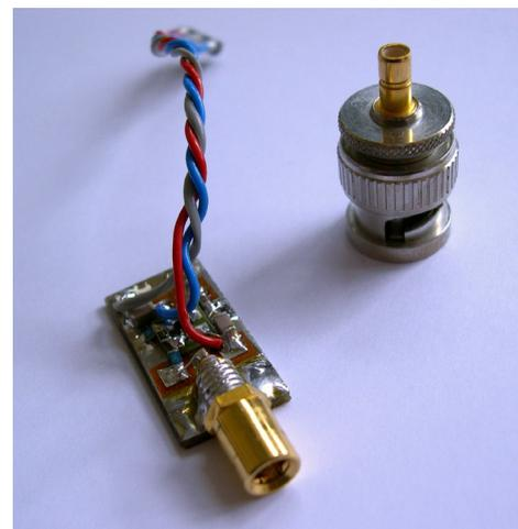
Figure 2. Prototype pocket-size white noise generator
