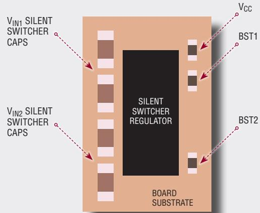
Silent Switcher 2 devices integrate the hot loop and warm loop caps into the package to simplify board layout.
