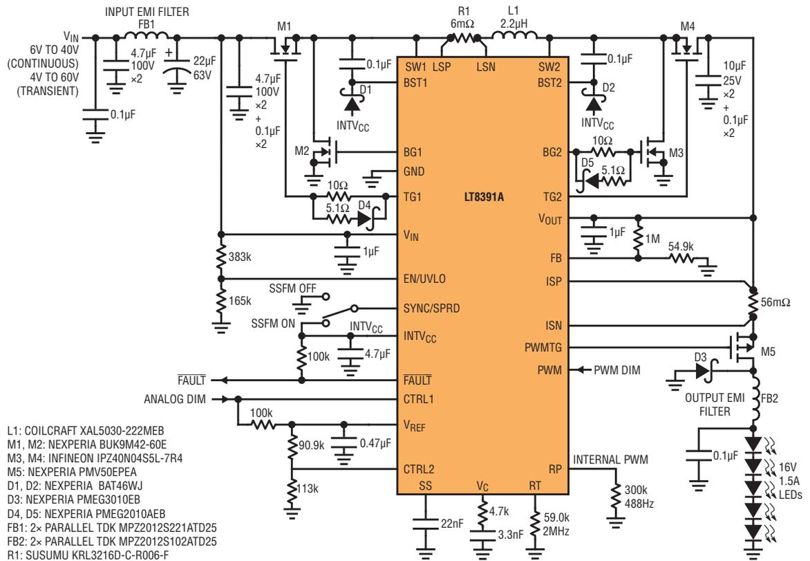
of the critical input and output hot loops—reducing EMI. Optional spread spectrum frequency modulation (SSFM) further reduces the controller’s EMI.
