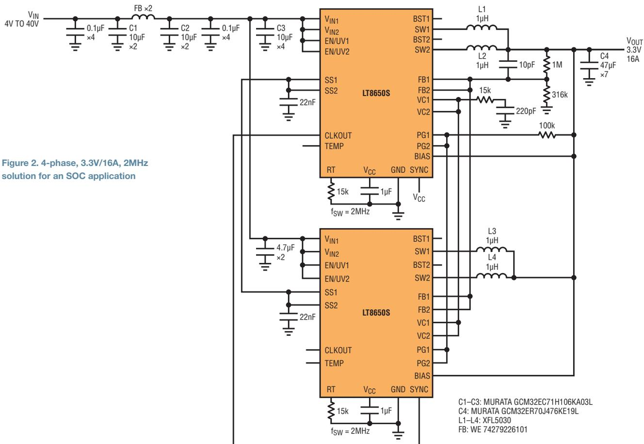
These monolithic ICs have integrated MOSFETs and they can run at greater than 2MHz, resulting in reduced solution size and cost while avoiding the AM band.
