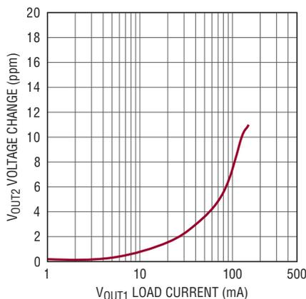
Figure 3. Channel-to-channel load regulation (effect of heating removed)
