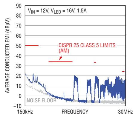
Figure 3. LT8391A demonstration circuit DC2575A passes CISPR 25 Class 5 automotive radiated EMI
