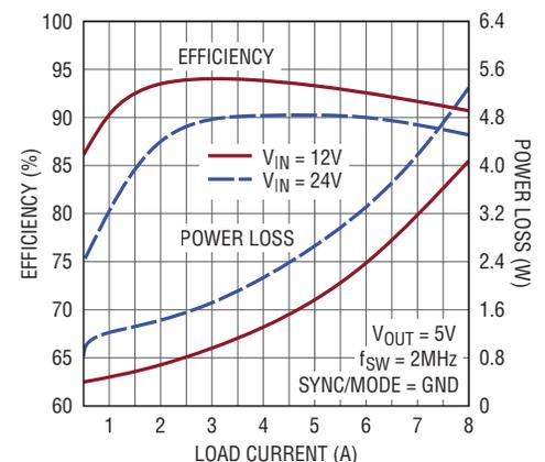
Figure 11. LT8645S efficiency for the ultralow EMI solution
