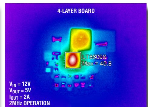
Thermal performance is another concern when fewer board layers are used, but is not a problem for the LT8609S. Silent Switcher 2 technology means lower noise level and greater efficiency, with less power loss generated from switching transitions.
