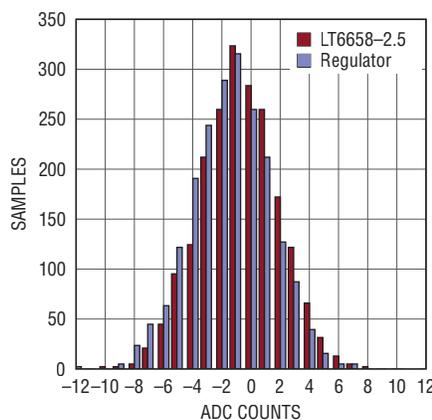
Figure 14. Histogram test results of the circuit in Figure 13
