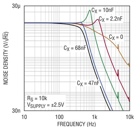
Figure 4. Output noise density of design in Figure 1
