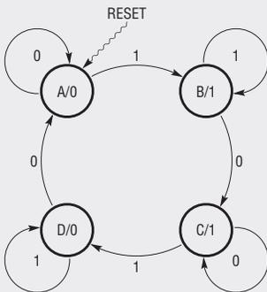
Each state of the state machine is defined using a `.state` command. The first state listed is the initial state, otherwise the order of the states makes no difference. The name of the state can be anything and the output of the state is defined by a value.
