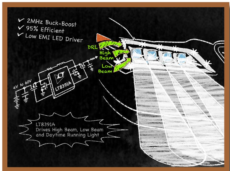
inductor and small overall solution size for high power LED applications. Unlike monolithic converters, whose power switches are contained within the IC package, controllers such as the LT8391A can drive external power switches with much higher peak currents, such as 10A. Such peak currents would burn up the small IC packages of typical integrated
