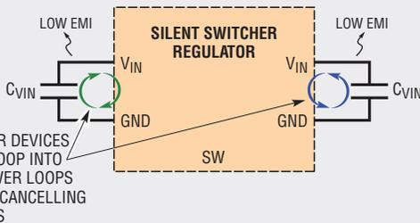
SILENT SWITCHER DEVICES SPLIT THE HOT LOOP INTO TWO LOWER POWER LOOPS WITH MUTUALLY CANCELLING MAGNETIC FIELDS
