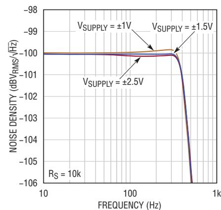
Figure 6. Output noise density for various supply voltages
