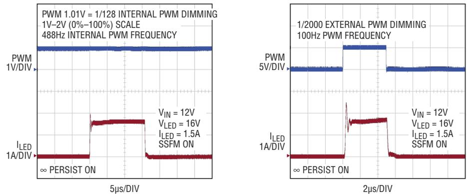
Figure 8. PWM dimming using internal and external PWM options; 1% and 0.05%, respectively
