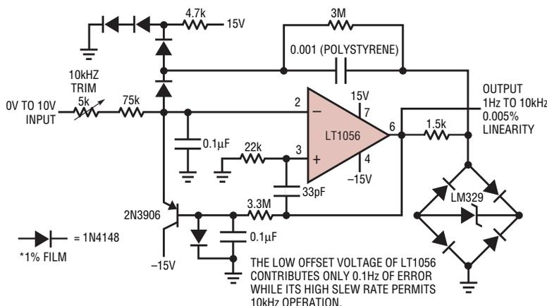
Figure 1. Precision: 1Hz to 10kHz voltage-to-frequency converter
