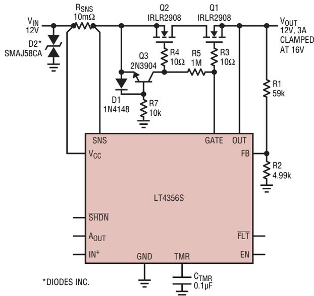
Figure 6. Redundant pass transistors
