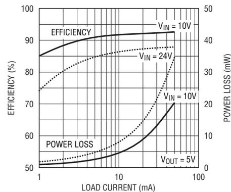
Figure 4. Efficiency for circuit in Figure 3
