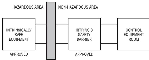
Figure 2. Isolation/protective barrier location
