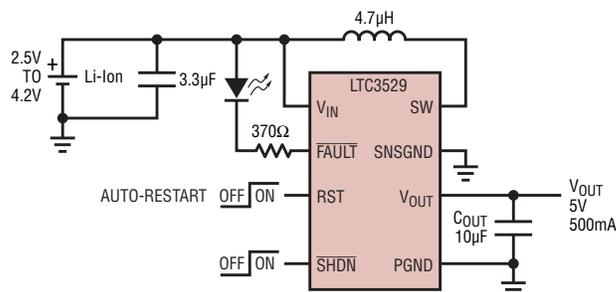
Figure 2. Li-Ion to 5V synchronous boost converter
