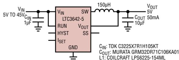
Figure 3. With the LTC3642EDD-3.3/5 only two capacitors and an inductor are required for operation
