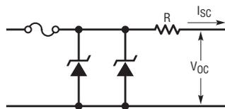
Figure 3. Simple passive component barrier
