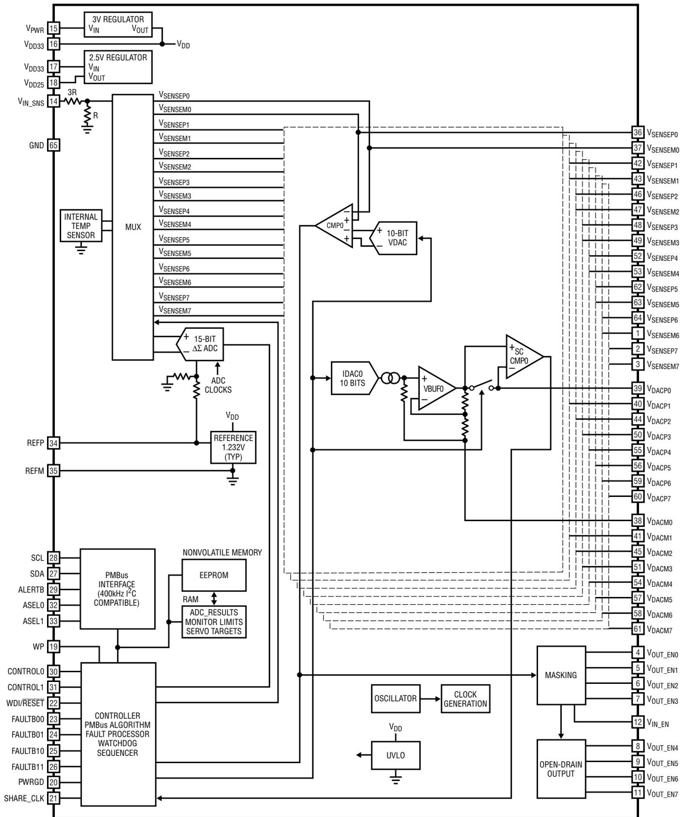
Figure 4. Block diagram of the LTC2978
