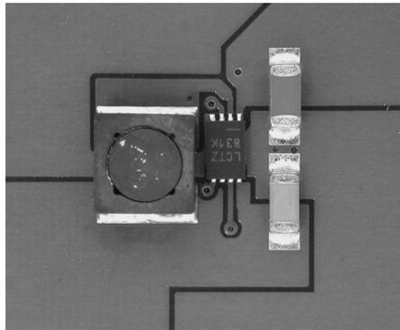
Figure 1. A tiny (1cm<sup>2</sup>) yet complete solution drives USB On-The-Go bus power.
