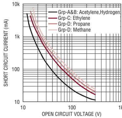
**Figure 4. Resistive circuit spark ignition curves**
