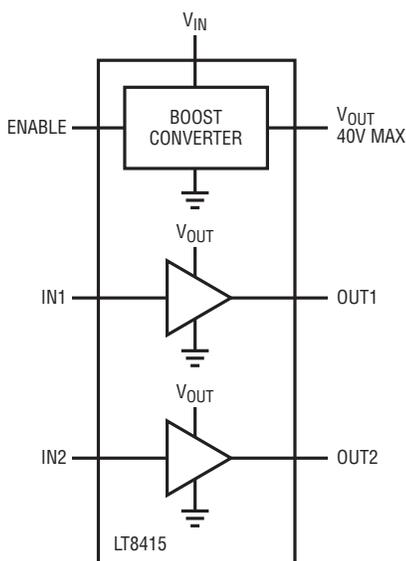
Figure 1. Simplified block diagram of the LT8415
