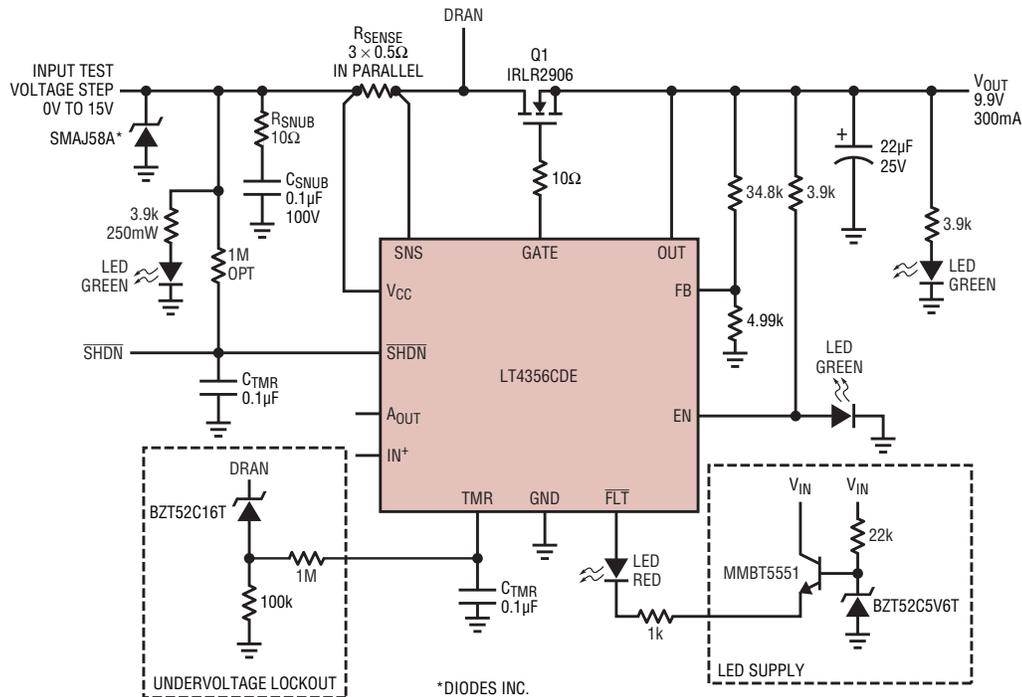
**Figure 7. Schematic of a modified DC1018A evaluation board**
