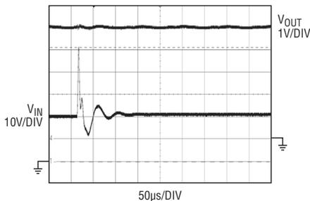
Figure 1. The LTC3642 continues to regulate the output despite a >45V spike on the input.
