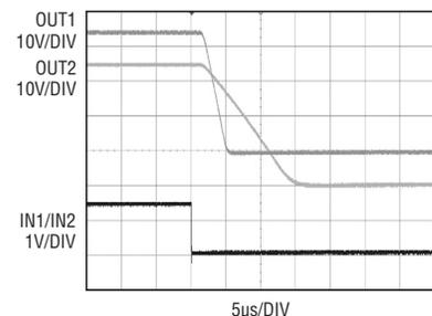
Figure 4. Turn-off delay and fall time for OUT1 and OUT2
