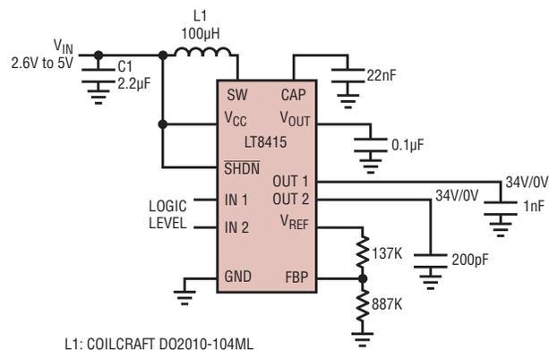
Figure 2. 2.6V–5V input to 34V dual half-bridge boost converter
