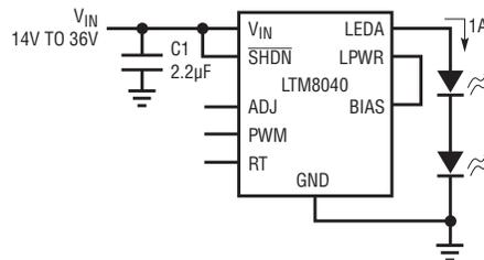
**Figure 1. Driving an LED string with the LTM8040 is simple—just add the input capacitor and connect the LED string**
