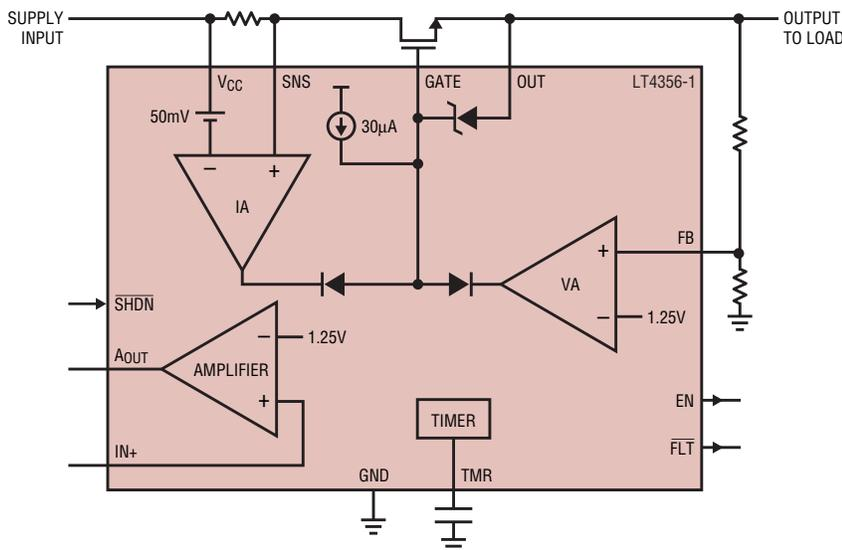
**Figure 5. Simplified block diagram of the LT4356**
