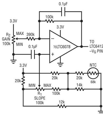
**Figure 12.** Thermistor-based application circuit for static gain adjust and temperature gain slope compensation. Adjust R1 and R2 as needed and route output to -V<sub>G</sub> control terminal of the LTC6412.
