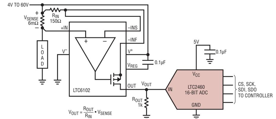
**Figure 1. A simple and compact high side current sensing solution that combines a high resolution  $\Delta\Sigma$  ADC (LTC2460) with a high precision current sensing amplifier (LTC6102).**
