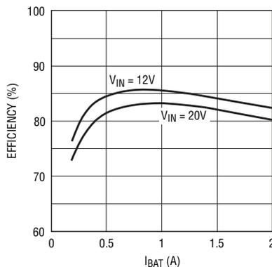
**Figure 4. Power conversion efficiency vs charger output current (I<sub>BAT</sub>) for the battery charger shown in Figure 2**
