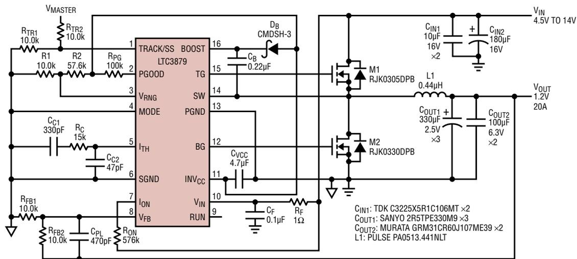
Figure 6. Coincident tracking example produces 1.2V at 20A, operating at 300kHz
