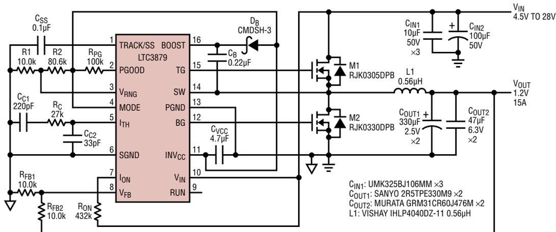
Figure 5. Wide input range to 1.2V at 15A, operating at 400kHz
