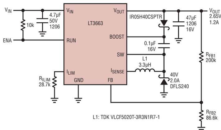
Figure 2. Capacitor charger circuit using the LT3663
