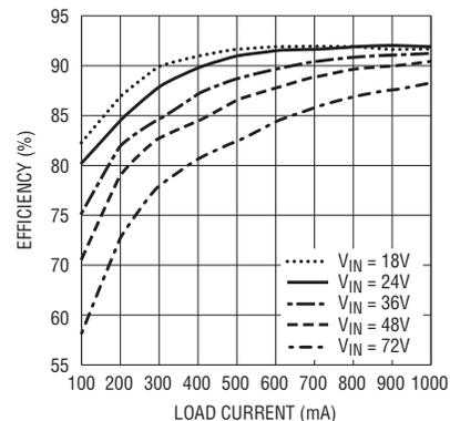
**Figure 6. Efficiency of the converter in Figure 5**
