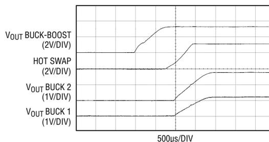
Figure 8. Power-up sequencing, buck-boost followed by the buck outputs
