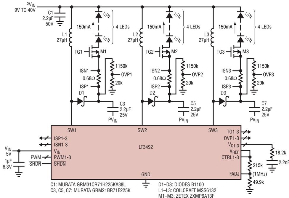
Figure 4. Triple buck-boost mode 150mA × 4 LED driver
