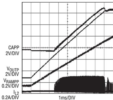
Figure 8.  $V_{OUTP}$  soft-start ramping from ground
