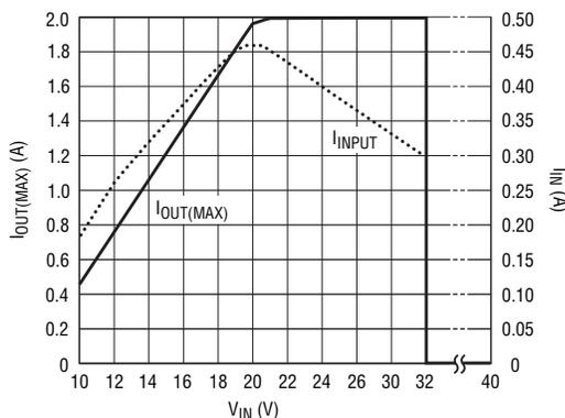
**Figure 8.** Charger maximum input current ( $I_{\text{IN}}$ ) and maximum output current ( $I_{\text{OUT(MAX)}}$ ) vs  $V_{\text{IN}}$  for the battery charger shown in Figure 7. Charge current reduction for  $V_{\text{IN}} < 20\text{V}$  keeps the charger input supply current below  $0.5\text{A}$
