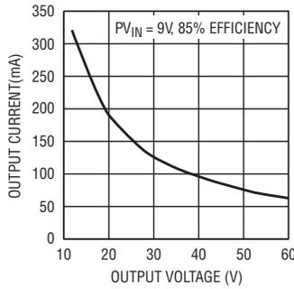
Figure 3. Maximum output current capability of an LT3492 boost circuit
