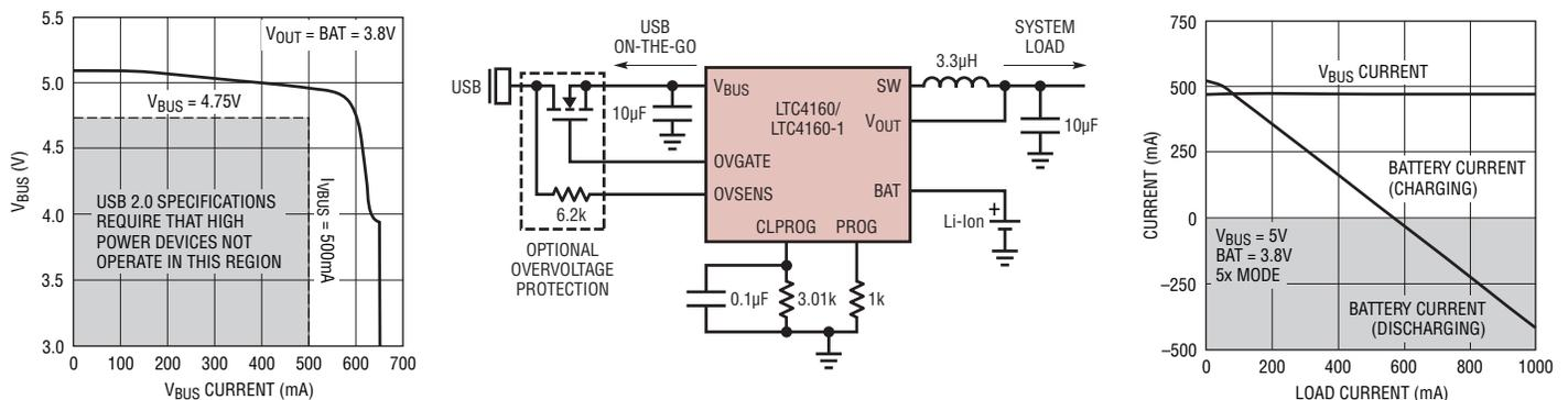
Figure 1. The LTC4160 provides bidirectional power transfer. Left plot:  $V_{BUS}$  voltage vs  $V_{BUS}$  current in On-The-Go mode. Right plot: battery and  $V_{BUS}$  currents vs load current when input power is available.
