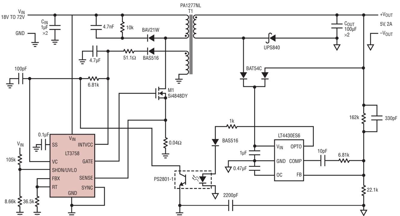
Figure 8. 18V-72V input, 5V/2A isolated flyback converter
