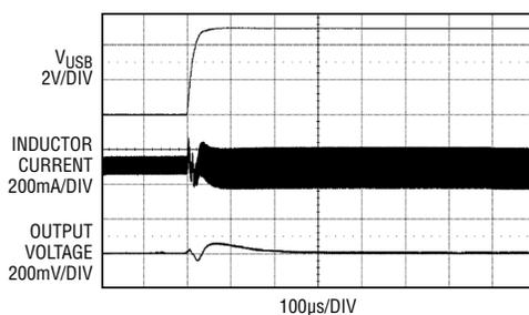
Figure 5. Buck-boost output voltage transient on USB hot plug
