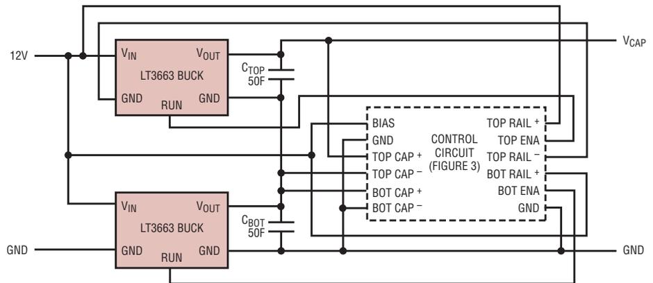
Figure 1. Block diagram for charging two supercapacitors in series
