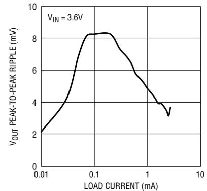
Figure 3. Output peak-to-peak ripple vs load current for Figure 1 converter at 3.6V
