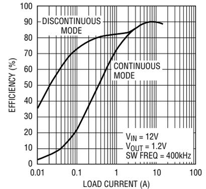
Figure 4. Efficiency for application in Figure 5
