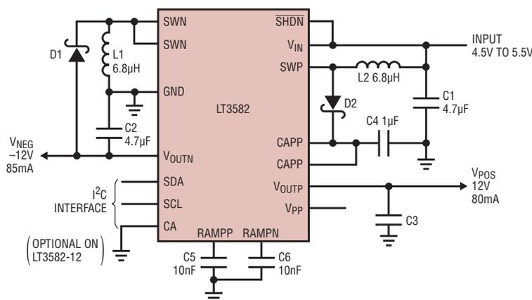
REGO/OTPO = 80h D1-D2: DIODES INC. B0540WS-7 C2: 4.7µF, 16V, X5R, 0805 C4: 1µF, 16V, X5R, 0603
