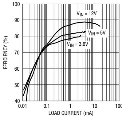
Figure 2. Efficiency vs load current for Figure 1 converter
