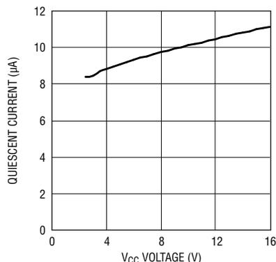
**Figure 5. Quiescent current vs V<sub>CC</sub> voltage (not switching)**
