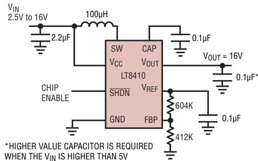
Figure 1. 2.5V-16V To 16V boost converter
