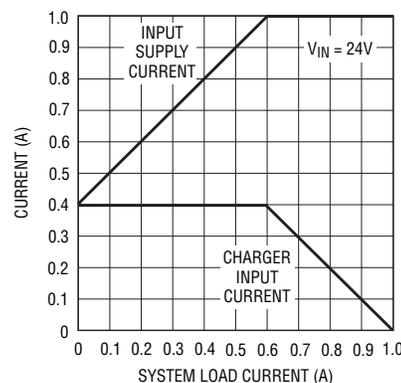
**Figure 9.** Charger maximum input current, system load current, and total input supply current for the battery charger shown in Figure 7 for  $V_{\text{IN}} = 24\text{V}$ . Battery charger output current is reduced to maintain a maximum input supply current of  $1\text{A}$ , which corresponds to  $50\text{mV}$  across the  $0.05\Omega$  resistor that is connected between the CLP and  $V_{\text{IN}}$  pins of the LT3650.
