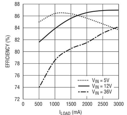
Figure 4. Efficiency of the converter in Figure 3
