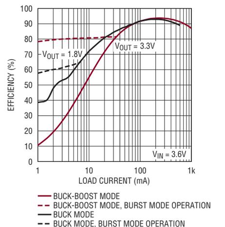
Figure 3. Efficiency vs load current for the circuit in Figure 2
