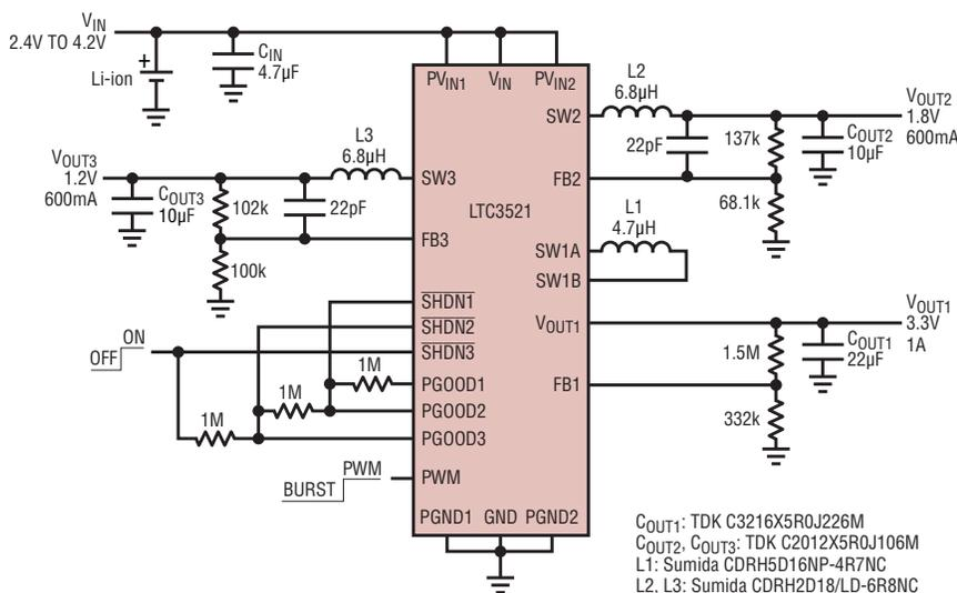
Figure 2. A 3-output converter takes a single Li-Ion battery to 3.3V at 1A (buck-boost mode), 1.8V at 600mA and 1.2V at 600mA.
