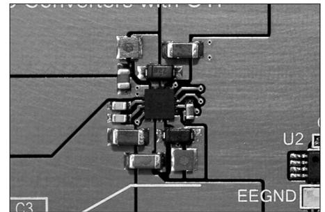
Figure 1. Dual output supplies in a small board footprint
