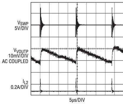
Figure 3. Switching waveforms at 1mA load for the boost application shown in Figure 2
