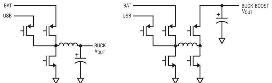
Figure 4. The low loss PowerPath architecture
