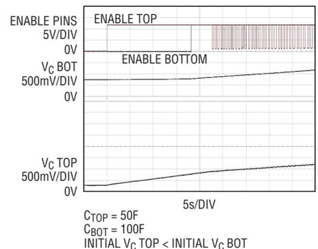
Figure 5. Charging with mismatched capacitors
