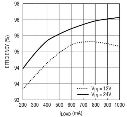
Figure 2. Efficiency of the converter in Figure 1
