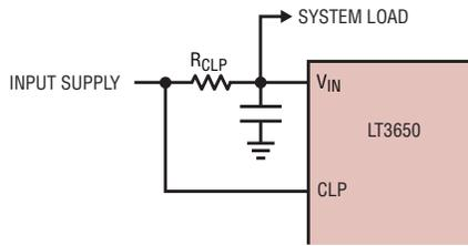
Figure 6.  $R_{CLP}$  sets the input supply current limit
