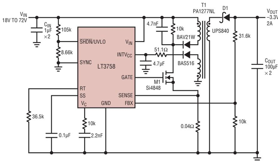
**Figure 7. 18V-72V input, -3.3V/2A output flyback converter**
