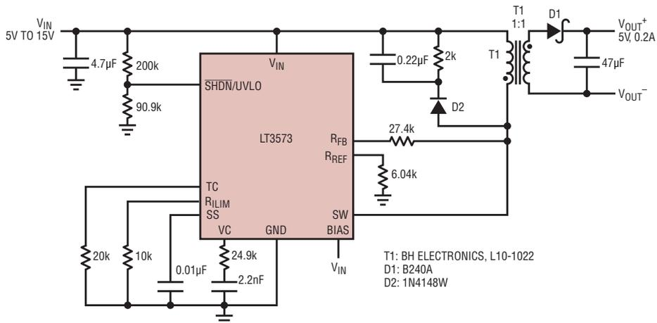
**Figure 1. Amazingly simple flyback converter takes advantage of the primary side sensing scheme of the LT3573. Note the absence of an optocoupler. Also note the tiny coupling inductor available from many magnetics vendors.**
