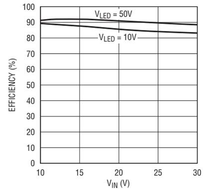
Figure 5. Efficiency for the buck-boost mode converter in Figure 4
