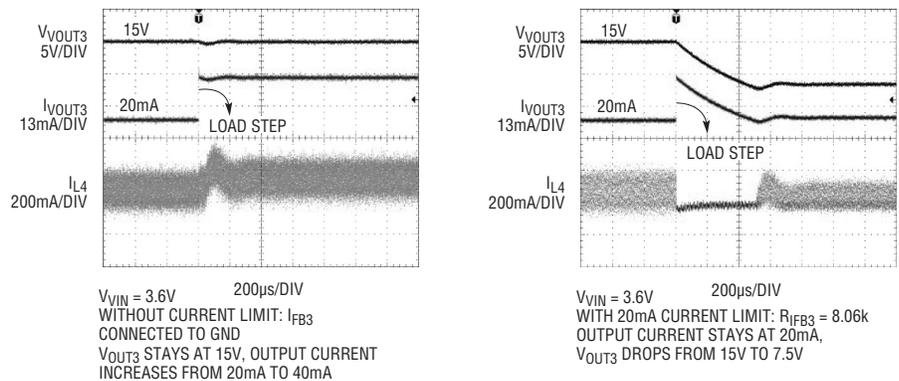
Figure 11. Channel 3 in an output current overload event with and without output current limit
