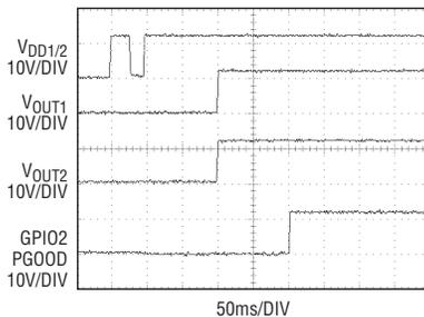
Figure 2. Start-up waveform with coupled turn-on
