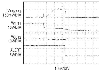
Figure 5. Fault-off waveform with independent faults
