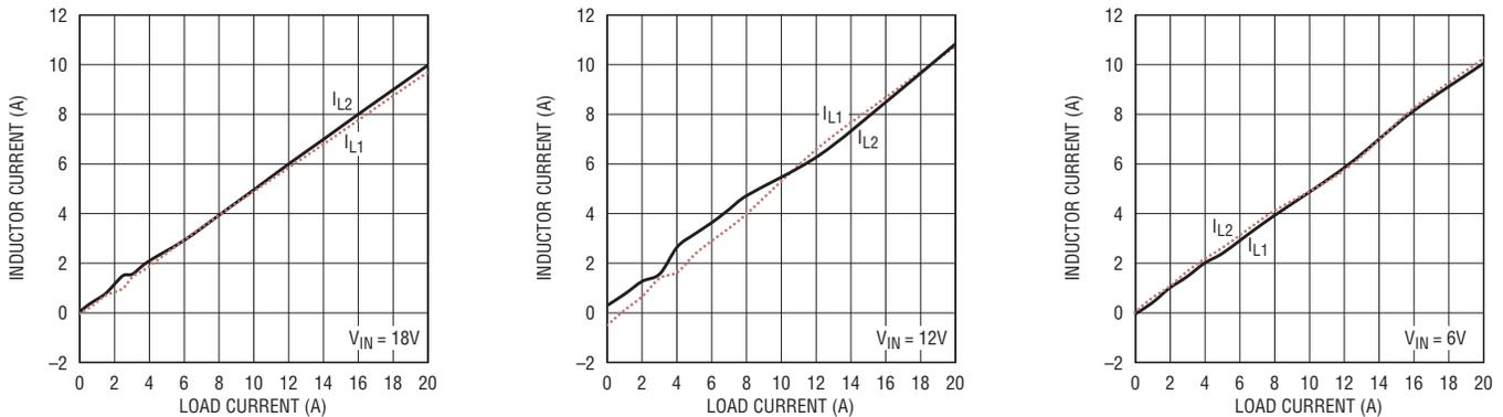
**Figure 3. Balanced inductor currents for two paralleled LTM4605s in different operating modes**
