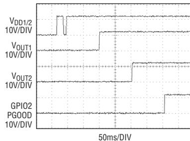
Figure 4. Start-up waveform with sequencing
