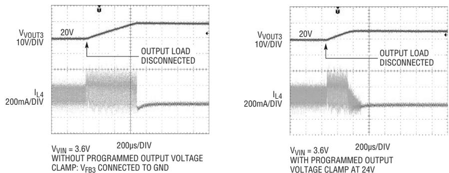
Figure 12. Channel 3 in an output open circuit with and without programmed output voltage clamp
