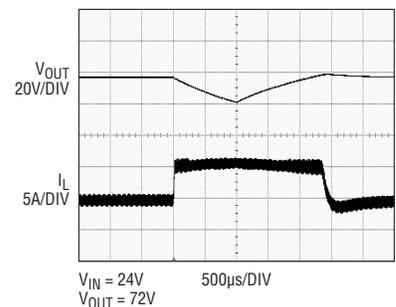
**Figure 9. Load step waveforms for diesel fuel injector actuator supply**
