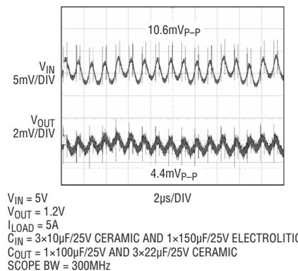
**Figure 8. Input and output noise of LTM4606  $\mu$ Module regulator is significantly lower than the regulator in Figure 7.**
