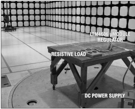
Figure 10. Setup of the radiated emission scan
