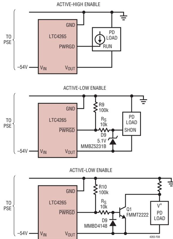
Figure 3. Examples of enabling/disabling the PD load via the complementary power good pins
