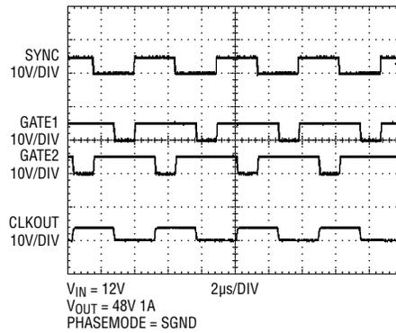
**Figure 7. Synchronizing the LTC3862 to an external clock using the phase lock loop**
