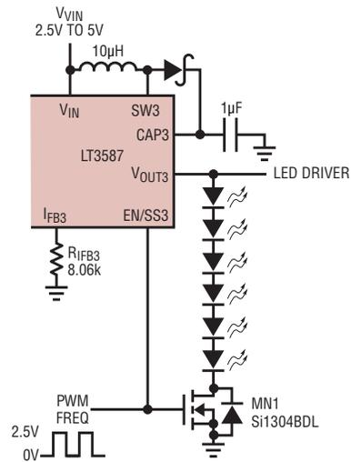
Figure 9. Driver for six LEDs with PWM dimming
