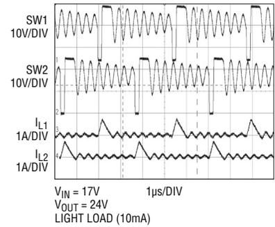
**Figure 6. Inductor and switch node voltage waveforms at light load (pulse-skipping)**
