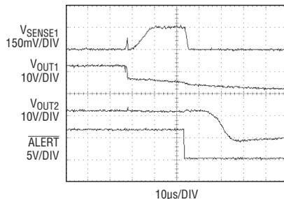
Figure 3. Fault-off waveform with coupled faults
