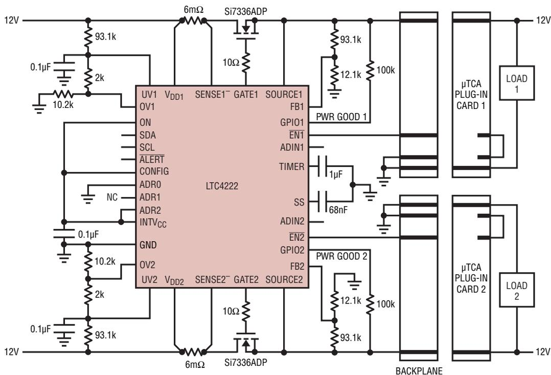
Figure 6.  $\mu\text{TCA}$  application supplying 12V payload power to two  $\mu\text{TCA}$  slots
