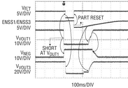
**Figure 6. Fault detection of a short circuit event**
