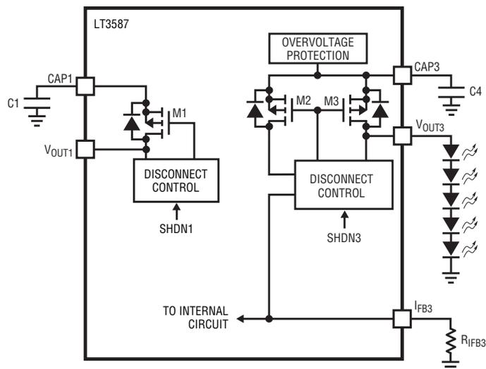
Figure 3. Partial block diagram of the LT3587 showing the disconnect PMOS for channels 1 and 3
