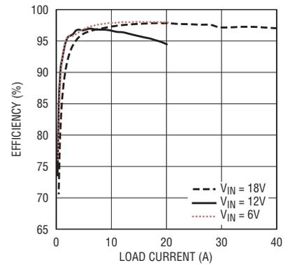
Figure 6. The tested efficiency for the four LTM4605s paralleled in Figure 5 (CCM mode)
