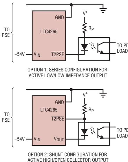
Figure 2. Interfacing with the Type-2 PSE via the T2PSE pin
