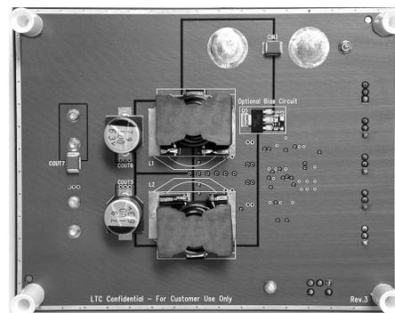
**Figure 13. 48V/5A output, high power demonstration circuit**
