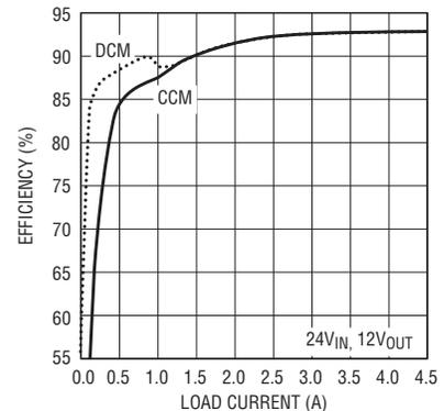
**Figure 4. Efficiency for the circuit in Figure 3.**
