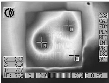
**Figure 5. Thermal image of an LTM4606 with 24V input and 3.3V output at 6A**
