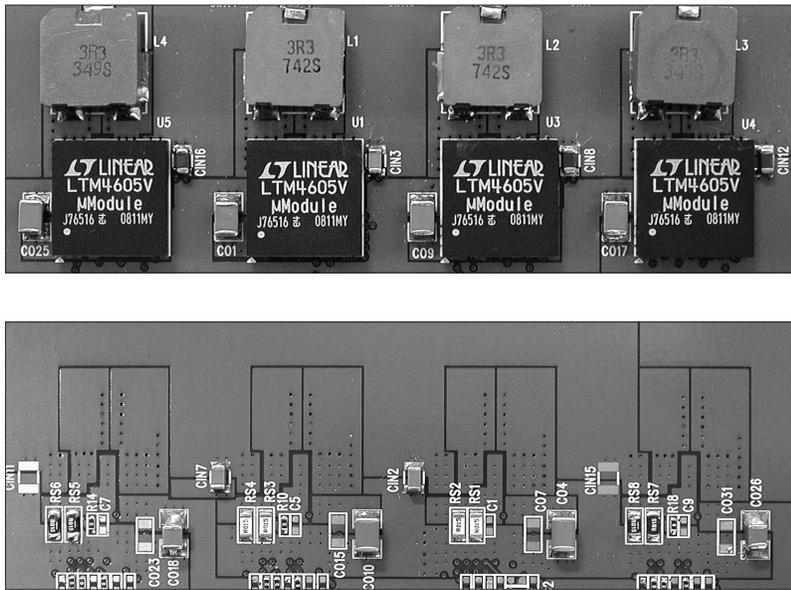
Figure 5. Simple layout of four LTM4605 μModule regulators in parallel: top and bottom sides of the board (additional input and output bulk caps are placed on the top and bottom).
