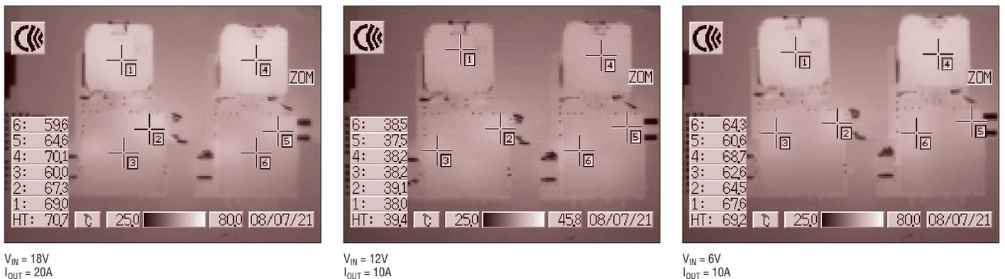
**Figure 4. Thermal stress is evenly distributed between the two LTM4605s and two inductors for the circuit in Figure 1 (shown here with no air flow or heat sink).**
