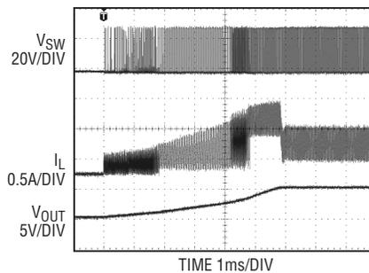
Figure 3. Soft-start waveforms
