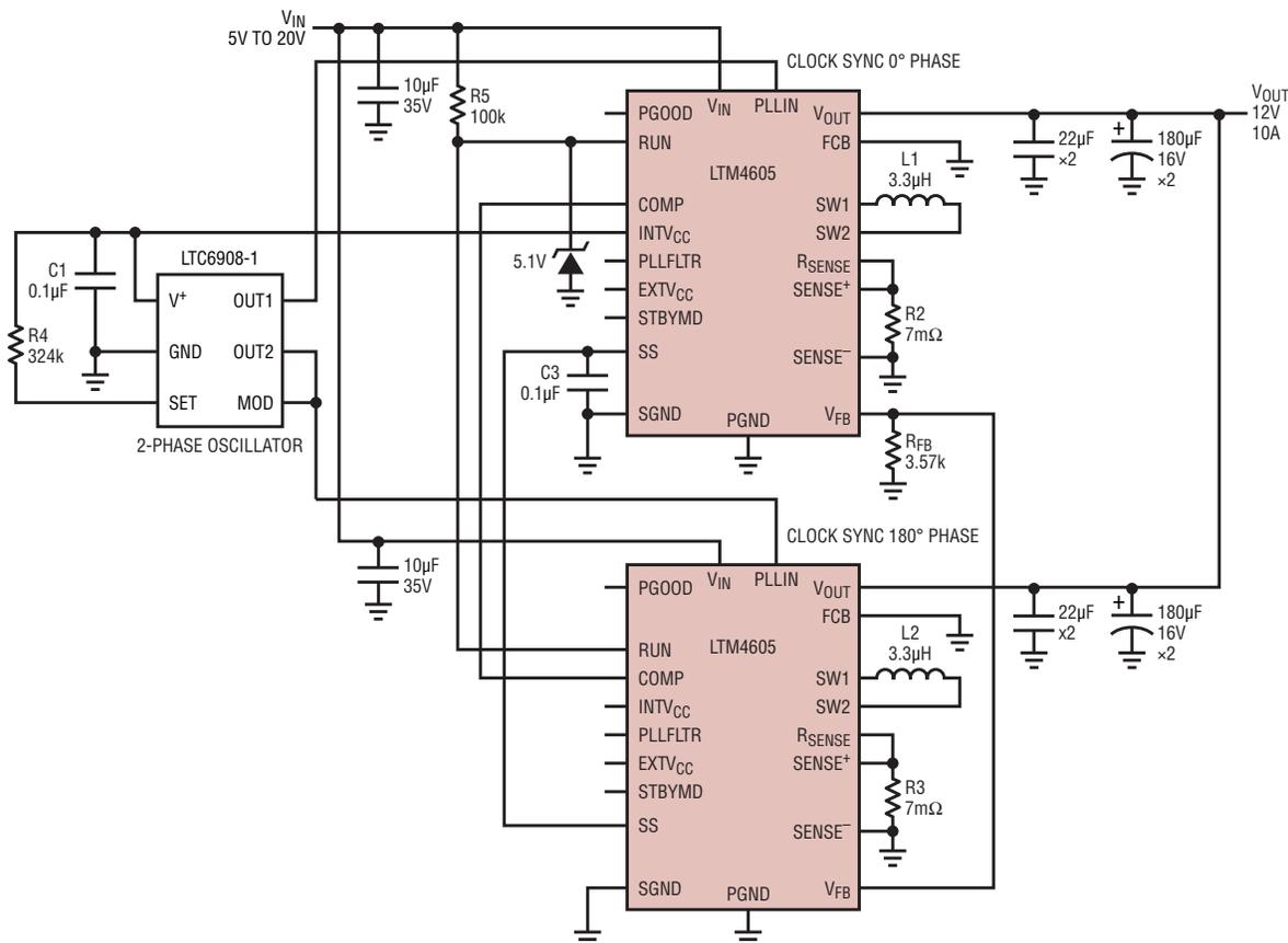
Figure 1. Paralleling two LTM4605s for high output current
