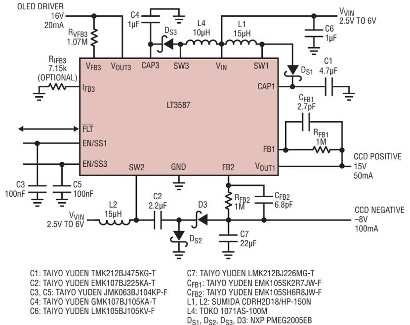
**Figure 14. Li-ion driver for an OLED panel and a CCD imager with a Schottky diode replacing the inverter's output inductor**
