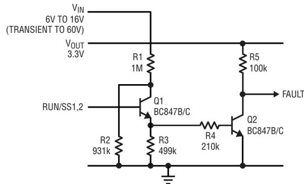
Figure 1. LT3509 RUN/SS to FAULT signal interface
