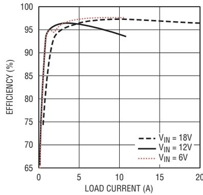
**Figure 2. High efficiency from the parallel LTM4605s in Figure 1 (CCM mode)**
