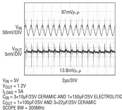
**Figure 7. Input and output noise of comparable  $\mu$ Module regulator without low noise feature**
