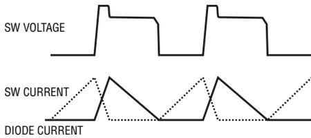
**Figure 2. LT3573 flyback converter in boundary mode.**
