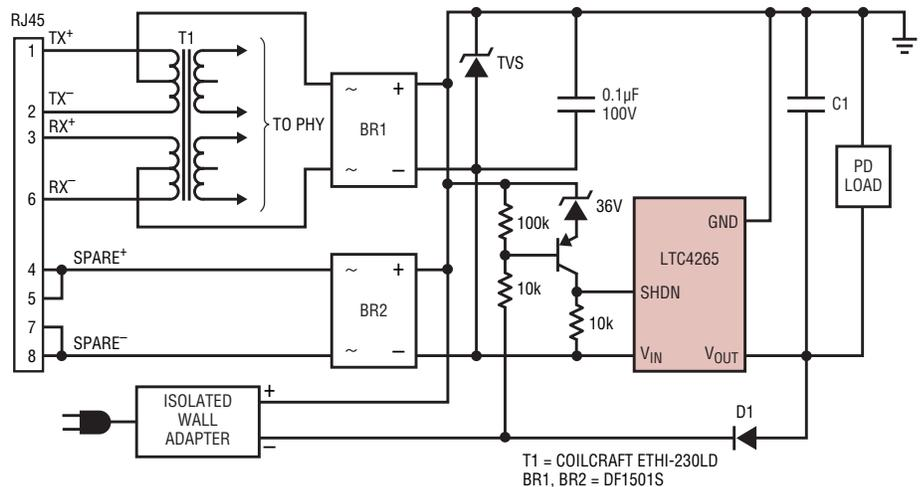
Figure 4. Auxiliary power supply. Auxiliary power takes precedence over PoE power (using the SHDN pin).
