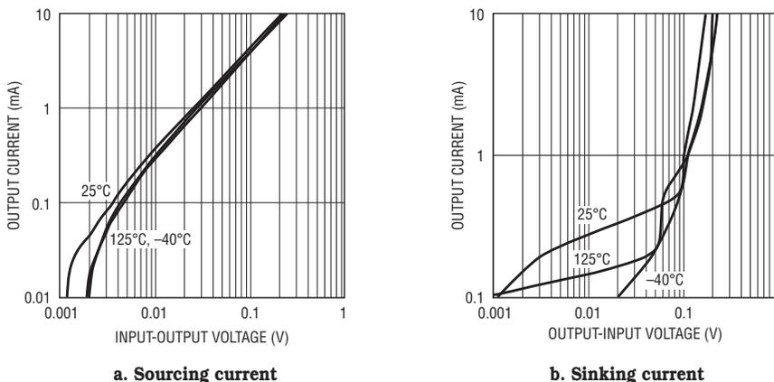
Figure 7. Dropout voltage sourcing and sinking current
