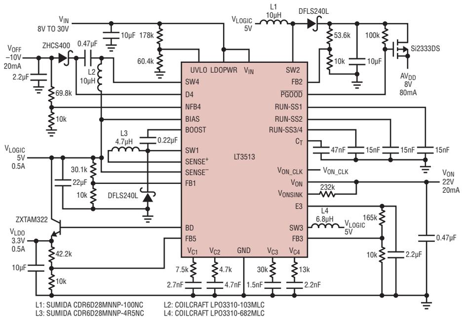
Figure 1. A complete 5-output 2MHz TFT-LCD power supply
