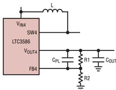
**Figure 5. Boost converter application circuit**
