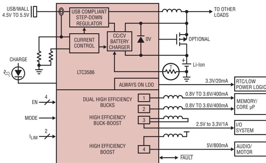
**Figure 4. The LTC3586 is a high efficiency PowerPath controller, always-on LDO, dual buck, buck-boost, plus boost—all in a 4mm x 6mm package**
