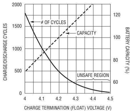
**Figure 2. Charger float voltage vs battery capacity and cycle life**
