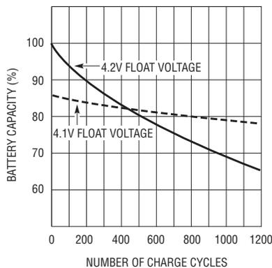
**Figure 3. Cycle life and capacity vs 4.1V and 4.2V float voltages**
