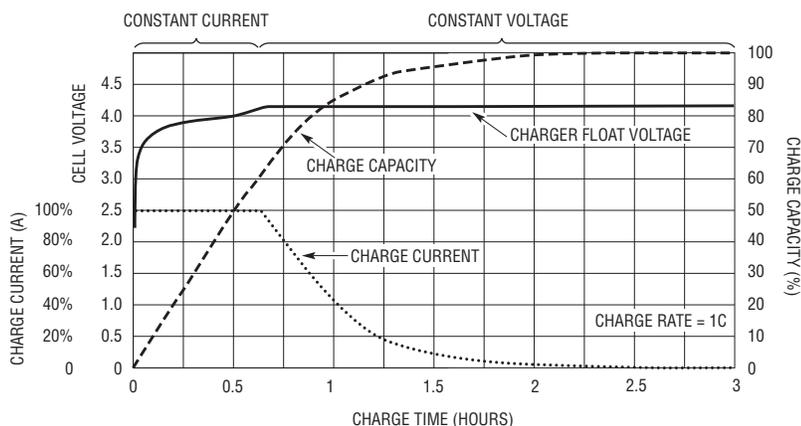
Figure 1. Typical charge profile showing charge current, voltage and capacity
