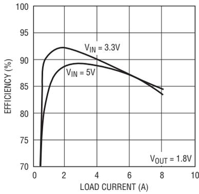
**Figure 4. High efficiency is achieved with the LTM4608 in the application of Figure 3.**
