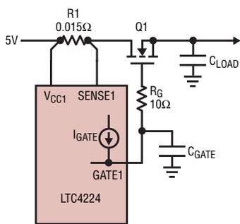
**Figure 3. A method to adjust inrush current by gate capacitor.  $R_G$  prevents parasitic self-oscillation in Q1**
