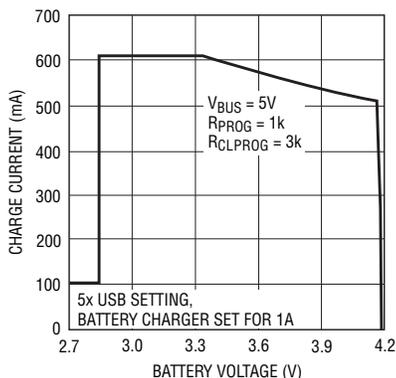
**Figure 1. Battery charge current vs battery voltage**
