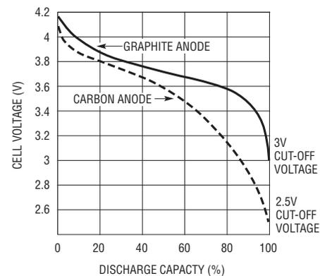
**Figure 4. Li-ion discharge voltage profile for different anode materials**
