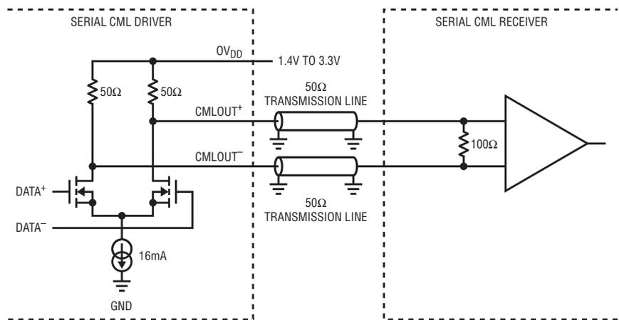
**b. CML termination, directly-coupled differential mode**
