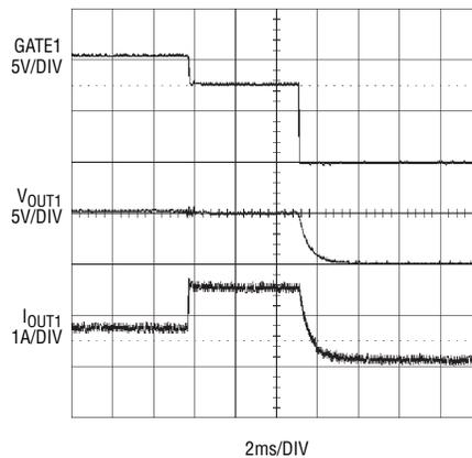
**Figure 4. Active current limiting latches off the external MOSFET following a mild overcurrent**
