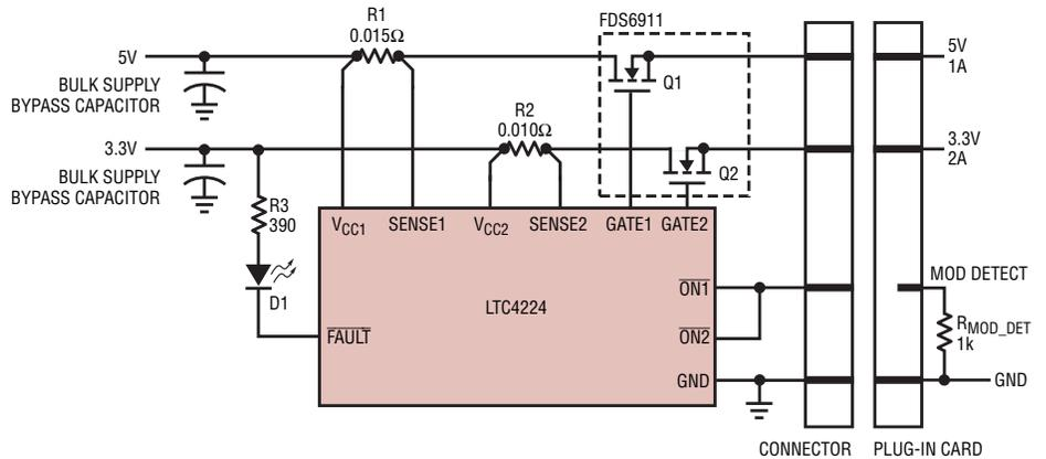
Figure 6. XENPAK/X2 optical module Hot Swap application
