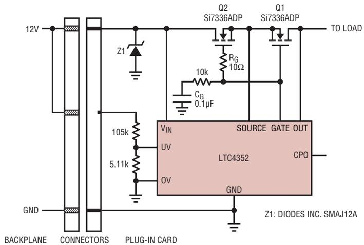
a. Omitting the CPO capacitor and adding an RC network on the gate allows inrush current control on a Hot Swap board.
