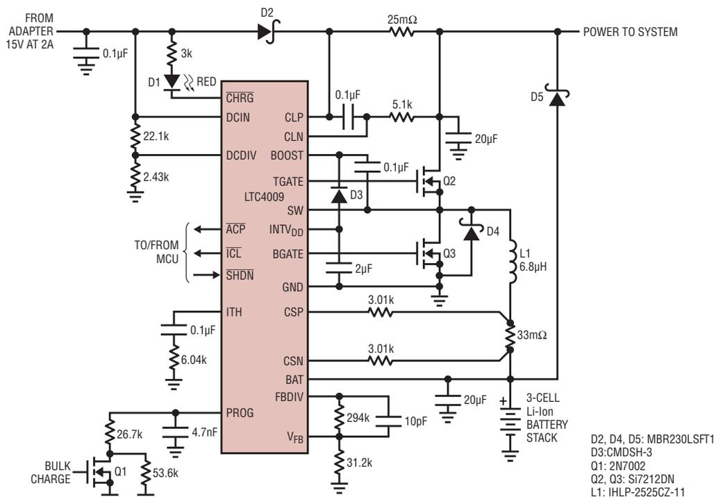
Figure 1. A 12.6V, 3A lithium-ion charger
