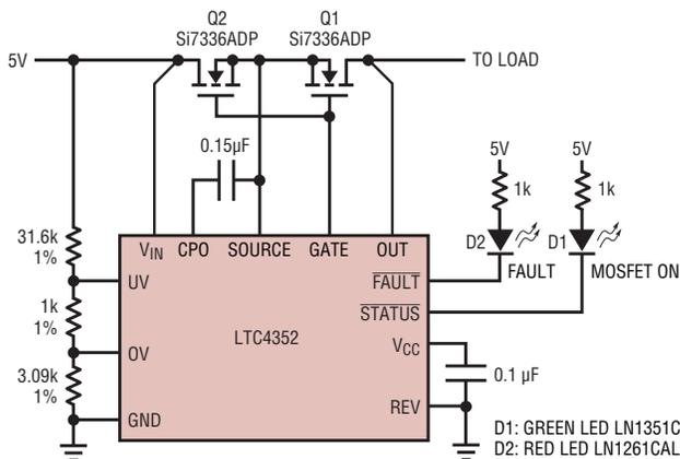
**Figure 6. A 5V ideal diode circuit with input undervoltage and overvoltage protection. Ideal diode function operates for  $4.36V < V_{IN} < 5.78V$ , else GATE is low.**
