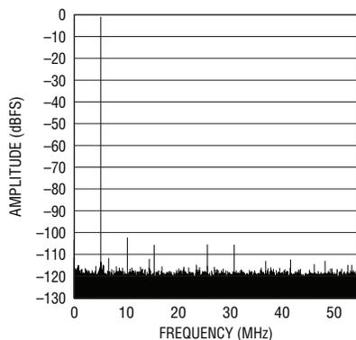
Figure 1. Typical LTC2274 performance at 105MSPS  $f_N = 4.93\text{MHz}$
