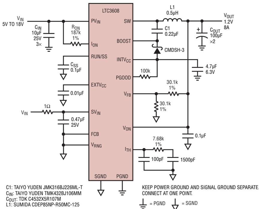
Figure 1. Typical application of the LTC3608
