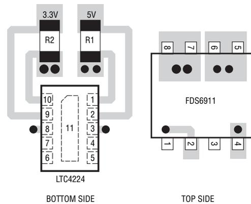
Figure 7. A compact PCB layout of the sense resistors, MOSFET and the LTC4224
