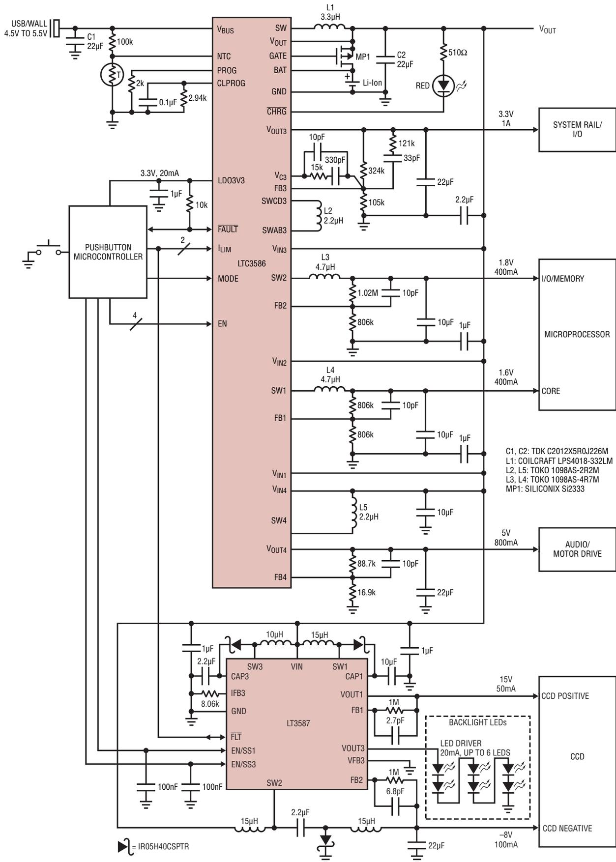
Figure 2. Complete power solution for portable cameras
