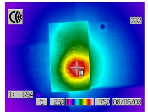
**Figure 7. Good thermal balance is maintained between two paralleled LTM4608 boards supplying 16A output current.**
