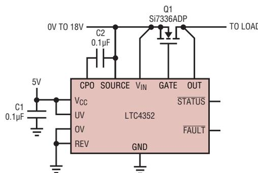
Figure 8. A 0V to 18V ideal diode circuit. By powering the V<sub>CC</sub> pin with an external supply in the 4.7V to 6V range (here 5V), V<sub>IN</sub> can operate down to 0V and up to 18V.
