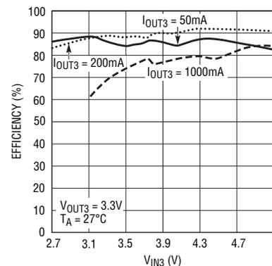
charger under worst case conditions. The LTC35xx switching power managers can charge at up to 1.2A max and provide seamless switchover to battery power when the external power is removed. In USB applications, the constant power (vs constant current) nature of the switching PowerPath controller makes it possible to charge with *more than* 500mA from a fixed 500mA USB input source, as shown in Figure 2.
