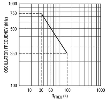
Figure 1. Relationship between oscillator frequency and resistor connected between FREQ/PLLFLTR and GND
