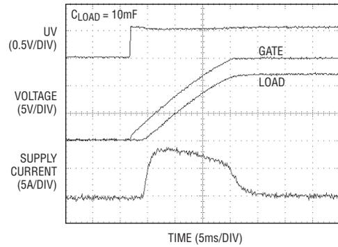
b. After short pin makes contact and UV is above 0.5V, GATE starts ramping up. Once it crosses the MOSFET threshold voltage, LOAD follows with the same dV/dt. Here, inrush is limited to 8.3A peak for a 10mF C<sub>LOAD</sub>.
