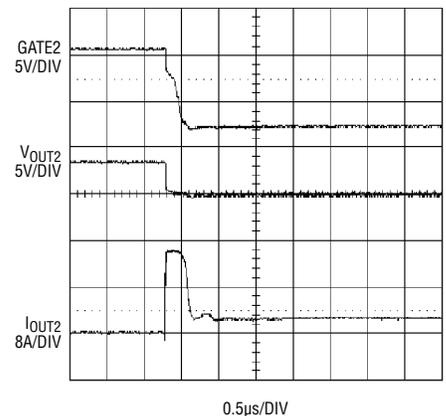
**Figure 5. Fast current limit isolates severe short circuit fault in less than 0.5µs**
