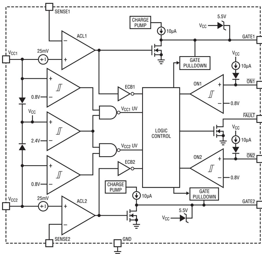
Figure 1. Functional block diagram of the LTC4224
