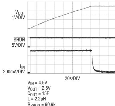
**Figure 4.** Waveforms of input current and  $V_{OUT}$ , charging large  $C_{OUT}$  from 0 volts
