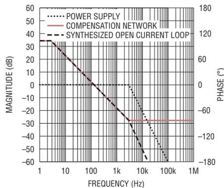
Figure 4. Current loop synthesis with 0,-1,-2 shape
