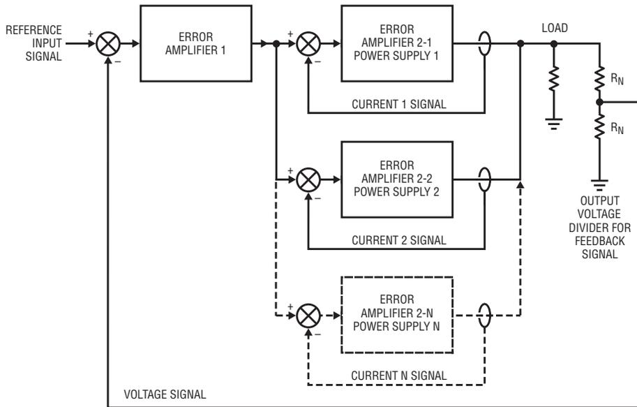
Figure 2. Power system control loop
