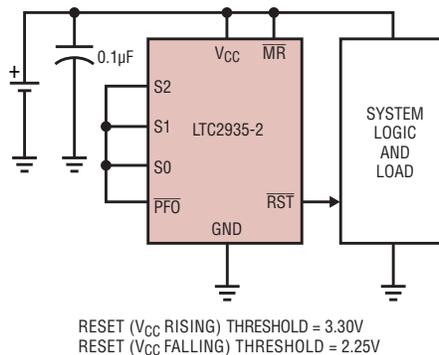
Figure 5. Active threshold control
