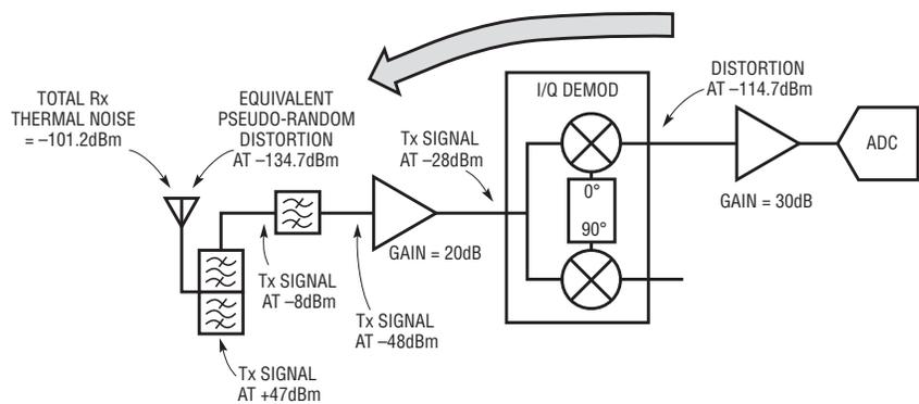
Figure 4. Transmitter leakage effects
