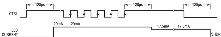
Figure 2. Current programming and shutdown timing
