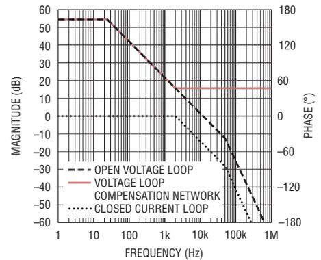
Figure 9. Voltage loop Bode design with closed current loop having 0,-1,-2 shape
