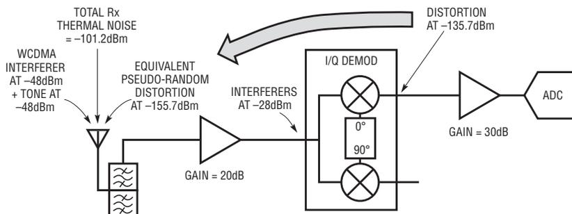
Figure 6. 3rd Order distortion due to WCDMA carrier + tone interferer
