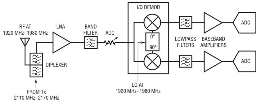
Figure 1. Direct conversion receiver architecture
