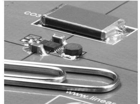
**Figure 1. A complete PCMCIA-powered, low profile solution for GSM transmitters**
