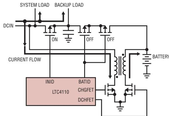
Figure 3. The LTC4110 in charge mode
