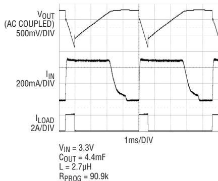
**Figure 3.** Waveforms of input current and  $V_{OUT}$  for a pulsed load current
