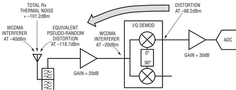
Figure 3. 2nd Order distortion due to WCDMA carrier
