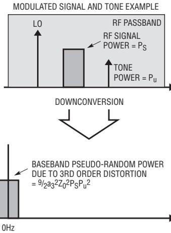
Figure 5. Effects of 3rd order distortion
