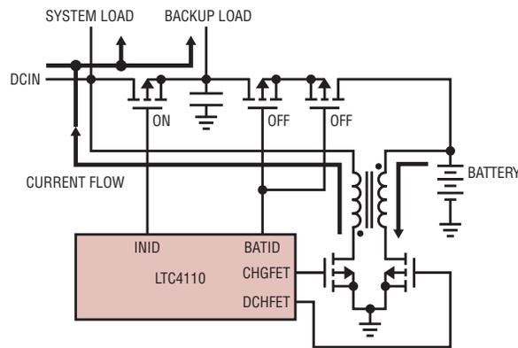
Figure 4. LTC4110 in calibration mode
