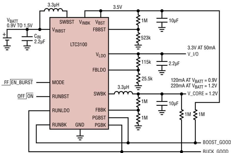
Figure 3. Single-cell dual output converter with voltage sequencing
