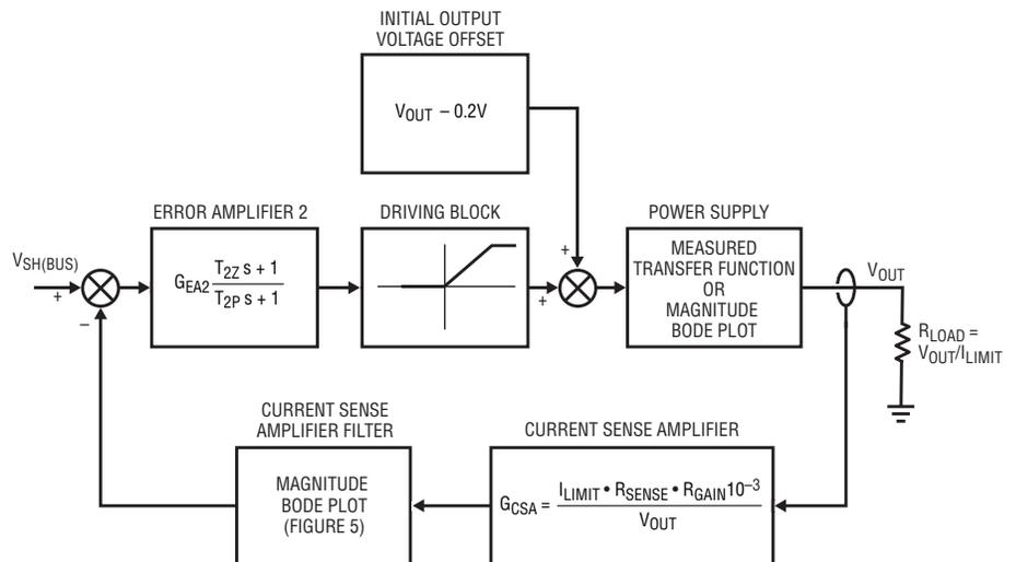
**Figure 6. Current loop control block diagram**
