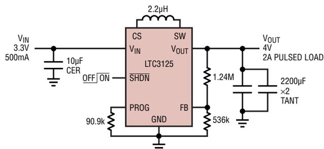
**Figure 2. PC Card or CompactFlash (3.3V/500mA max) 4.0V output, GSM pulsed load**
