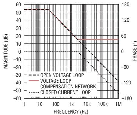
Figure 8. Voltage loop Bode design with current closed loop having 0,-1 shape
