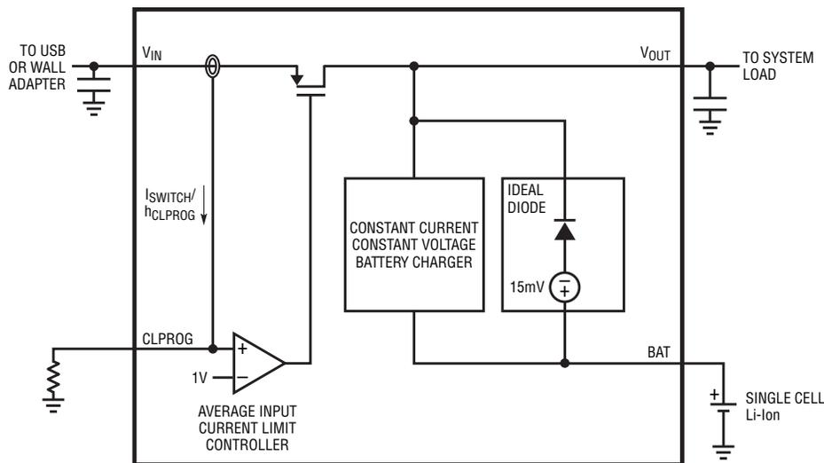
Figure 2. Block diagram of a traditional linear PowerPath, which has significant inherent efficiency limitations.
