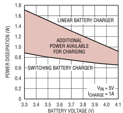
**Figure 1. Reduce battery charge time and keep handheld devices cool by using a switching PowerPath manager/battery charger.**
