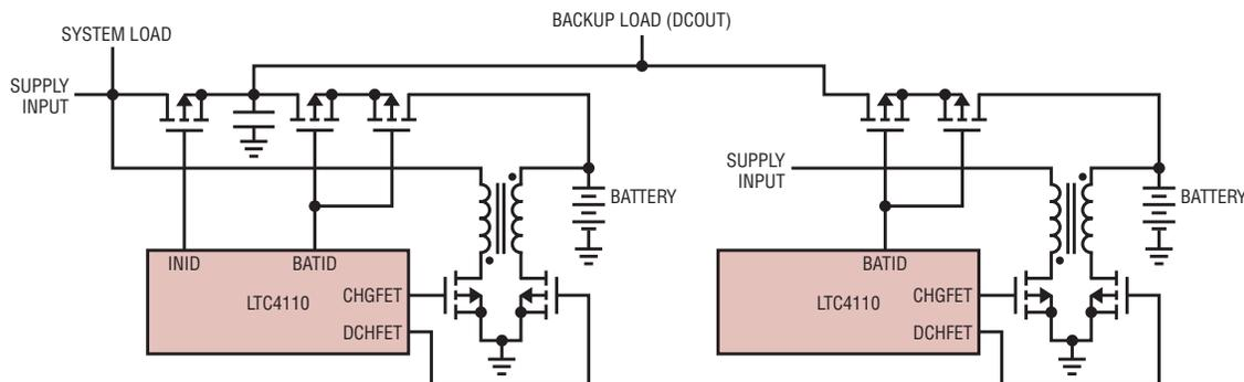
Figure 6. Dual LTC4110 system using standard batteries
