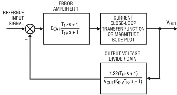
Figure 7. Voltage loop control block diagram
