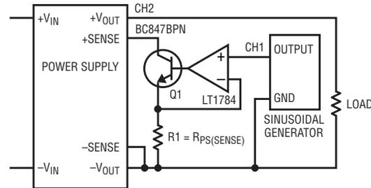
Figure 1. Power supply closed-loop Bode plot measurement block diagram
