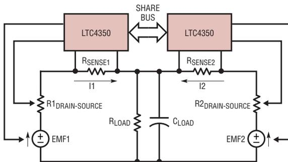
Figure 10. Output power stage equivalent circuitry. The power supply output characteristic exists in the second quadrant
