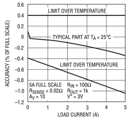
**Figure 3. Measurement accuracy vs load current for the LT6106 and LT6107**
