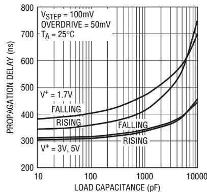
**Figure 1. Speed is maintained with high capacitive loads**
