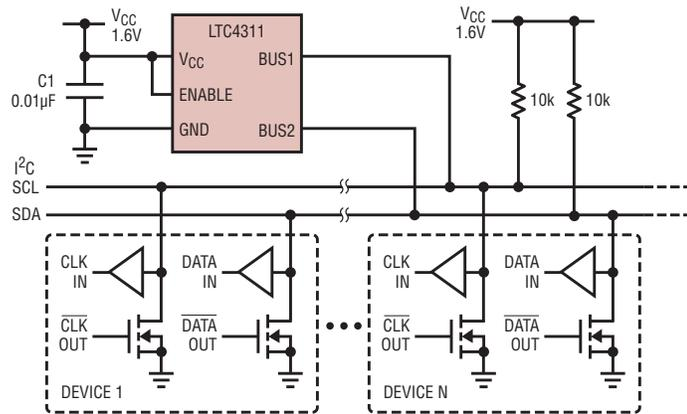
Figure 1. Typical LTC4311 low voltage application circuit
