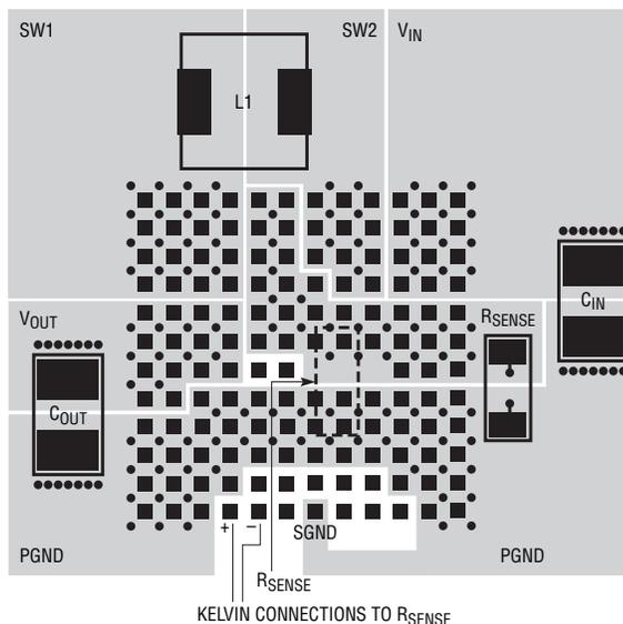
Figure 11. Kelvin connection used to sense current.
