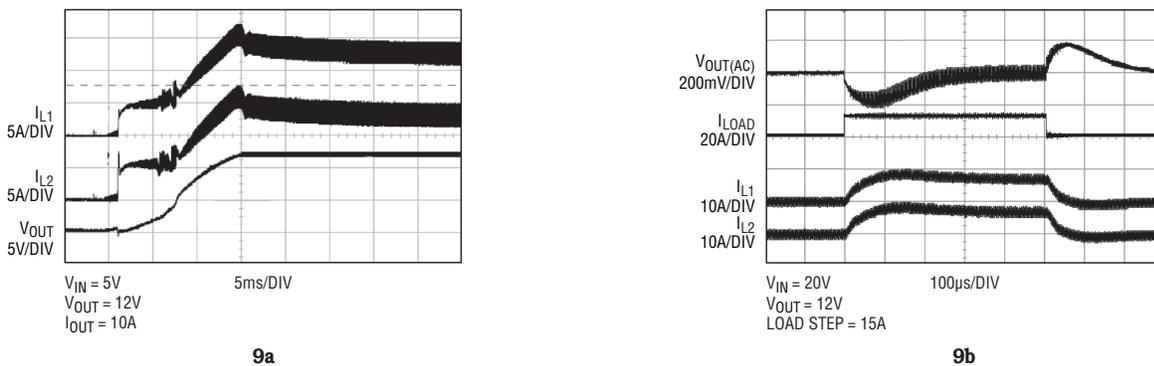
Figure 9. Inductor current waveforms at start-up and load transient with two LTM4607s in parallel
