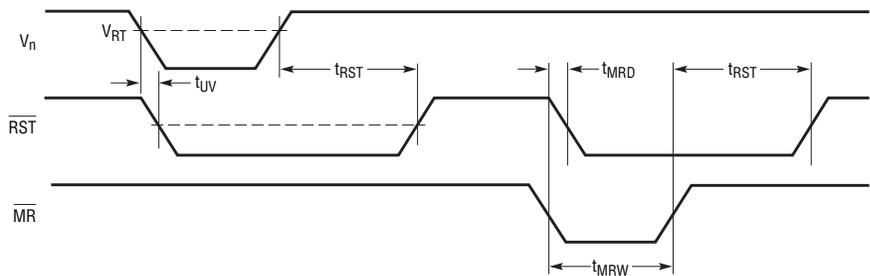
Figure 8.  $\overline{MR}$  timing diagram
