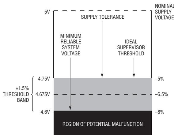
Figure 3. Tight 1.5% threshold accuracy yields high system reliability
