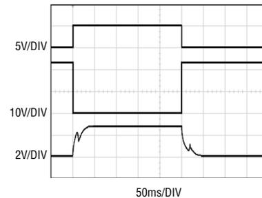
**Figure 7.** Waveforms for solenoid driver. Top trace is the MOSFET gate, with high on. Middle trace is the bottom of the solenoid/inductor. Bottom trace is the LT6105 output, representing solenoid current at 80mA/DIV. Glitches are useful indicators of solenoid plunger movement.
