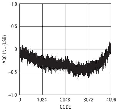
**Figure 2. Typical INL error of ADIN voltage is within  $\pm 0.5$ LSB.**
