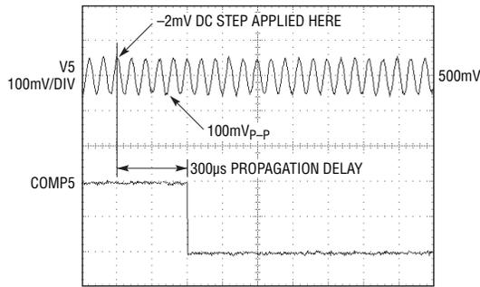
**Figure 4. Comparator output is resistant to noisy input voltage**
