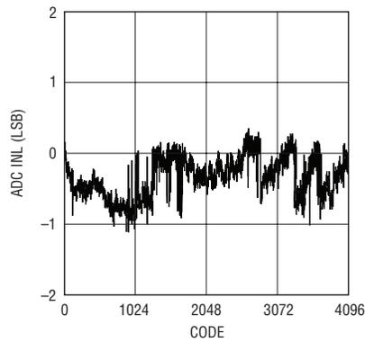
**Figure 3. Typical INL error of current sense voltage is within  $\pm 1$ LSB.**
