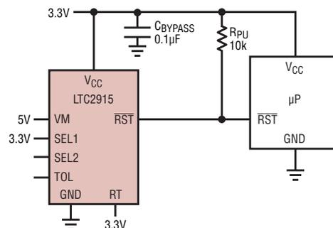
Figure 2. A 5V, -10% tolerance supply monitor with 200ms internal reset timeout
