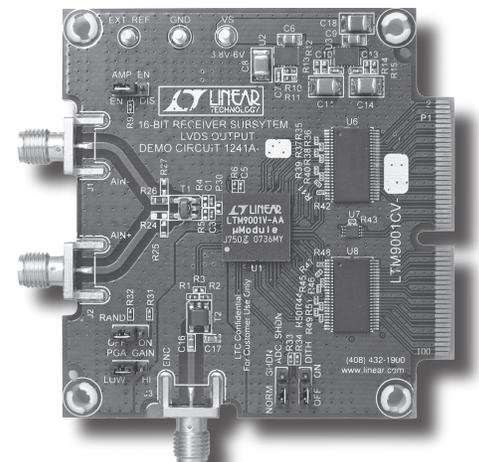
**Figure 4. An evaluation board shows the small overall circuit. Note that no external components are required.**
