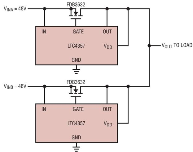
Figure 1. Two load-sharing, redundant, 48V/10A power supplies using an ideal diode
