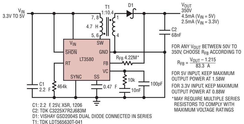
Figure 6. This 350V power supply features a tiny 5.8mm × 5.8mm × 3mm transformer switching at 200kHz.
