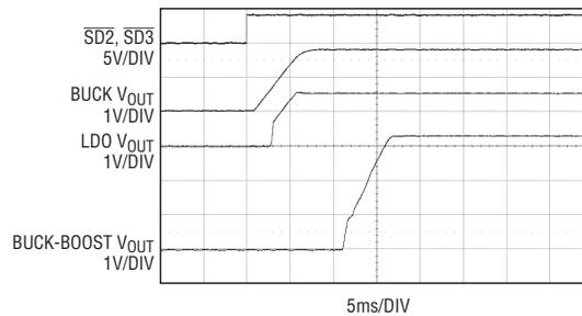
Figure 3. Output voltages during sequenced start-up
