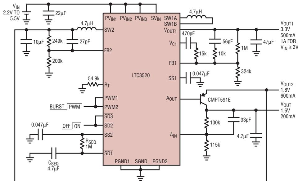
**Figure 2. Sequenced start-up, triple-output converter**
