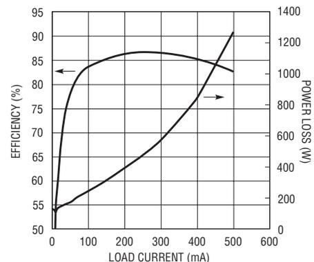
Figure 3. The high 2.5MHz switching frequency of this 5V to 12V boost converter allows the use of a tiny 4mm x 4mm x 1.7mm inductor.
