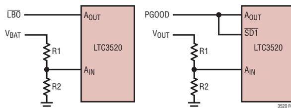
Figure 4. Implementation of low battery and power-good indicators
