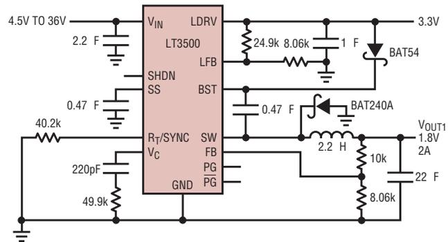
**Figure 5. 1.8V/2A step-down regulator**
