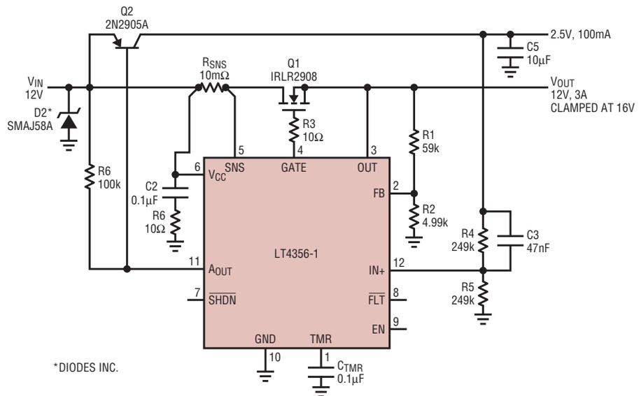
Figure 6. The LT4356's internal spare amplifier can drive an external PNP to provide another supply rail.
