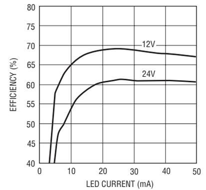
the 24V input supplies respectively. In comparison, the resistor-biasing approach would yield dismal 25% and 12.5% efficiencies.
