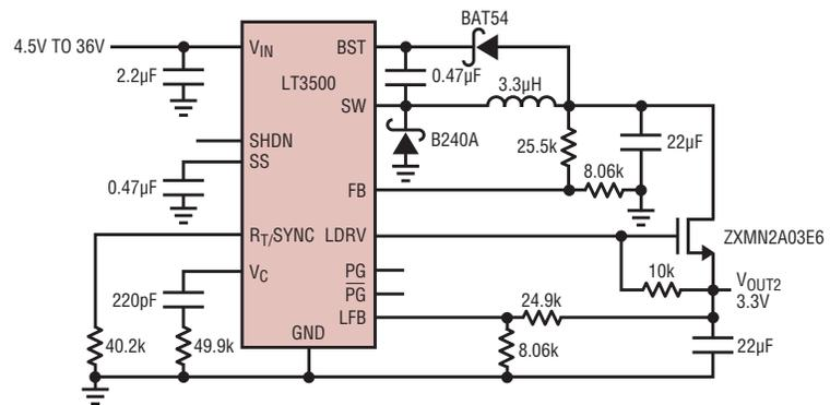
**Figure 6. High efficiency linear regulator**
