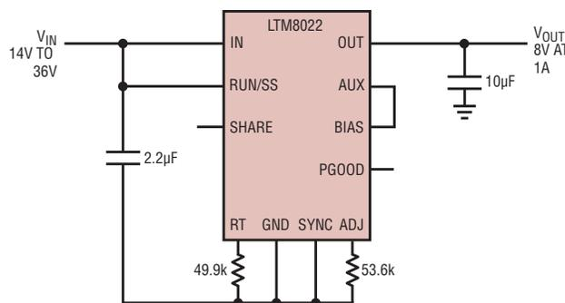
Figure 4. The LTM8022 can produce 8V, too
