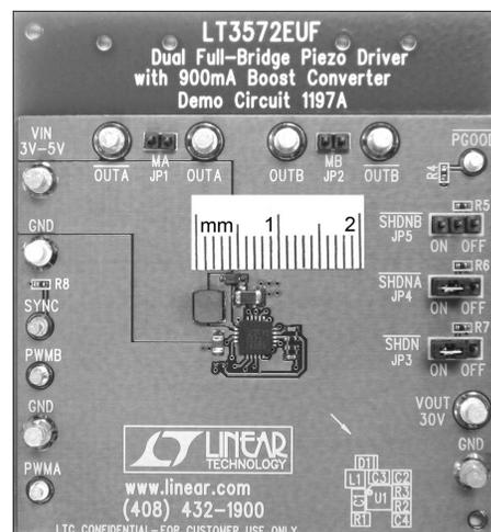
Figure 2. Typical layout for the Figure 1 converter
