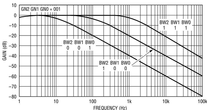
**Figure 8. Measured frequency responses for Figure 7**
