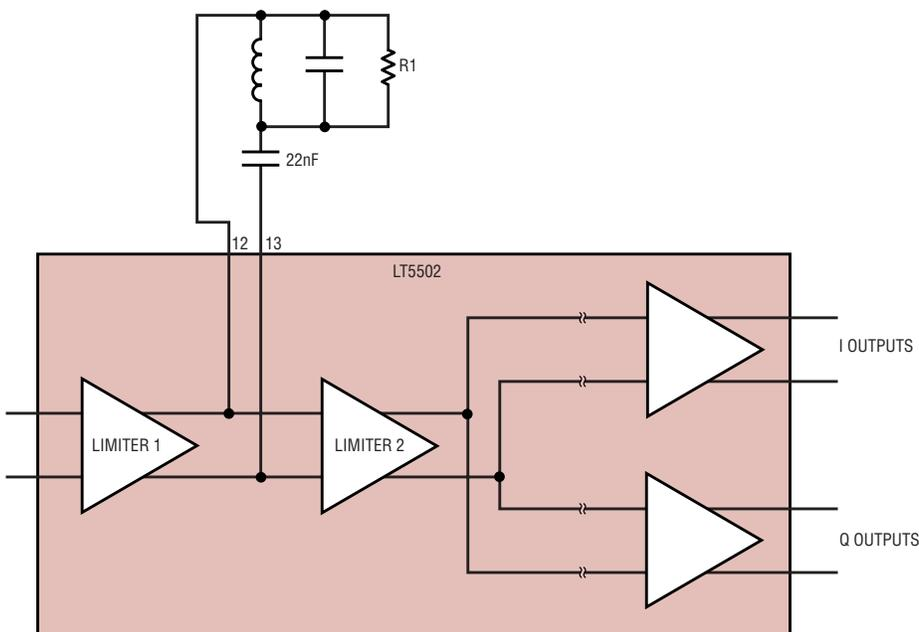
Figure 5. Example of an LT5502 interstage filter
