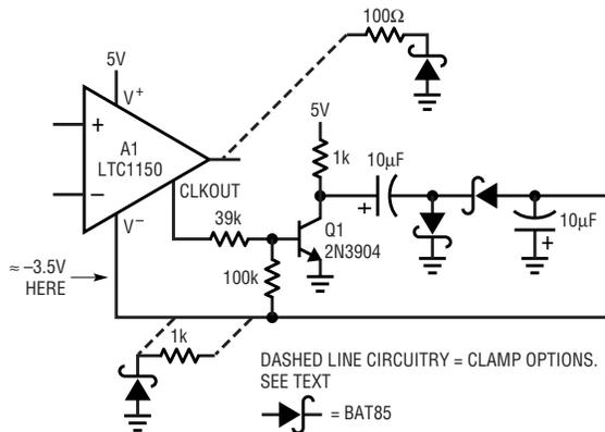
**Figure 1. Single rail powered amplifier has true zero volt output swing. A1's clock output switches Q1, driving diode-capacitor charge pump. A1's  $V^-$  pin assumes negative voltage, permitting zero (and below) volt output swing.**
