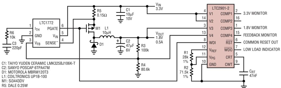
**Figure 8.** Use the LTC2901-2 to monitor the input, output, feedback voltage and low load conditions on a DC/DC controller. In this case, the controller is an LT1772 used in a 3.3V input to 1.8V output application.
