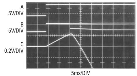
**Figure 2. Amplifier bootstrapped supply start-up. Amplifier  $V^-$  pin (trace C) initially rises positive at 5V supply (trace A) turn-on. When amplifier internal clock starts (trace B, 5th vertical division), charge pump activates, pulling  $V^-$  pin negative.**
