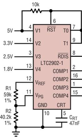
**Figure 9. Quad supply monitor with asymmetric hysteresis**
