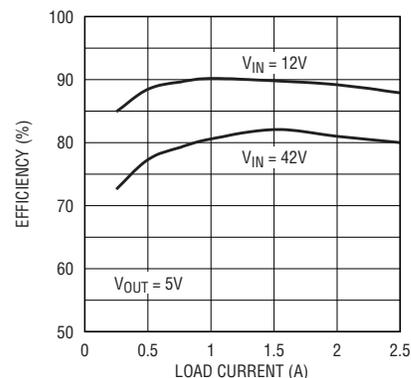
**Figure 3. Efficiency of the circuit shown in Figure 2**
