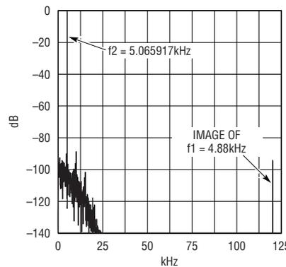
**Figure 4. Secondary channel translated from 120kHz to 5kHz**
