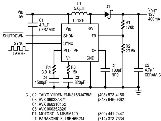
Figure 1. 5V to 12V converter synchronized at 1.6MHz
