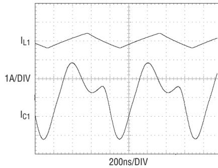
**Figure 2b. In the circuit shown in Figure 1b, the output capacitor (C1) peak-to-peak current ripple is five times as high as inductor peak-to-peak ripple (and therefore five times as high as the current ripple shown in Figure 2a) with 1A output.**
