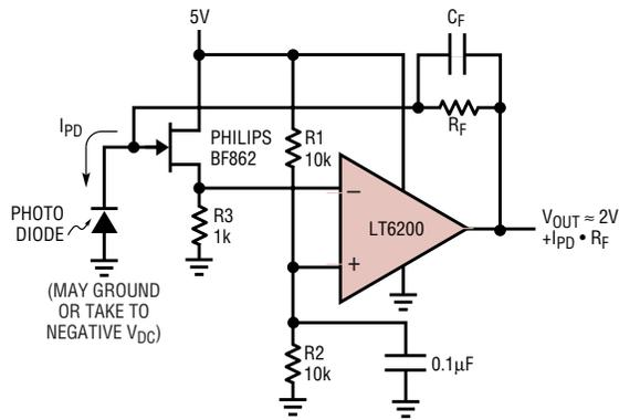
Figure 7. Single supply,  $1.5\text{nV}/\sqrt{\text{Hz}}$ , photodiode amplifier
