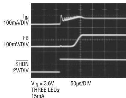
**Figure 4. Soft-start waveforms**
