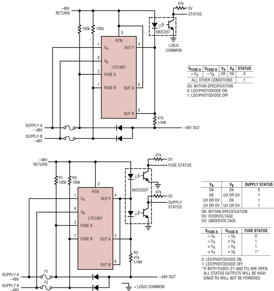
Figure 3: Output OR allows for fewer components
