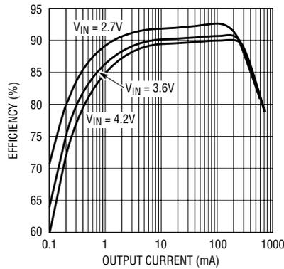
**Figure 4. Efficiency vs Load Current for LTC3406-1.8**
