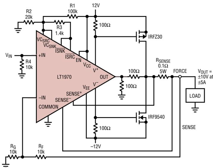
**Figure 4. Boosting the output current capability to ±5A**
