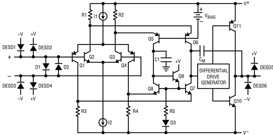
Figure 3. LT6200-4 simplified schematic
