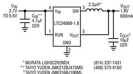
Figure 1. 1.8V/600mA step-down regulator using all ceramic capacitors
