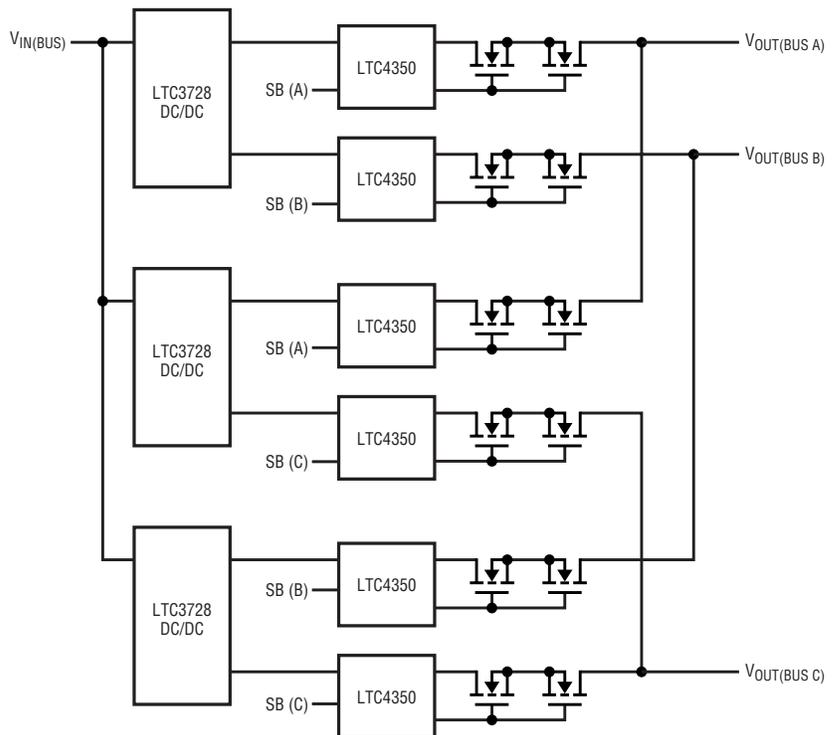
**Figure 6. Block diagram of a redundant multiple voltage output system**
