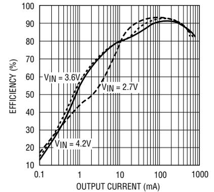
**Figure 5. Efficiency vs Load Current for LTC3406B-1.8**
