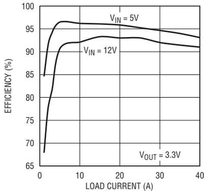
Figure 3. Measured efficiency of the LTC3729 circuit
