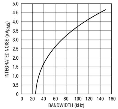
Figure 6. Line receiver integrated noise 25kHz to 150kHz
