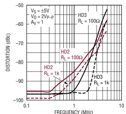
Figure 2. LT6200 distortion vs frequency
