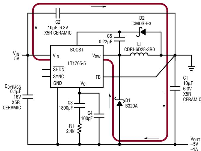
Figure 1b. LT1765 5V to -5V converter with the bulk cap between  $V_{IN}$  and ground has much higher output ripple than the circuit in Figure 1a. The high  $di/dt$  path, indicated here with bold red lines, includes the output capacitor, thus increasing output ripple.
