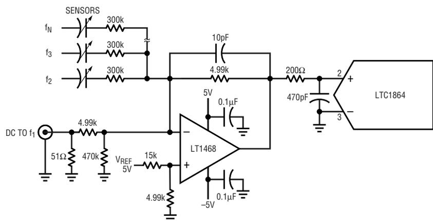
Figure 2. Using a large number of sensors
