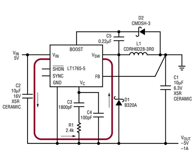
Figure 1a. LT1765 5V to -5V converter with bulk input cap between  $V_{IN}$  and  $V_{OUT}$  (IC GND pin) has low output ripple. The high  $di/dt$  path, indicated here with bold red lines, does not include the output capacitor.
