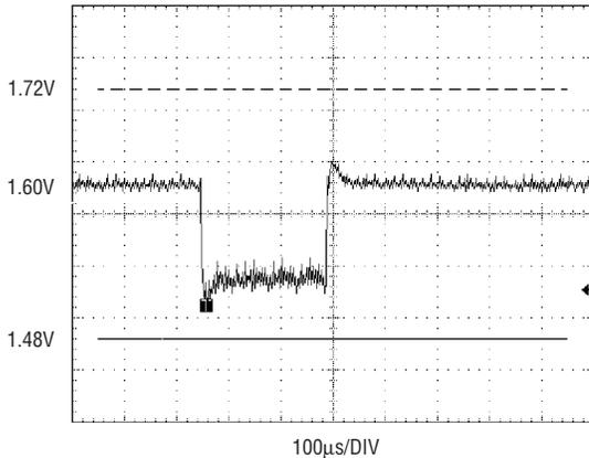
**Figure 2. Transient response for a 12A load-current step**
