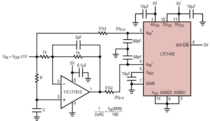
**Figure 8b. True differential inputs accept  $4V_{P-P}$  bipolar differential signal with  $2V_{P-P}$  swings on each input and an effective gain of 2 from the LT1813 inputs. SINAD = 70.7dB with a 1MHz input.**
