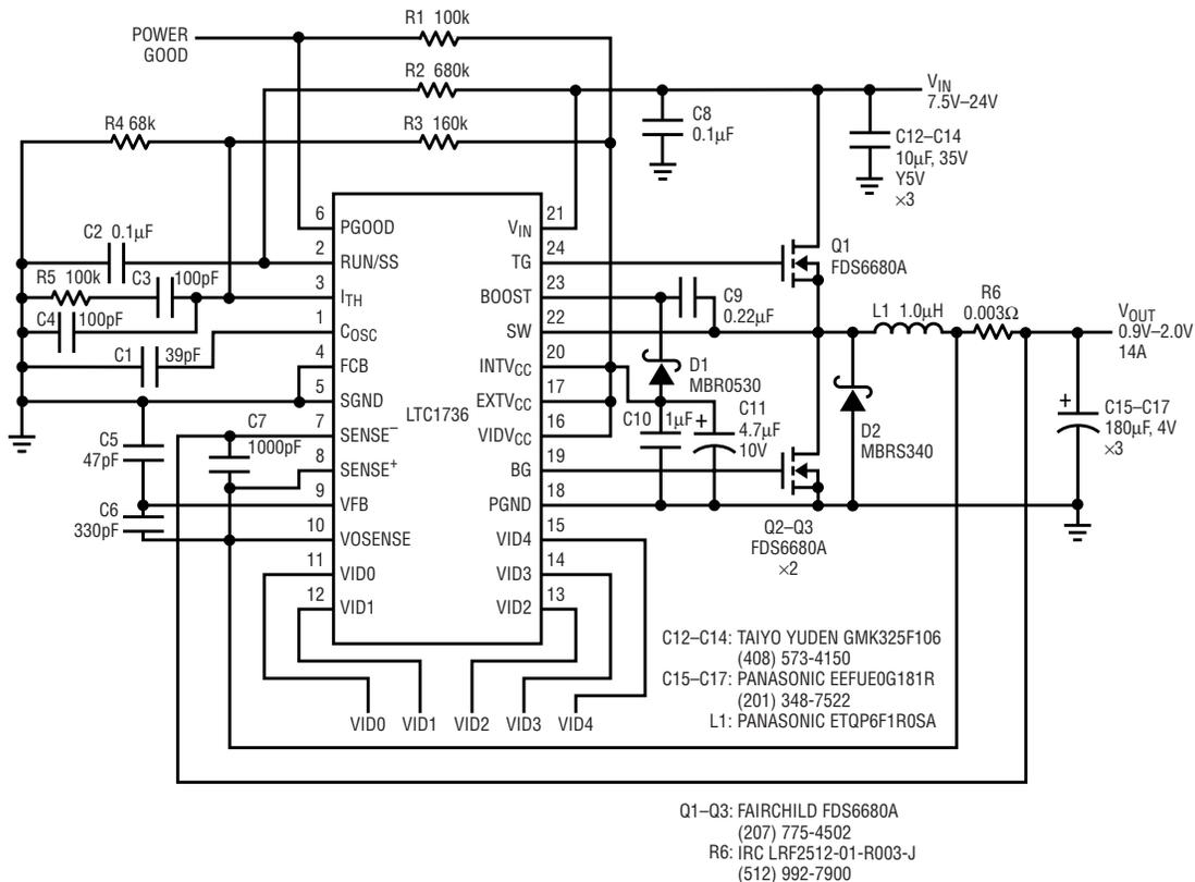
Figure 1. LTC1736-based core-voltage regulator with active voltage positioning
