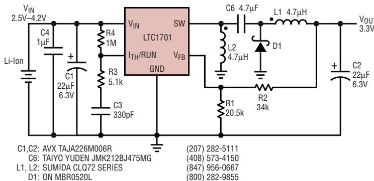
**Figure 7. Single-cell Li-Ion to 3.3V zeta converter**
