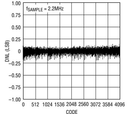
**Figure 6. Differential nonlinearity vs output code (unipolar 0V–4V)**
