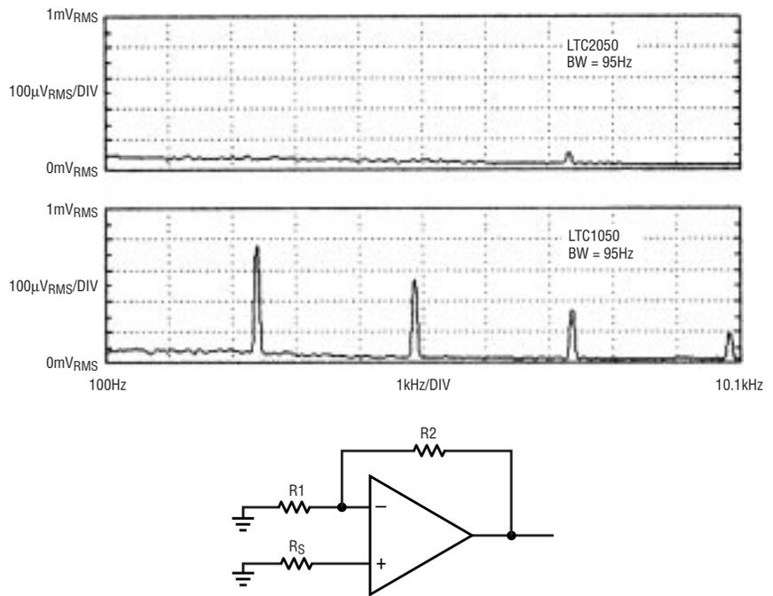
Figure 4. Output spectrum with a gain of  $100$ ;  $R_2 = 100k$ ;  $R_1 = R_S = 1k$
