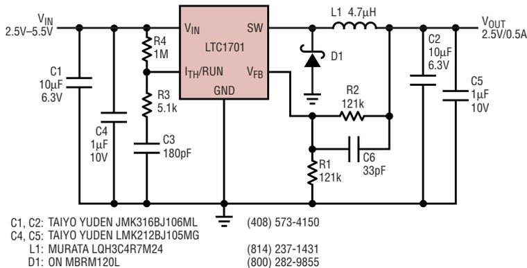
Figure 11. All-ceramic-capacitor converter delivers 2.5V at 500mA.
