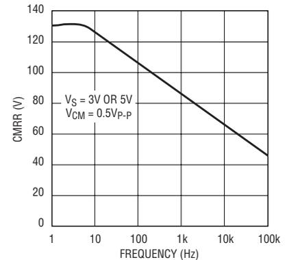
**Figure 2. LTC2050 common mode rejection ratio vs frequency**
