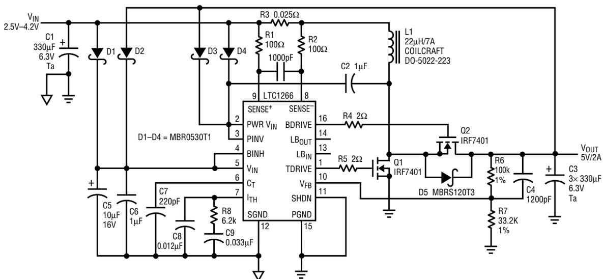
Figure 1. Bootstrapped synchronous boost converter
