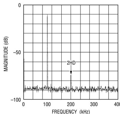
**Figure 3. Harmonic distortion performance of Figure 1's circuit with a 100kHz sine wave at 8.5V<sub>p,p</sub> into 100Ω**
