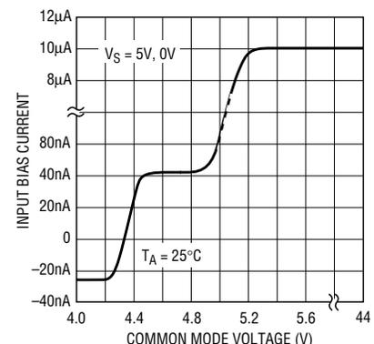
Figure 2. Input bias current vs common mode voltage
