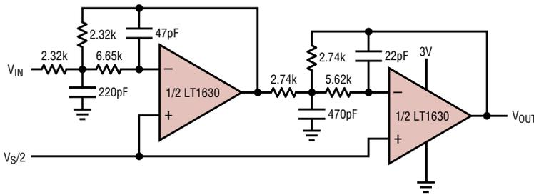
**Figure 5. Single-supply, 400kHz, 4th order Butterworth filter**
