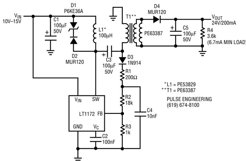
Figure 1. 24V/200mA bulk supply with 3750V<sub>RMS</sub> isolation
