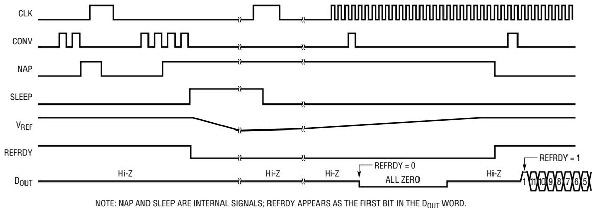
**Figure 3. NAP and SLEEP mode waveforms**
