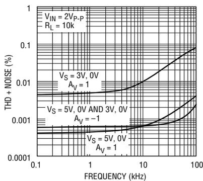
**Figure 1. LT1630 total harmonic distortion + noise vs frequency**
