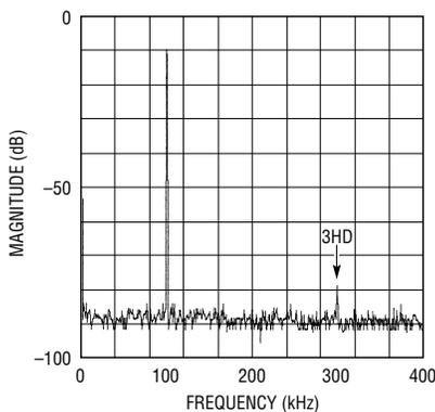
**Figure 2. Harmonic distortion performance of Figure 1's circuit with a 100kHz sine wave at 15V<sub>p,p</sub> into 100Ω**
