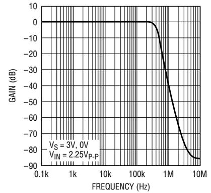
**Figure 6. Frequency response of filter in Figure 5**
