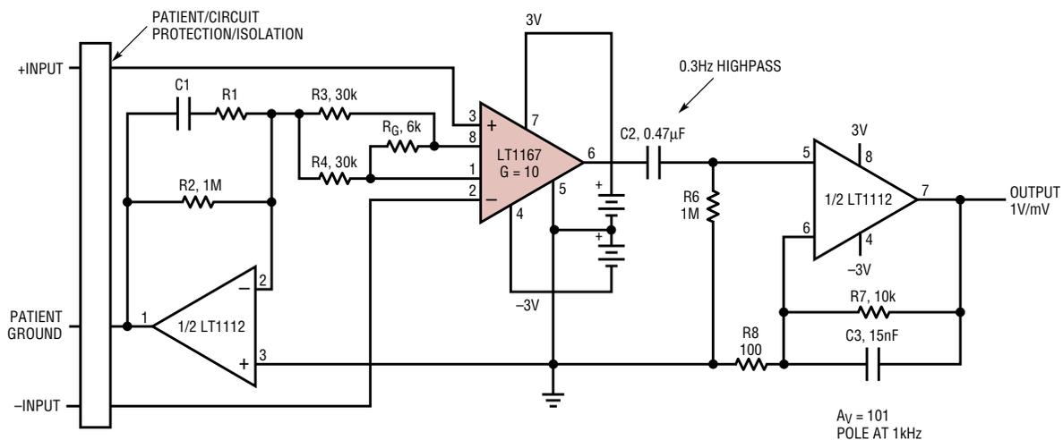
Figure 8. Medical ECG monitor
