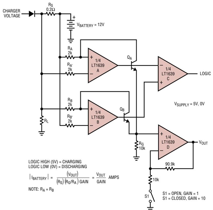
Figure 3. LT1638 battery current monitor—an Over-The-Top application
