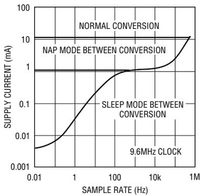
**Figure 4. LTC1404 power consumption in various operating modes**
