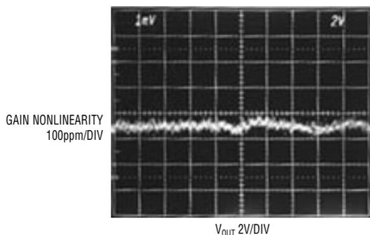
Figure 2. LT1167 gain nonlinearity: R<sub>C</sub> = 1k; V<sub>O</sub> = ±10V
