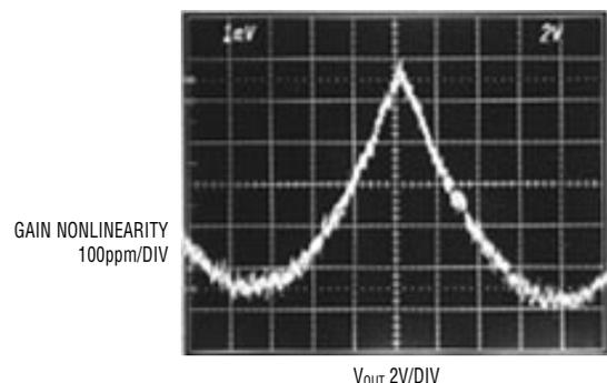
Figure 3. Gain nonlinearity of a previous generation instrumentation amp: R<sub>C</sub> = 1k; V<sub>O</sub> = ±10V
