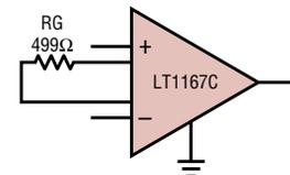
LT1167 MONOLITHIC INSTRUMENTATION AMPLIFIER, G = 100
