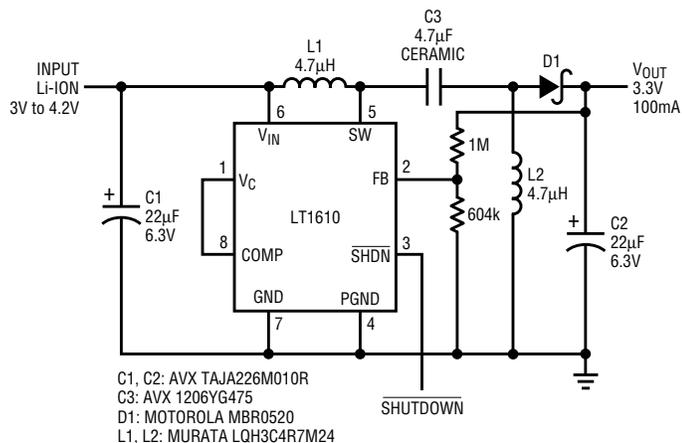
Figure 6. Li-Ion to 3.3V SEPIC converter delivers 100mA.
