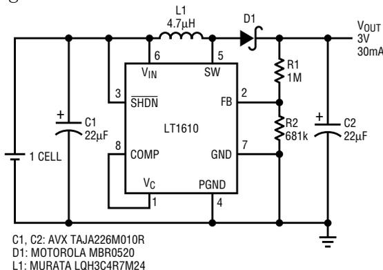
Figure 1. Single cell to 3V converter delivers 30mA.
