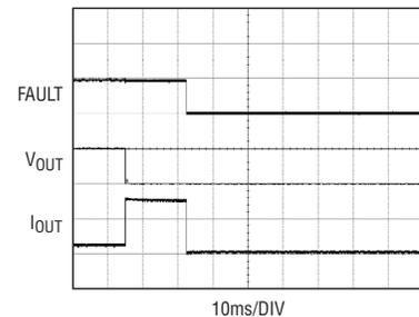
**4b. RST low: converter remains shut down until power is cycled.**
