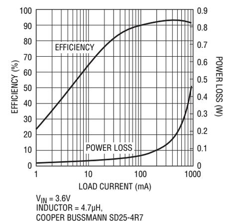
**Figure 3. Efficiency for the circuit in Figure 2**
