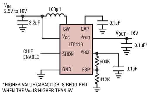
Figure 1. 2.5V-16V To 16V boost converter
