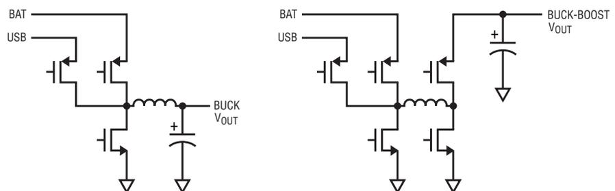
Figure 4. The low loss PowerPath architecture
