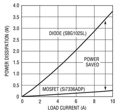
Figure 2. As load current increases, so do the power savings gained from using an ideal diode (LTC4352 + Si7336ADP) instead of a power Schottky diode (SBG1025L).
