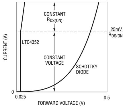
Figure 4. The forward I-V characteristic of the LTC4352 ideal diode vs a Schottky diode.
