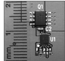
Figure 1. The LTC4352 controlling an N-Channel MOSFET replaces a power diode and associated heat sink to save power, PCB area, and voltage drop. Also shown: the small PCB footprint of the ideal diode circuit using a 3mm x 3mm DFN-12 packaged LTC4352 and SO-8 size MOSFET.
