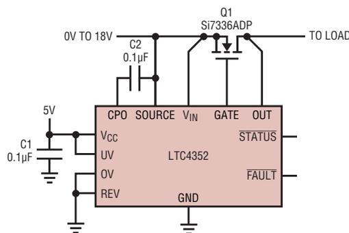
Figure 8. A 0V to 18V ideal diode circuit. By powering the  $V_{CC}$  pin with an external supply in the 4.7V to 6V range (here 5V),  $V_{IN}$  can operate down to 0V and up to 18V.
