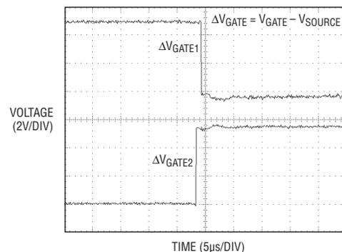
b. Supply switchover from  $V_{IN1}$  to  $V_{IN2}$  due to short-circuit on  $V_{IN1}$  shows minimal disturbance on load voltage.
