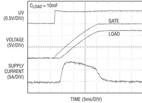
b. After short pin makes contact and UV is above 0.5V, GATE starts ramping up. Once it crosses the MOSFET threshold voltage, LOAD follows with the same  $dV/dt$ . Here, inrush is limited to 8.3A peak for a 10mF  $C_{LOAD}$ .
