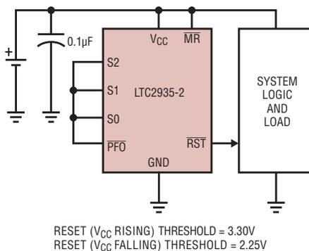
Figure 5. Active threshold control
