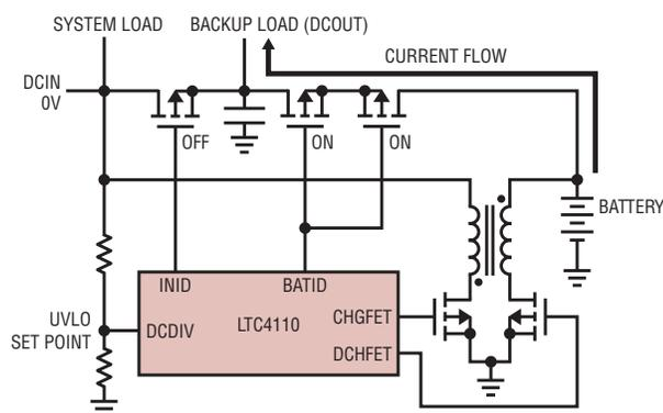
Figure 5. The LTC4110 in battery backup mode
