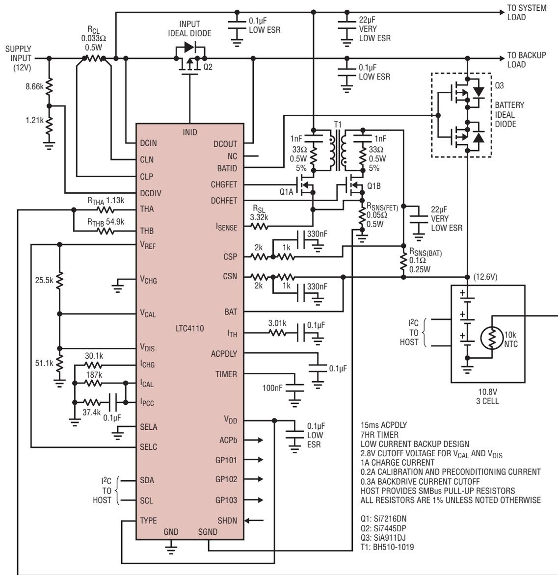
Figure 2. A LTC4110-based battery backup system
