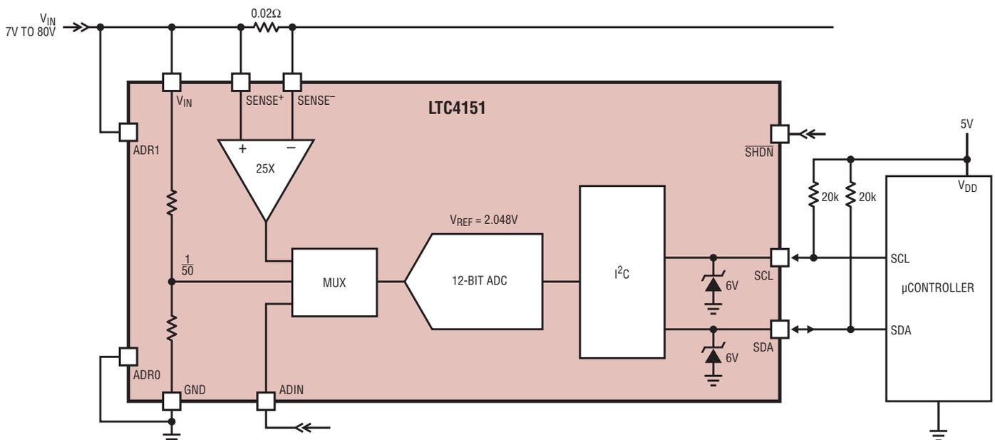
Figure 1. Full featured current and voltage monitor simplifies high voltage, high side sensing.
