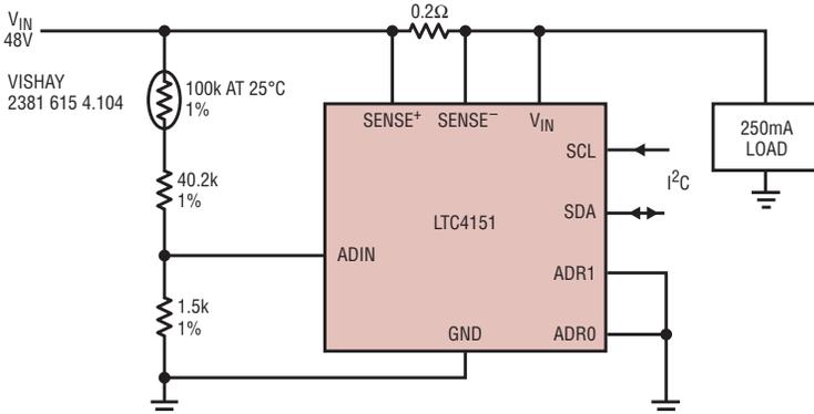
Figure 6. Temperature monitoring is simple with LTC4151 and an NTC thermistor.
