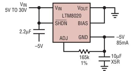
Figure 2. A simple reconfiguration of the µModule generates a negative output
