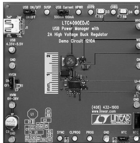
**Figure 2. A complete LTC4090-based USB Power Manager with a 2A high voltage buck regulator fits into 3cm<sup>2</sup>.**
