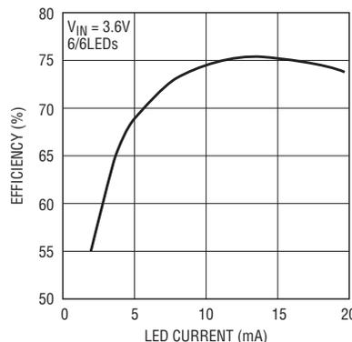
Figure 2. Efficiency of the circuit in Figure 1
