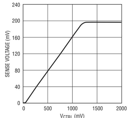
Figure 3. LED sense voltage versus CTRL pin voltage
