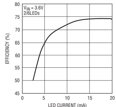
Figure 9. Efficiency of the circuit in Figure 8
