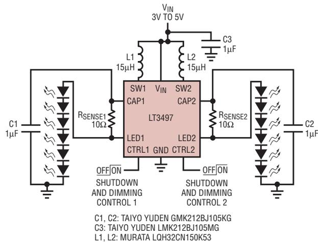
Figure 1. Li-Ion powered driver for twelve white LEDs
