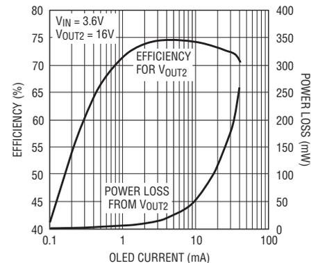
Figure 3. Efficiency of the OLED Driver in Figure 1
