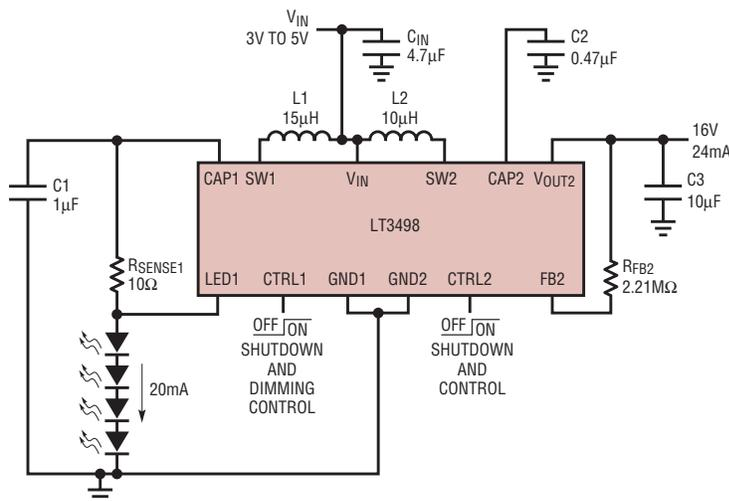
C<sub>IN</sub>, C<sub>2</sub>: X5R OR X7R WITH SUFFICIENT VOLTAGE RATING
