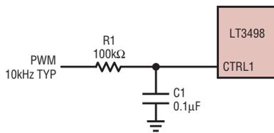
**Figure 6. Filtered PWM dimming**
