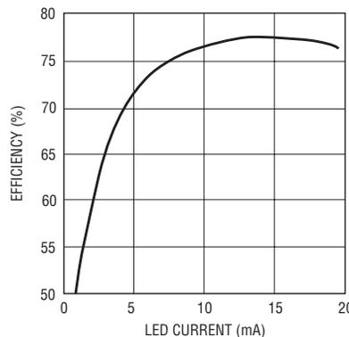
Figure 2. Efficiency of the LED driver in Figure 1
