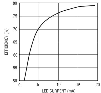
**Figure 10. Efficiency of the LED driver in Figure 9**
