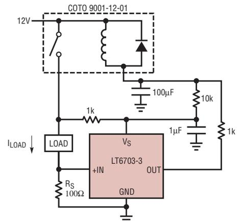
**Figure 7. Latch-off protection circuit with load sensing auto-reset**
