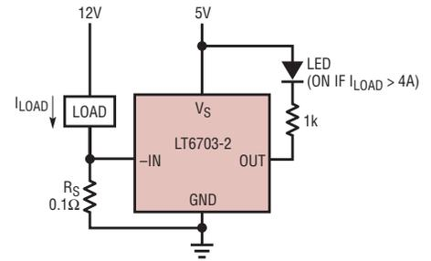
**Figure 5. Low side current sense alarm**
