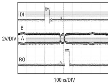
**Figure 8.** The LTC2854 driver delivering a single 50ns pulse through 100ft of Cat 5 cable, which is received by another LTC2854. Both parts have their on-chip termination enabled. Top trace is the input to the transmitting device and the middle and bottom traces are observed at the receiving part.
