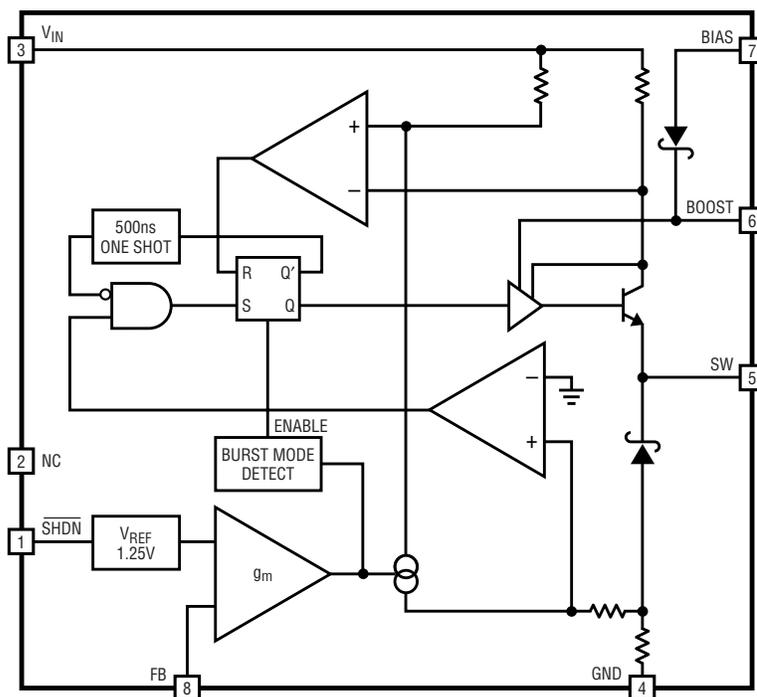
Figure 1. The block diagram of the LT3470 shows the integrated boost and catch Schottky diodes. Inductor current is kept under control at all times by monitoring the  $V_{\text{IN}}$  current as well as the catch diode current, thereby providing short circuit protection even if  $V_{\text{IN}} = 40\text{V}$ .
