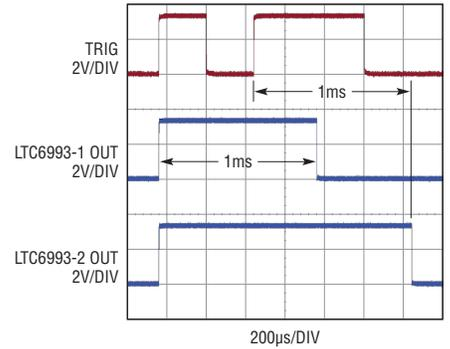
Figure 11. The LTC6993 non-retriggerable and retriggerable functionality
