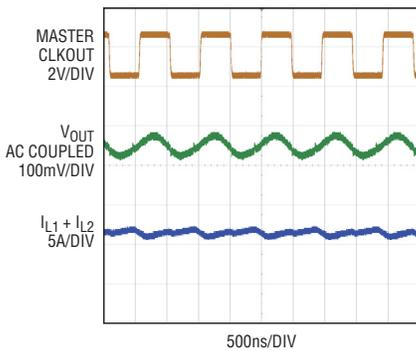
Figure 16. Output ripple at maximum load for the dual phase circuit shown in Figure 15
