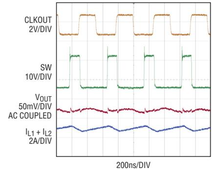
Figure 13. High operating frequency results in low output ripple, even at maximum load
