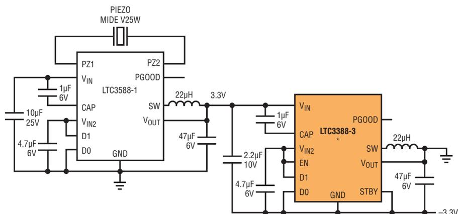
Figure 3: Piezoelectric energy harvester with dual  $\pm 3.3\text{V}$  outputs
