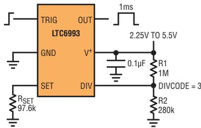
Figure 10. An LTC6993 monostable pulse generator (one-shot)
