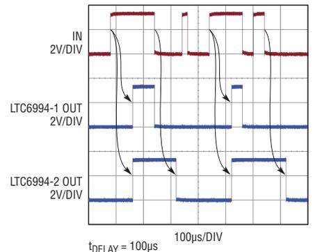
Figure 13. LTC6994 single and double-edge delay functionality
