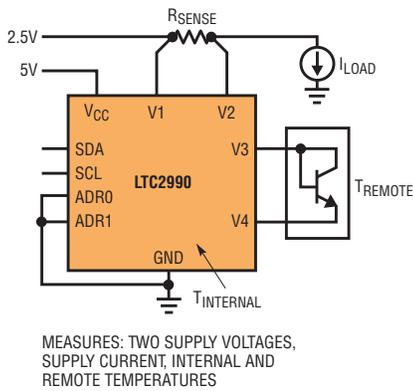
Figure 12. Temperature compensated current sense resistor
