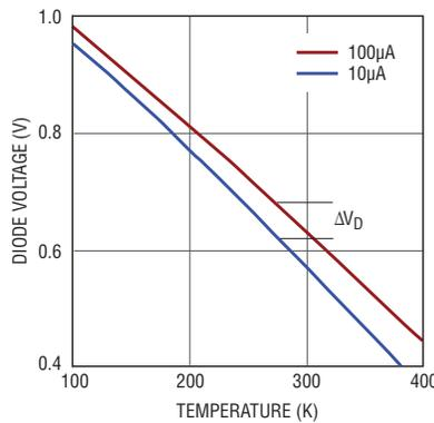
Figure 1. Diode voltage  $V_D$  vs temperature  $T(K)$  for different bias currents
