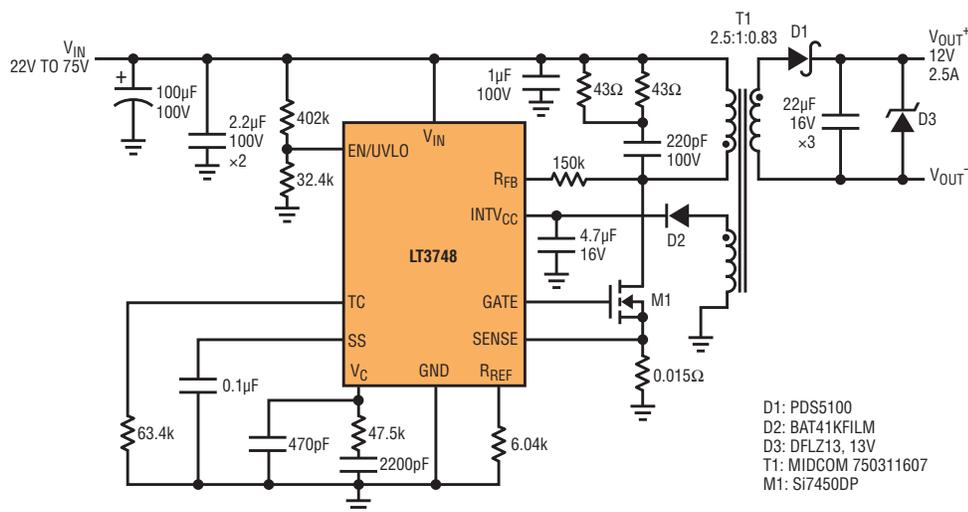
**Figure 6. IGBT controller supply for hybrid and electric vehicle applications**
