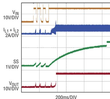
Figure 9. Operating waveforms for a hot plug event
