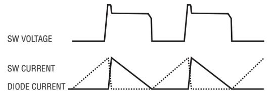
Figure 1. Idealized waveforms for an LT3748-based flyback converter operating in boundary mode
