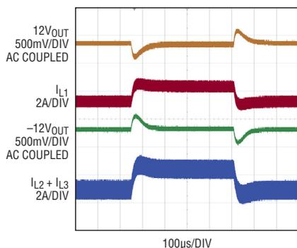
Figure 5. Load step from 0.25A to 0.75A between +12V and –12V rail, with 5V input
