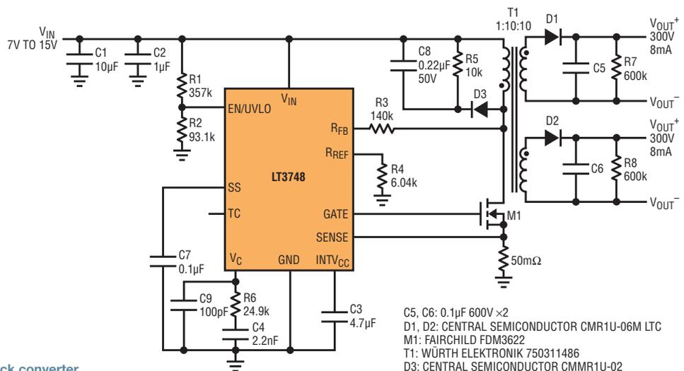
**Figure 7. A ±300V isolated flyback converter**
