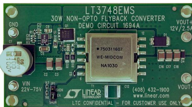
Figure 3. The LT3748 is available in an MSOP-16 package with four pins removed for high voltage operation.
