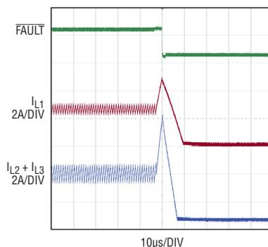
Figure 6. Transient short between rails with 5V input, 0.9A load before short
