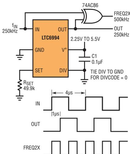
Figure 14. 90° phase-shifted (quadrature) signal generator and frequency doubler
