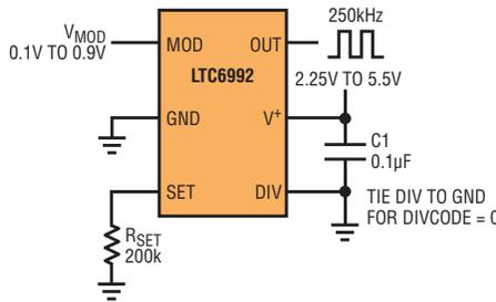
Figure 8. An LTC6992 pulse-width modulator
