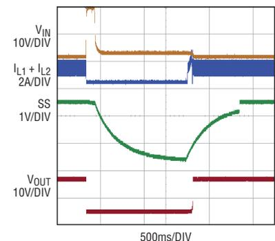
Figure 11. Operating waveforms for a  $V_{IN}$  overvoltage transient
