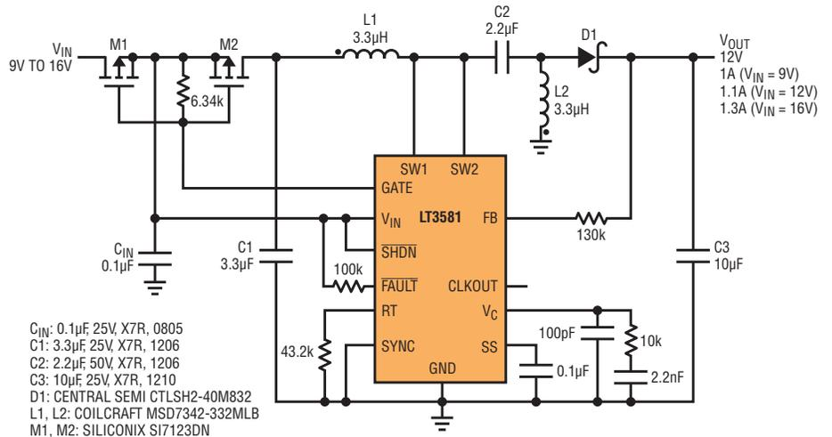
Figure 8. A 9V-16V input to 12V output SEPIC with hot plug, reverse input voltage, and input overvoltage protection
