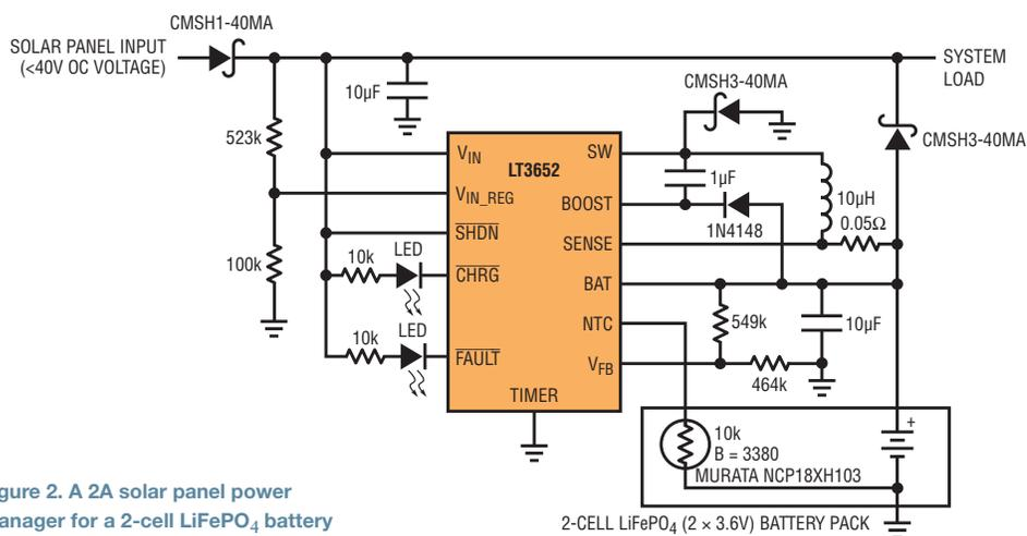
Figure 2. A 2A solar panel power manager for a 2-cell LiFePO<sub>4</sub> battery with 17V peak power tracking
