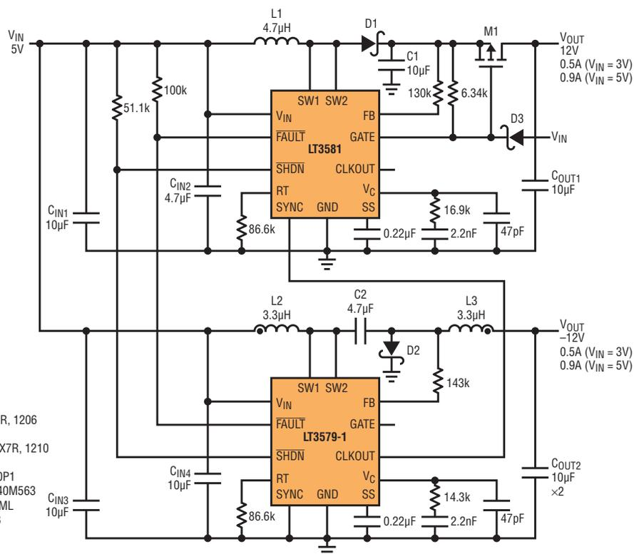
Figure 4. A 3V–5V input to ±12V output converter
