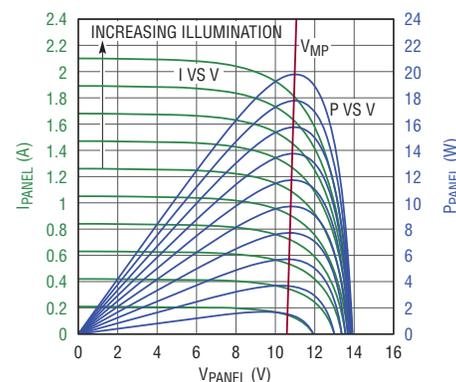
Figure 1. Current vs voltage and power vs voltage for a solar panel at a number of different illumination levels. The panel output voltage at the maximum power point ( $V_{MP}$ ) remains relatively constant regardless of illumination level.
