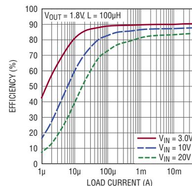
Figure 2: LTC3388-1 Efficiency vs load current for the 1.8V output
