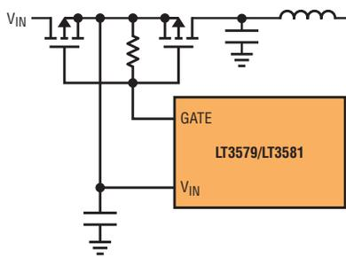
Figure 7. Recommended connections for hot plug, reverse input voltage, and input overvoltage events
