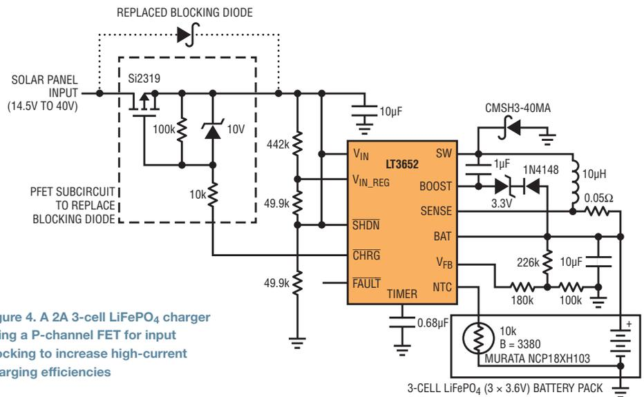
Figure 4. A 2A 3-cell LiFePO<sub>4</sub> charger using a P-channel FET for input blocking to increase high-current charging efficiencies
