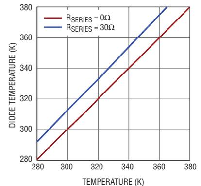
Figure 2. Reported uncompensated diode temperature  $T_D(K)$  vs temperature  $T(K)$  with series resistance
