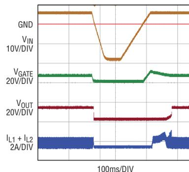
Figure 10. Operating waveforms for a negative  $V_{IN}$  transient
