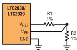
Figure 2. Programming the voltage monitoring mode
