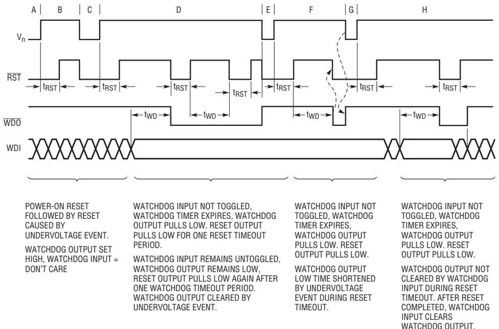
The LTC2938 and LTC2939 are specifically designed to allow a microprocessor to distinguish between resets caused by input supply undervoltage or those due to software malfunction (watchdog timeout).
