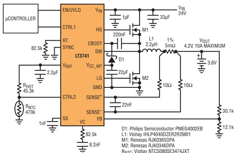
CTRL2 provides the thermal limit control using a temperature dependent resistor.
