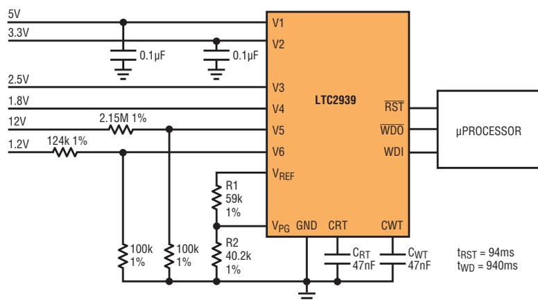
A single pin ( $V_{PG}$ ) allows the selection of one of 16 possible threshold configurations. This programmability eliminates the need to qualify, source and stock unique part numbers for different threshold voltage combinations.
