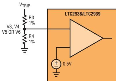
Figure 3. Setting the positive adjustable trip point,  $V_{TRIP} = 0.5V \cdot (1 + R3/R4)$
