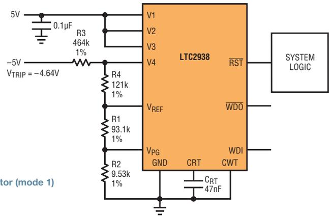
Figure 10. A  $\pm 5\text{V}$  supply monitor (mode 1) with unused inputs disabled
