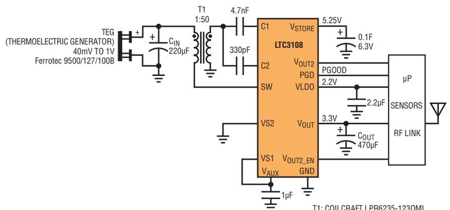
Figure 13. Wireless sensor application, powered by a TEG
