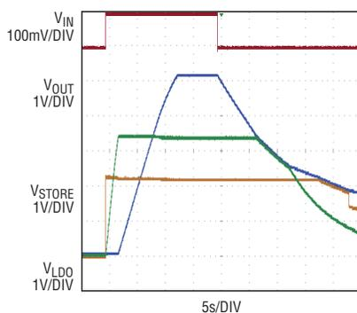
Figure 3. Voltage sequencing during power-up and power-down
