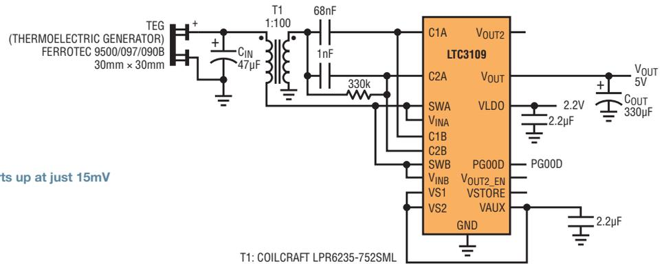
Figure 17. Unipolar converter using the LTC3109 starts up at just 15mV
