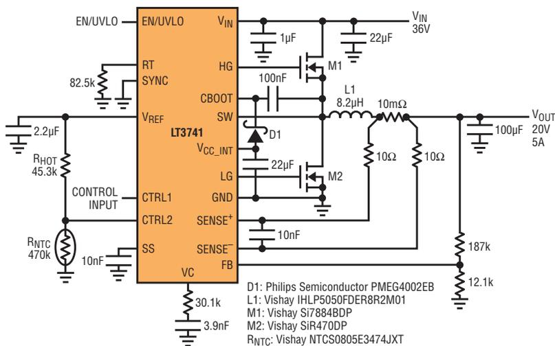
Figure 6. A 100W 20V/5A constant-current, constant-voltage step-down converter
