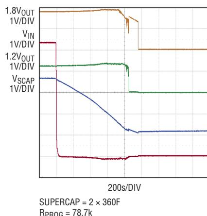
Figure 4. Supercapacitor backup time supporting a 20W Load
