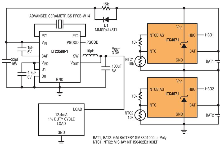
With a few easy-to-use components, it is possible to build a complete compact energy-harvesting power subsystem for wireless sensor-transmitters.
