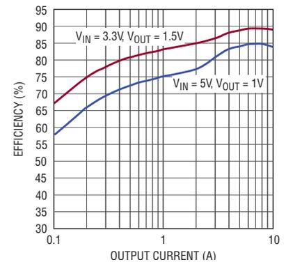
Figure 6. LTM4611 Burst Mode operation efficiency
