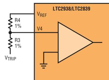
Figure 4. Setting the negative adjustable trip point,  $V_{TRIP} = -V_{REF} \cdot (R3/R4)$
