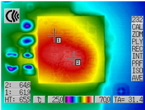
Figure 7. Top thermal image of an LTM4611 regulator producing 1.5V at 15A from a 5V input. Power loss is 3.5W. No-airflow bench testing results in a 65°C surface temperature hotspot.
