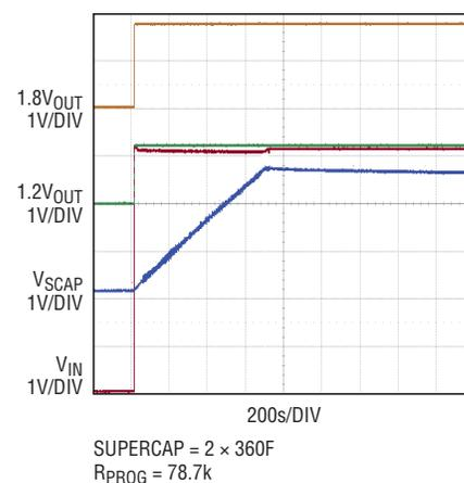
Figure 5. Recharge of series-connected pair of 360F supercapacitors
