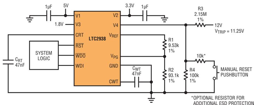
Figure 9. Quad-supply monitor (mode 14) with pushbutton reset
