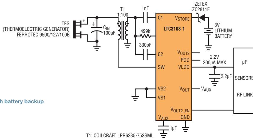
Figure 14. Energy harvester with battery backup
