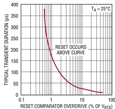
**Figure 6. Transient duration versus comparator overdrive**
