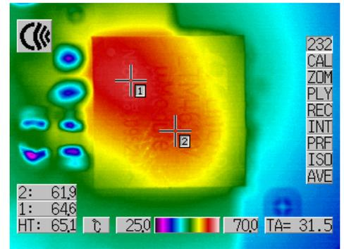
Figure 8. Top thermal image of an LTM4611 regulator producing 1.5V at 15A from a 1.8V input. Power loss is 3.2W. No-airflow bench testing results in a 65°C surface temperature hotspot.
