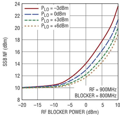
Figure 2. LTC5540 noise figure vs RF blocker level
