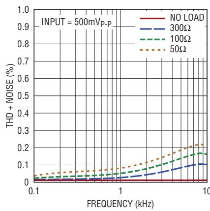
Figure 19. LTC6262 bridge driver THD and noise with different loads vs amplitude at 1kHz
