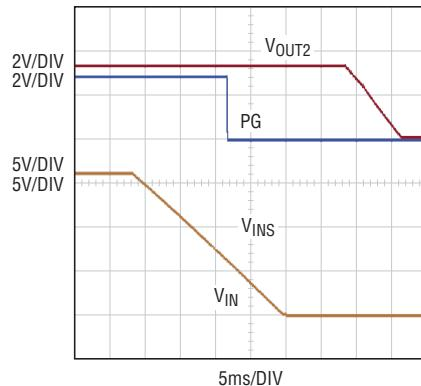
**Figure 2.** When the input voltage  $V_{IN}$  drops, the converter U1 boosts  $V_{OUT1}$  to maintain  $V_{INS}$  at 8V.  $V_{INS}$  provides power to keep  $V_{OUT2}$  in regulation for over 20ms after  $V_{IN}$  drops out.
