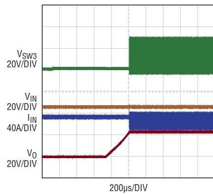
**Figure 6.** Start-up waveform with LTC7820 pre-balance shows elimination of inrush current
