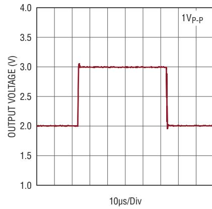
The low supply current of these op amps at the bandwidth and noise performance allows for excellent fidelity at a fraction of the usual dissipation in portable audio equipment. As with active filters, revisiting portable audio equipment headphone drivers is a rational enterprise, given the unique capabilities of the LTC6261.
