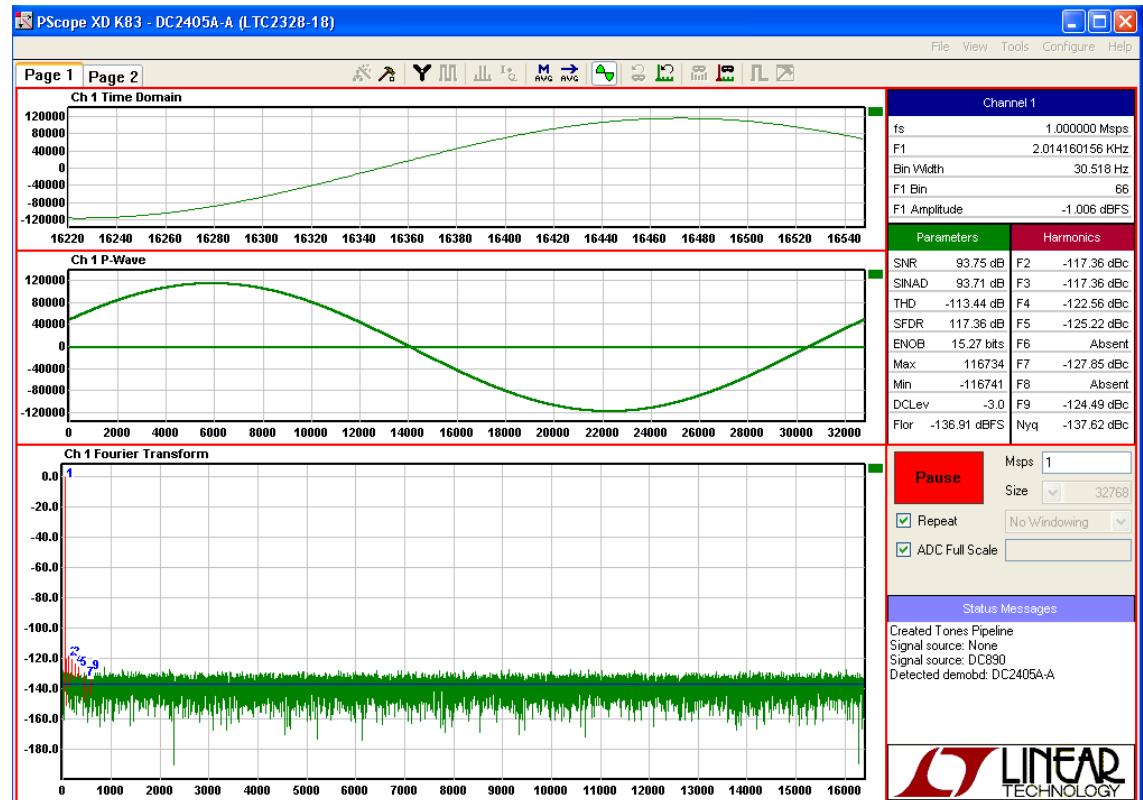
Figure 7. PScope plot of the DC2405A demonstration circuit
