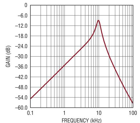
Figure 5. Bandpass filter gain/phase vs frequency
