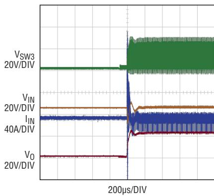
**Figure 5.** Start-up waveform without pre-balance shows large inrush current
