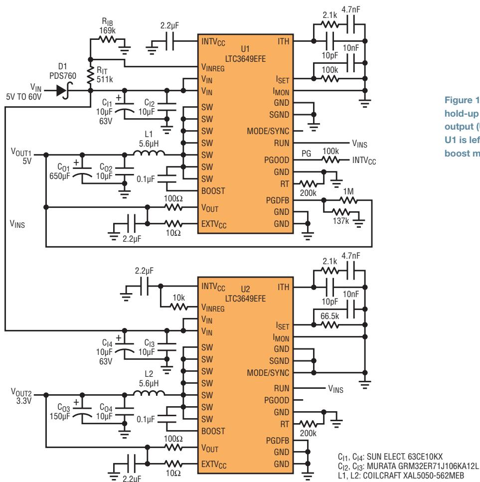
**Figure 1.** The 5V output converter (U1) provides hold-up power for protected load on the 3.3V output (U2). Note that the pin MODE/SYNC of U1 is left floating, allowing the LTC3649 to enter boost mode.
