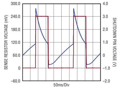
Figure 10. LED blinker current
