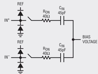
**Figure 3.** Simulation schematic of SAR ADC analog input equivalent circuit
