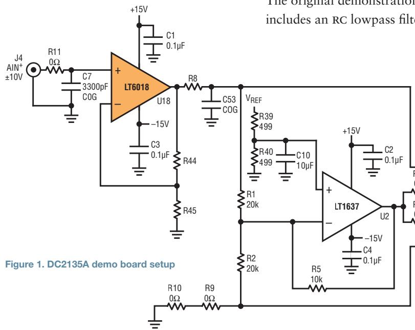
Figure 1. DC2135A demo board setup
