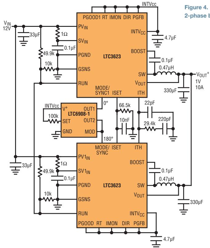
**Figure 4.** 12V to 1V at ±10A 2-phase buck converter
