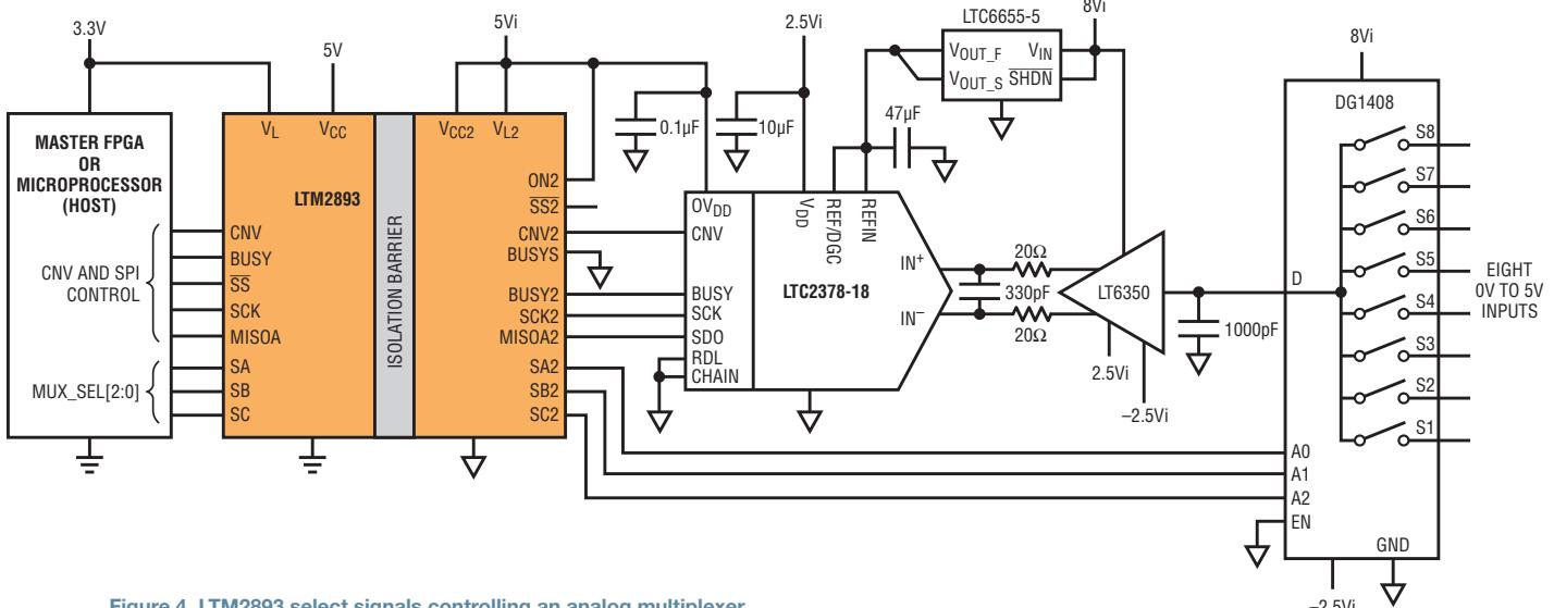
**Figure 4.** LTM2893 select signals controlling an analog multiplexer
