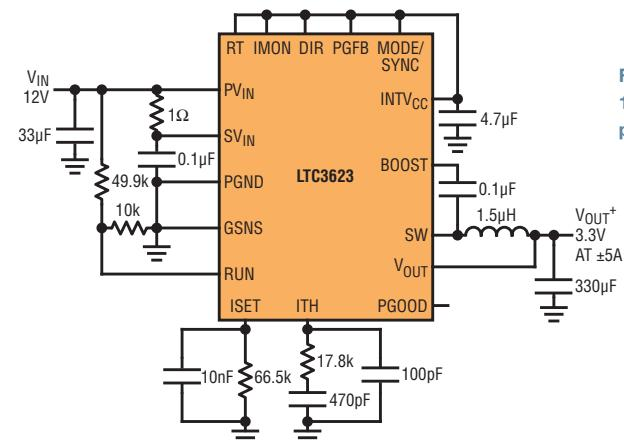
Figure 1. High efficiency 12V to 3.3V 1MHz step-down regulator with programmable reference
