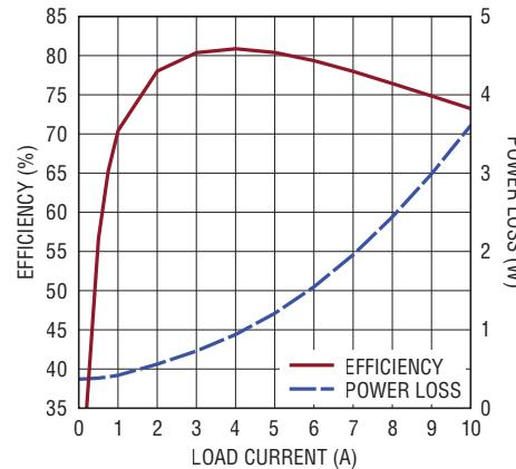
Figure 2 shows the continuous and discontinuous conduction mode efficiency and power loss. Discontinuous conduction mode significantly improves light load efficiency while adding a slight increase in output voltage ripple. Figure 3 shows the load-step response with only 330µF of output capacitance.
