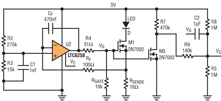
Figure 9. LED driver with self-oscillation
