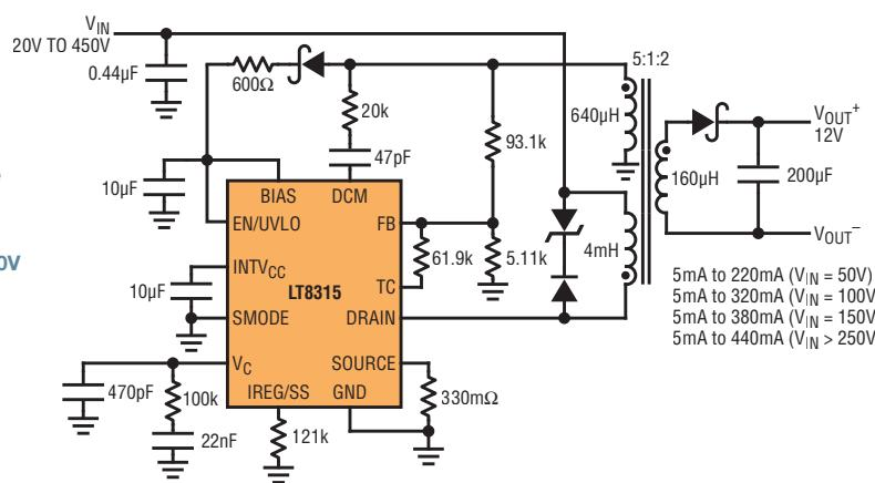
The LT8315 integrates a 630V MOSFET and control circuitry in a thermally enhanced 20-pin TSSOP package with four pins removed for high voltage spacing. By sampling the isolated output voltage from the third winding, no opto-coupler is required for regulation. The output voltage is programmed with two external resistors and a third optional temperature compensation resistor.
