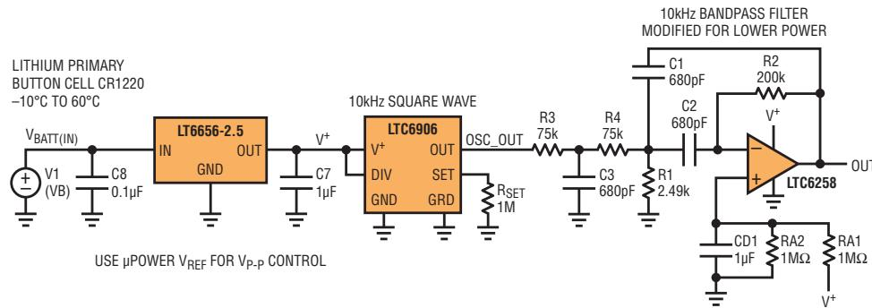
**Figure 8.** Oscillator and filter with a regulated supply
