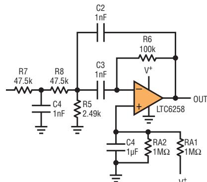
Figure 4. 10kHz bandpass filter
