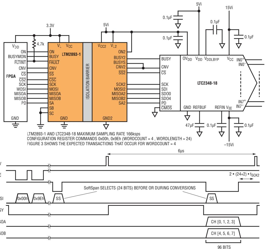
Additionally, with ADCs that support chaining (Figure 5), up to eight ADCs can be connected to a single LTM2893. Reading more than two parallel ADCs requires a write to the configuration register in the LTM2893 to select the number of devices. The configuration register allows the selection of two, four, six or eight devices to be accessed through the two MISOA and MISOB SPI outputs.
