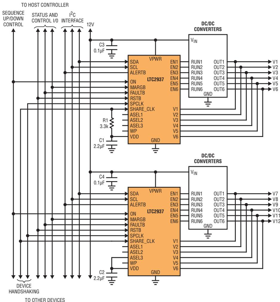
The LTC2937 simplifies power system sequencing and supervision. It requires very little board real estate for a complete system. It is flexible and reconfigurable, yet autonomous through its EEPROM memory. It can operate on its own, or in concert with other chips in a large system, seamlessly orchestrating the operations of up to 300 power supplies.
