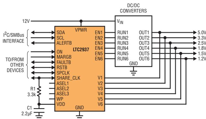
Each of the LTC2937's six channels has two dedicated comparators to accurately monitor over- and undervoltage conditions to within  $\pm 0.75\%$ . The comparator thresholds are individually programmable over a range of 0.2V to 6V with 8-bit resolution.
