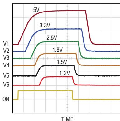
Figure 2. Power supply sequencing waveforms
