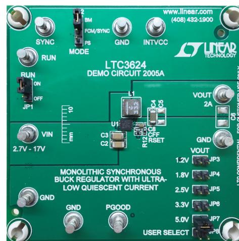
Figure 2. Small total solution size: 13mm × 12mm
