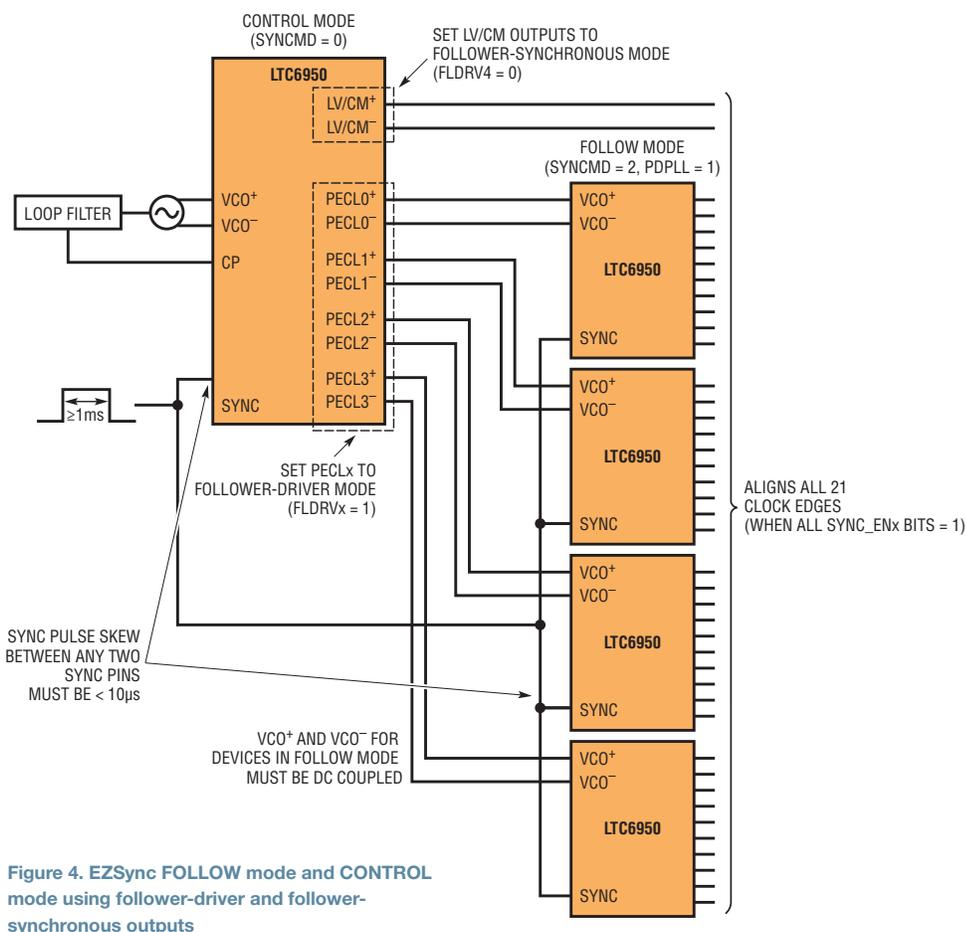
Figure 4. EZSync FOLLOW mode and CONTROL mode using follower-driver and follower-synchronous outputs
