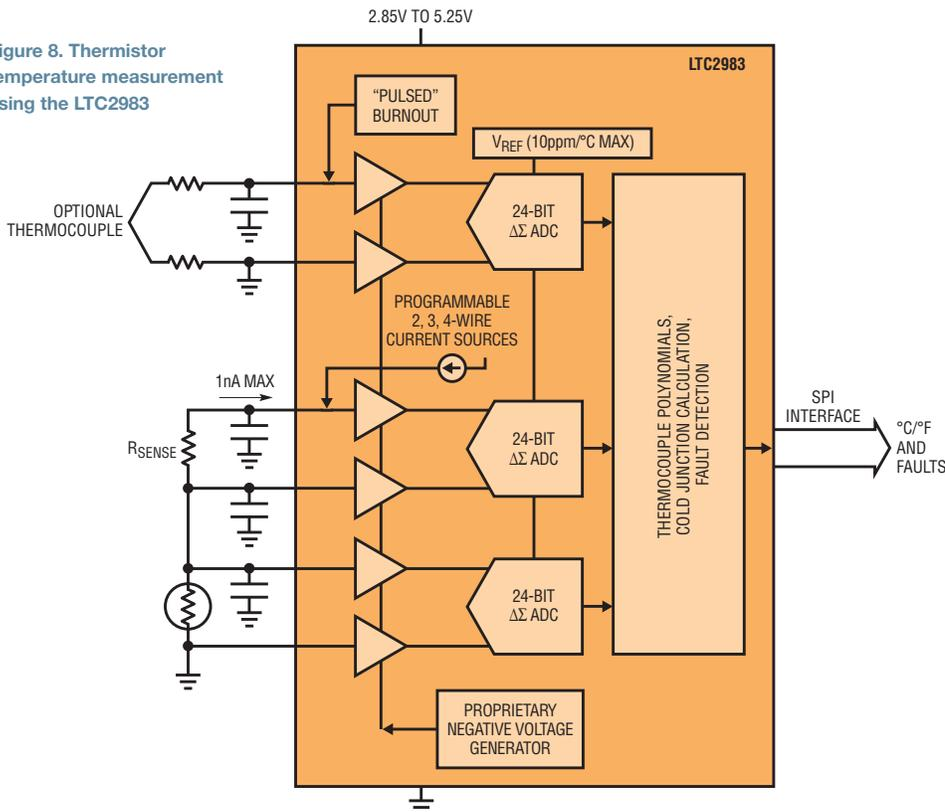
The LTC2983 is a groundbreaking, high performance integrated temperature measurement system that directly digitizes thermocouples, RTDs, thermistors and diodes with laboratory grade precision. It features high accuracy, an easy sensor interface and tremendous flexibility.
