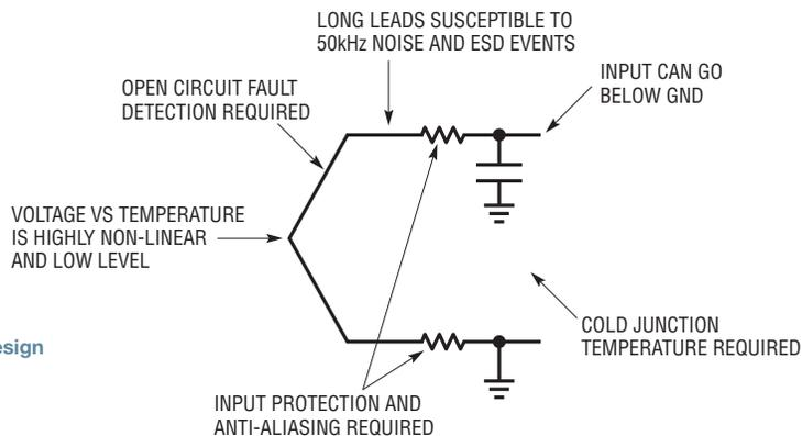
Figure 2. Thermocouple design challenges
