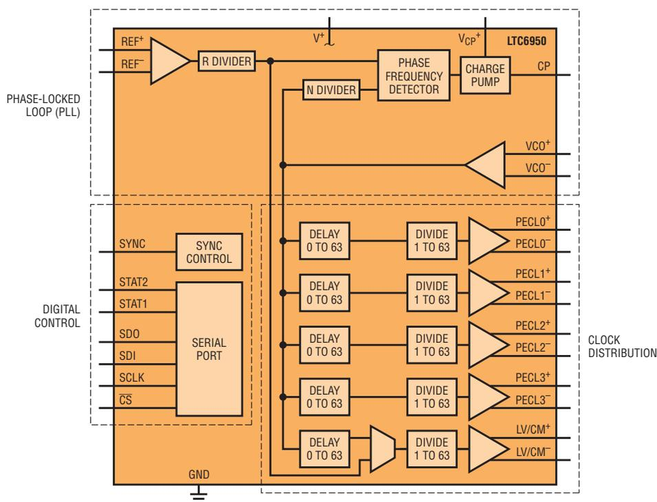
The LTC6950 is the first device to offer Linear Technology's EZSync technology, which simplifies aligning multiple clocks across multiple parts, boards and systems. LTC6950 performance levels enable direct clocking of high performance data converters, simplifying system design and reducing system cost.
