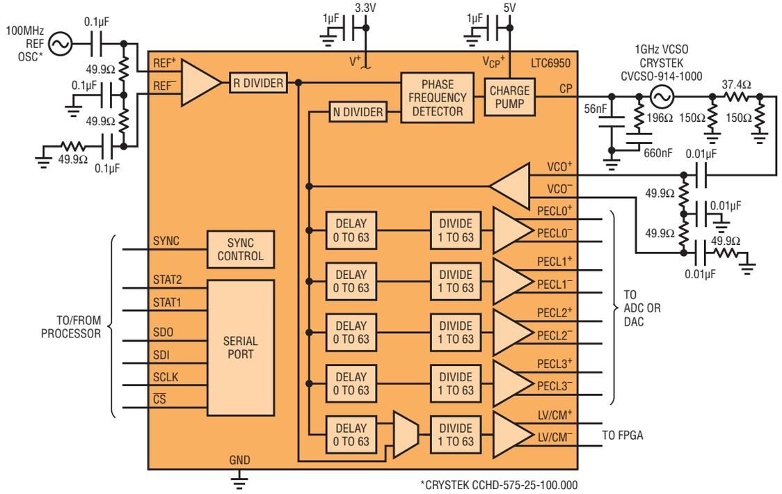
Figure 11. ClockWizard LTC6950 loop filter design
