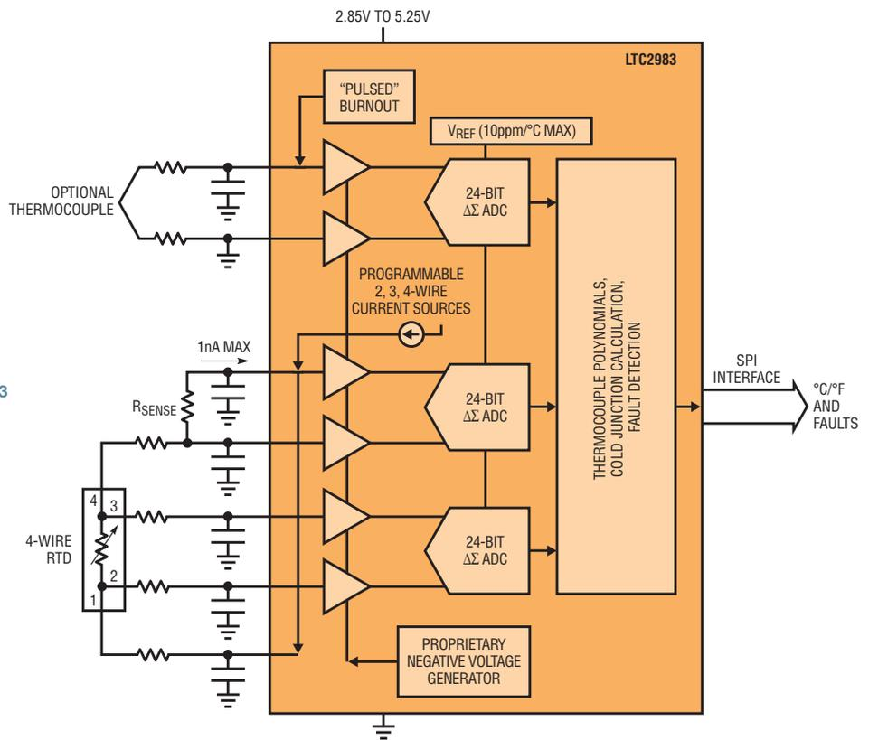
Figure 6. RTD temperature measurement using the LTC2983
