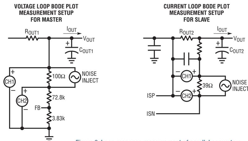
Figure 6. Loop response measurement of parallel converters
