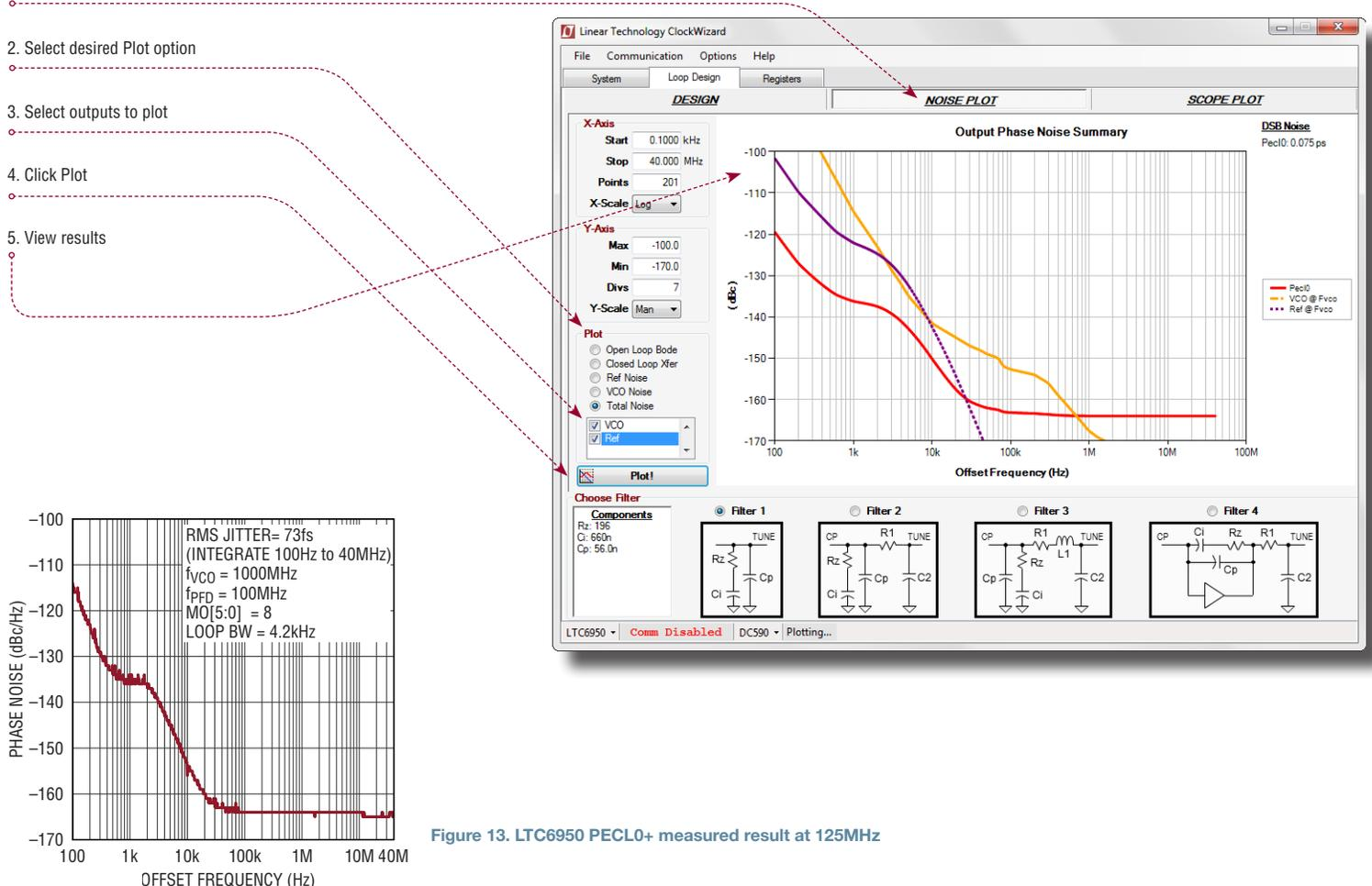
Figure 13. LTC6950 PECL0+ measured result at 125MHz
