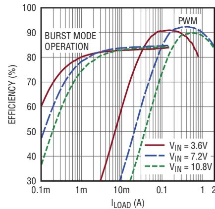
Figure 4. 5V output efficiency from one, two and three Li-ion cells
