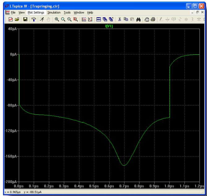
Figure 8. The trap ringing example circuit of Figure 6 run in PSpice (left) does not exhibit trap ringing, but produces other artifacts most likely due to an error in the implementation of the Yang-Chatterjee charge model. LTspice (right) produces the correct result.
