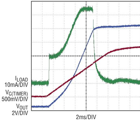
Figure 2. (Case 1) Pure capacitive load. Operating point leaves current limit mode in the third area, where current limit is  $I_{LIMIT}$ .
