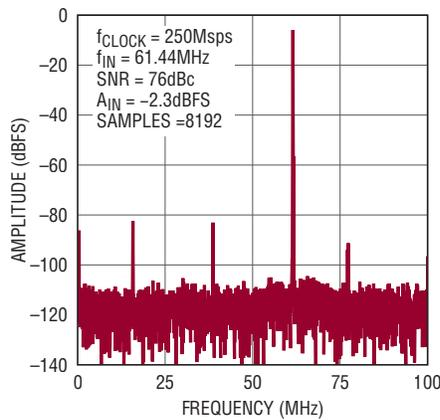
Figure 8. LTC6950 direct ADC clocking performance
