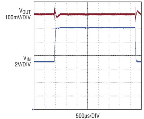
Figure 7. Line response for  $V_{OUT} = 3.3V$ ,  $V_{IN}$  stepped from 7.2V to/from 12V
