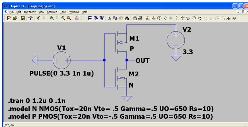
Figure 6. Circuit prone to trap ringing
