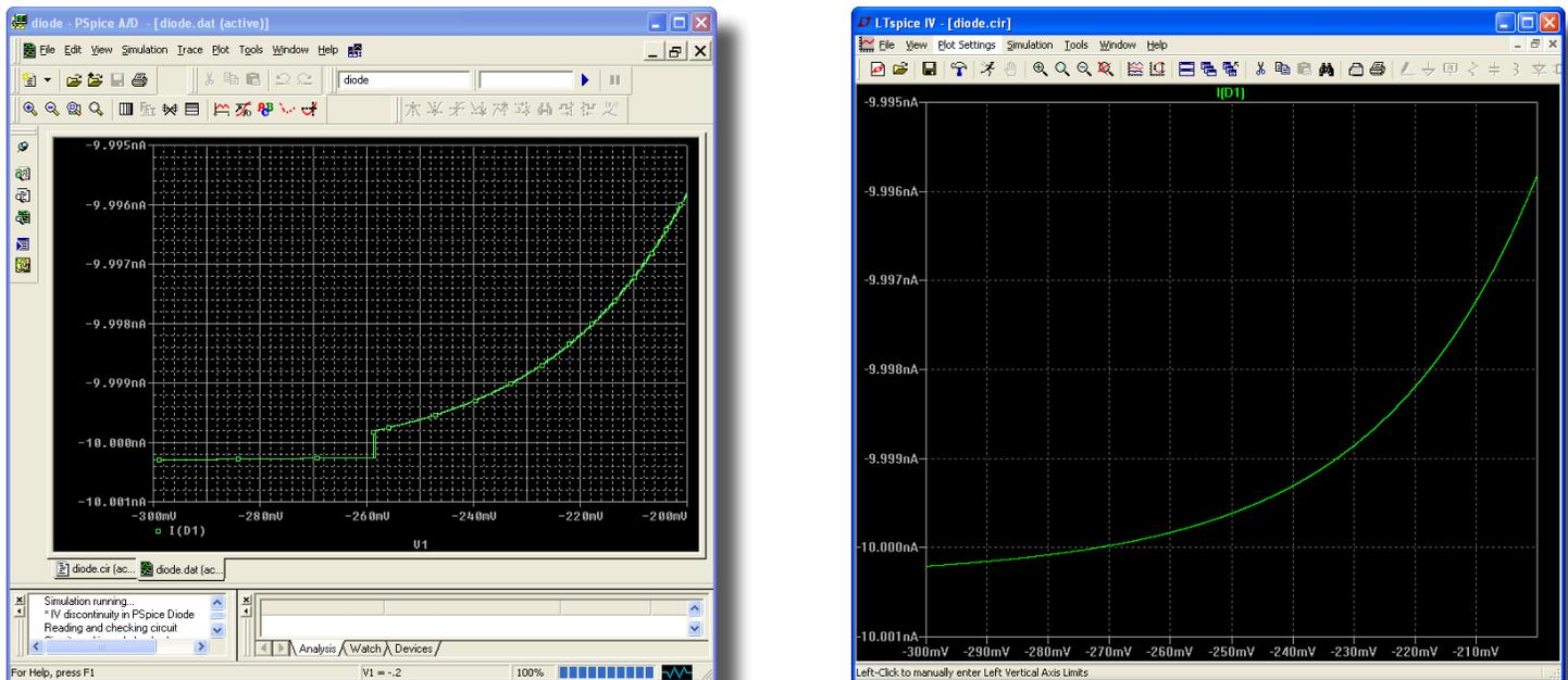
Figure 1. Discontinuity in PSpice (left) diode I-V curve vs continuous diode I-V curve in LTspice (right). Discontinuities negatively impact a simulator's ability to solve nonlinear circuits.
