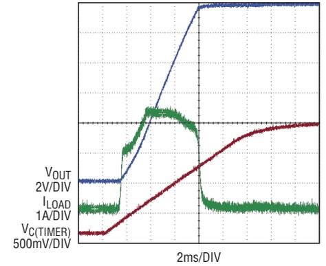
Figure 4. (Case 4) Pure capacitive load with a limited  $S_O$  (natural output voltage slew rate). Operating point leaves current limit mode in the second area, where current limit rises linearly.
