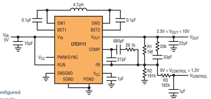
Figure 8. LTC3111 configured as a variable output supply
