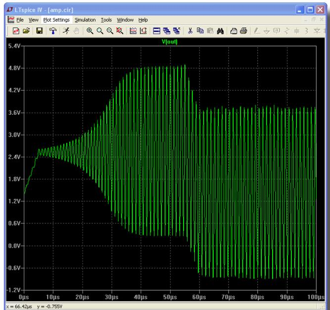
Figure 5. Simulated output from an unstable power amplifier in the face of a large signal transient. PSpice (left) incorrectly indicates the circuit as stable, while LTSpice (right) correctly reveals the instability.
