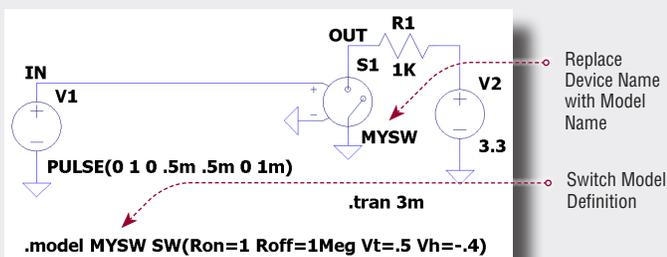
One classic application of voltage-controlled switches is simulating open-circuit and short-circuit conditions. In the example shown, two switches simulate a short- and open-circuit condition on an LED string.
