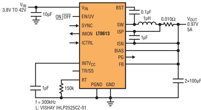
**LT8613 1V STEP-DOWN WITH 5A OUTPUT CURRENT LIMIT**
