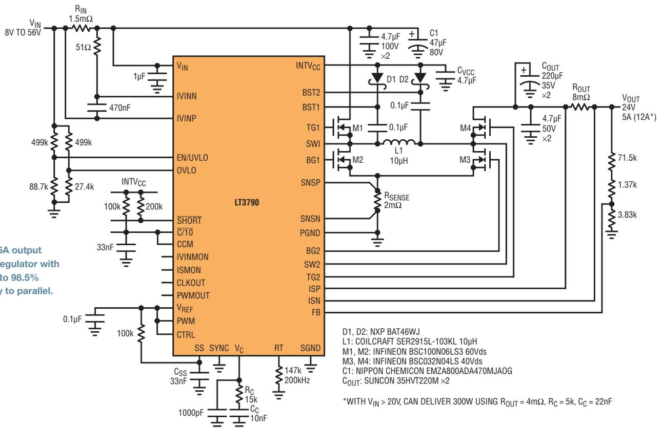
Figure 3. Two LT3790 24V voltage regulators are easy to parallel for double the output with limited discrete component temperature rise.
