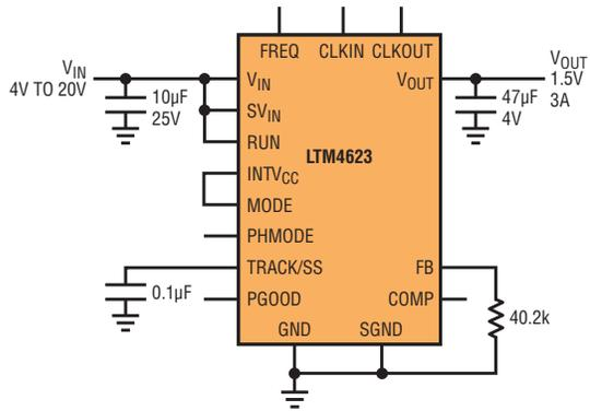
**LTM4623 4V–20V VIN, 1.5V VOUT AT 3A WITH ULTRALOW PROFILE (< 2mm)**
