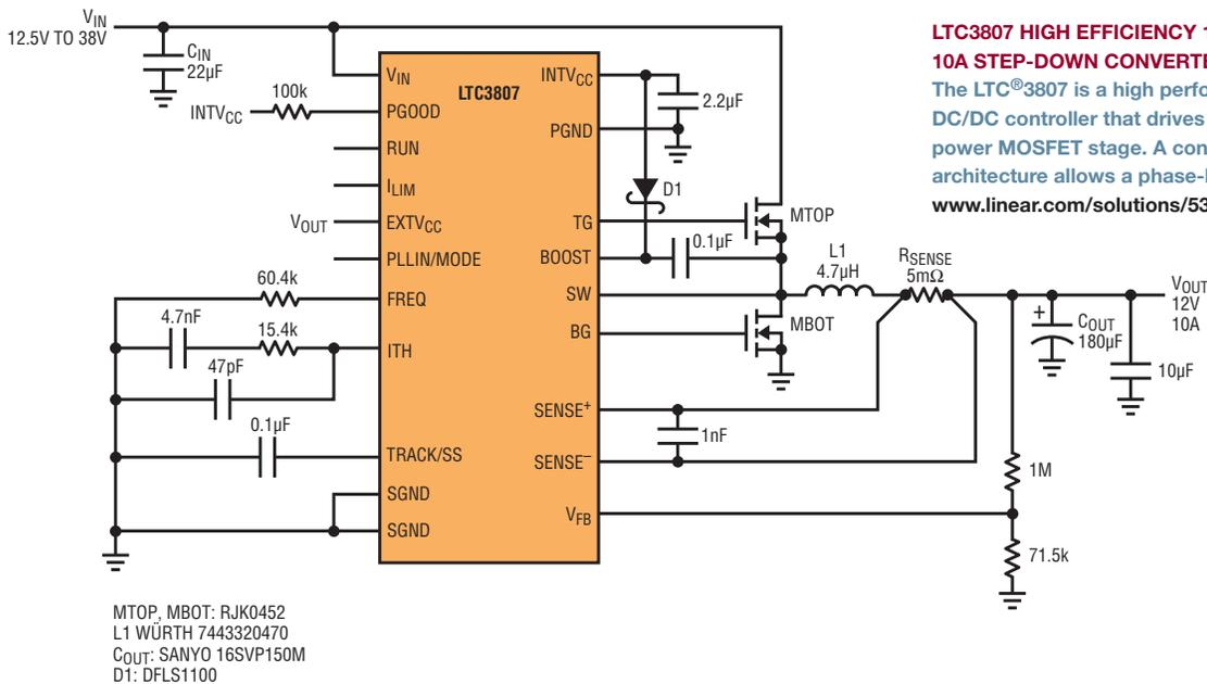
**LTC3807 HIGH EFFICIENCY 12V OUTPUT AT 10A STEP-DOWN CONVERTER**
