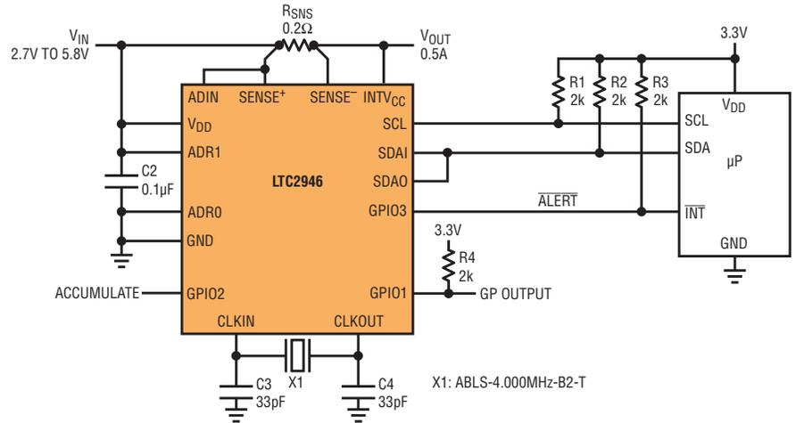
POWER FOR REVERSE PATH = CODE<sub>ADIN</sub> × CODE<sub>VDD</sub> TO BE PERFORMED BY µP
