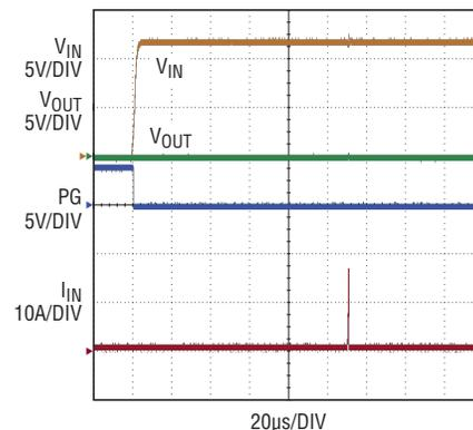
Figure 5. Start-up into a short circuit
