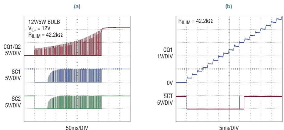
While IO-Link drivers normally see capacitive loading of at most 4nF when connected by cable to another IO-Link PHY, the LTC2874 and LT3669 can drive more than 100mA (up to 250mA for the LT3669) for compatibility with legacy sensors and a variety of industrial loads. For example, this drive strength is sufficient to operate miniature incandescent lamps used in 12V and 24VDC systems.
