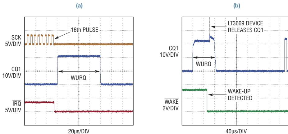
While sensors built with digital IO-Link interface are likely less susceptible to noise than older analog-output models, their wide-swing (24V), single-ended signaling through unshielded wire can produce electromagnetic interference (EMI). The CQ line drivers of both the LTC2874 and LT3669 use slew-rate limiting circuitry to reduce the high frequency content of signaling emissions. Both products also offer a slow edge rate mode.
