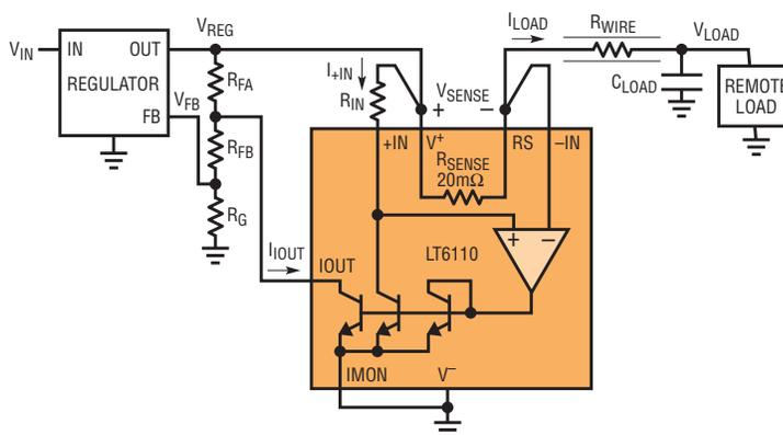
For precise load regulation, an accurate estimate of the resistance between the power source and load is required. If  $R_{\text{WIRE}}$ ,  $R_{\text{SENSE}}$  and the resistance of the cable connectors and PCB traces in series with the wire are accurately estimated, the LT6110 can compensate for a wide range of voltage drops to a high degree of precision.
