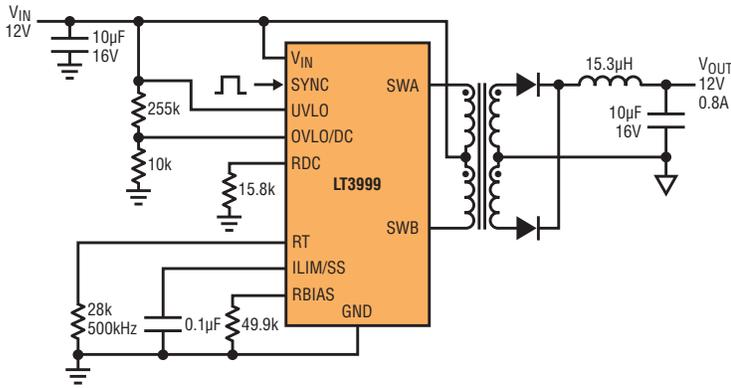
**LT3999 12V TO 12V, 10W LOW NOISE ISOLATED DC/DC CONVERTER**
