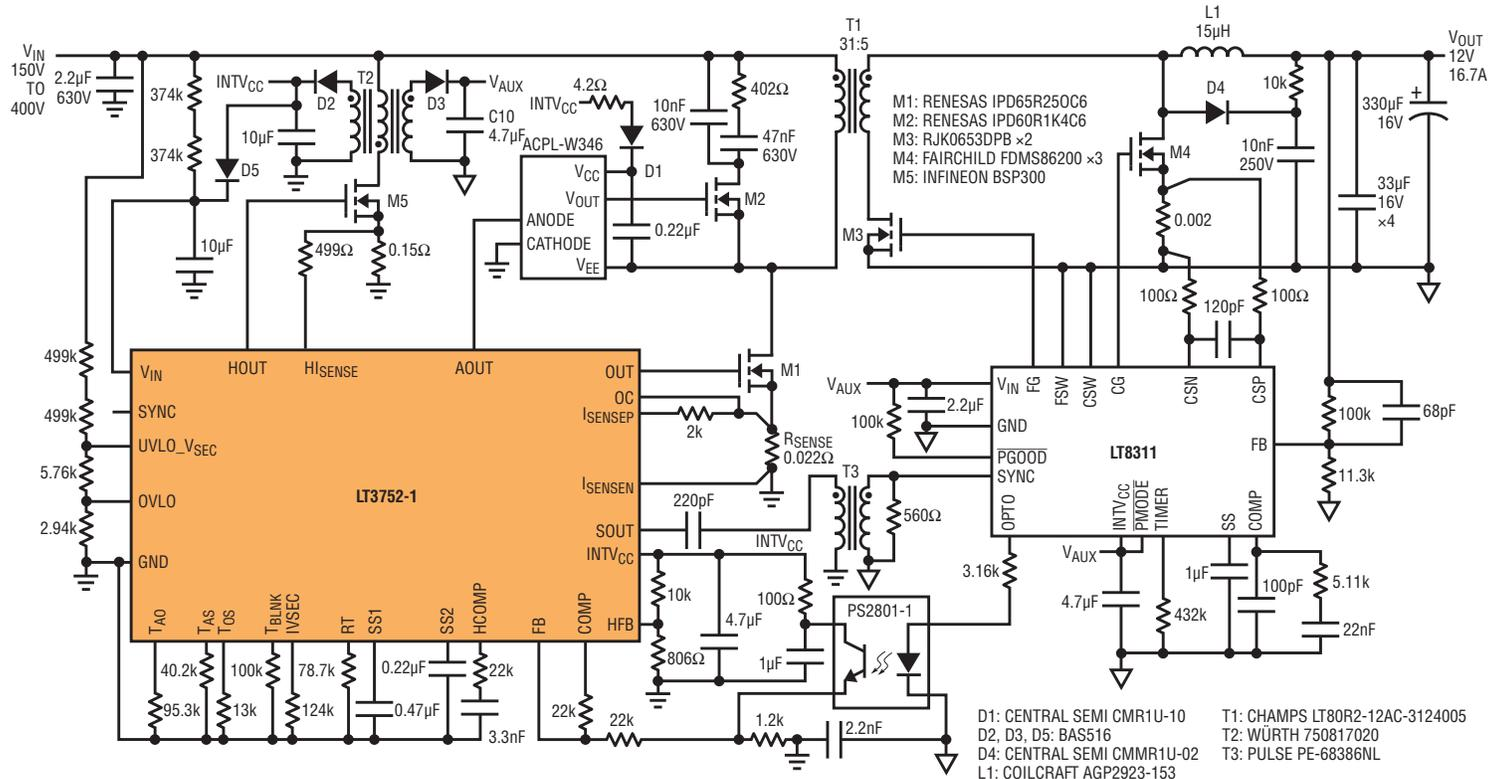
Figure 9. 150V–400V input, 12V/16.7A output isolated forward converter
