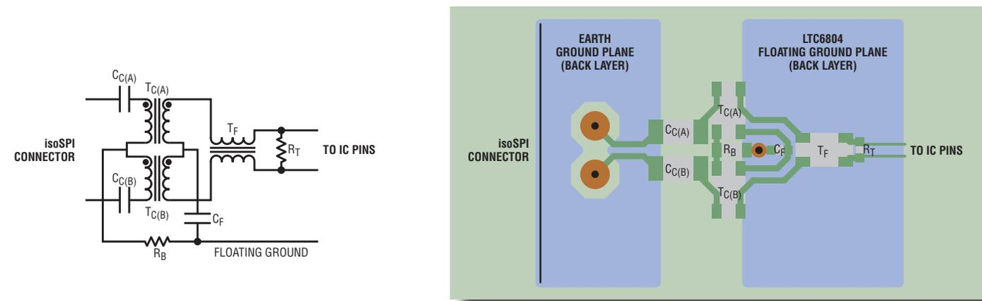
Figure 8. Complete high voltage isoSPI bus with echo control
