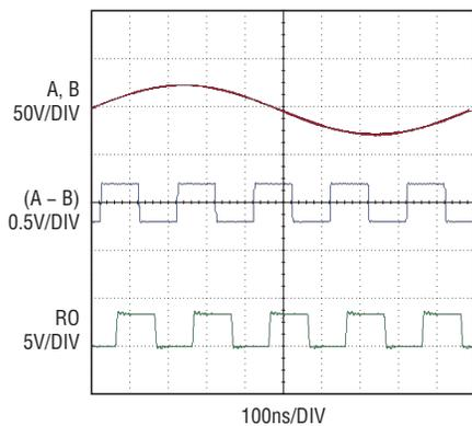
Figure 2. LTC2865 receiving 10Mbps  $\pm 200mV$  differential signal with 1MHz 50VP-P common mode sweep
