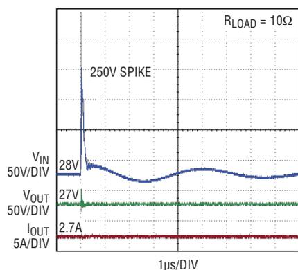
Figure 8. Positive input spike
