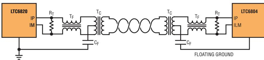
Figure 2. AC-coupled isoSPI point-to-point link for increased voltages
