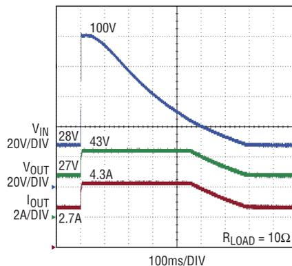
Figure 6. MIL-STD-1275D 100V/500ms surge test
