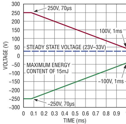
Figure 2. Envelope of spike in generator-only mode
