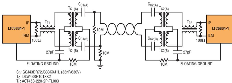
Use an AC-coupling method to mitigate the cost impact of high voltage isoSPI systems, eliminating the double insulation requirement on magnetics. Cost can be further reduced by replacing specialty toroidal transformer magnetics with inexpensive bobbin-wound common-mode-choke (CMC) components. Both the capacitors and CMCs are relatively low profile surface-mount chip components.
