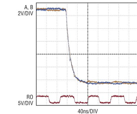
Figure 3. LTC2865 receiving 20Mbps  $\pm 200mV$  differential signal with  $-12V$  36ns fall time common mode step
