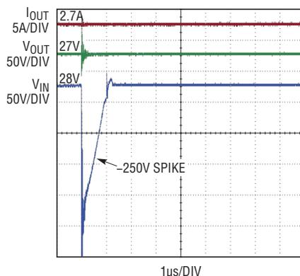
Figure 9. Negative input spike
