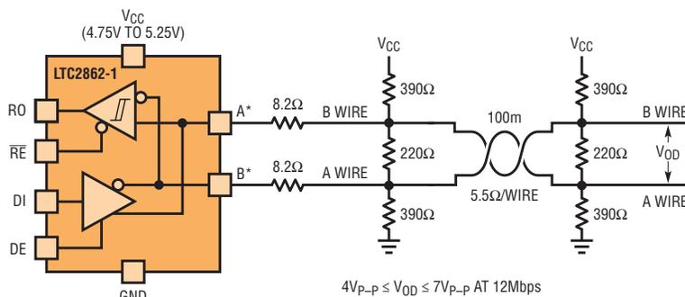
**Figure 10.** LTC2862-1 PROFIBUS compatible line interface
