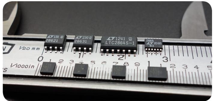
However, most high voltage tolerant RS485 transceivers lack the performance and features of the latest non high voltage tolerant RS485 transceivers. The LTC2862–LTC2865 transceivers fill this gap by combining fault tolerance with the expanded capabilities demanded in the specifications for contemporary network applications.
