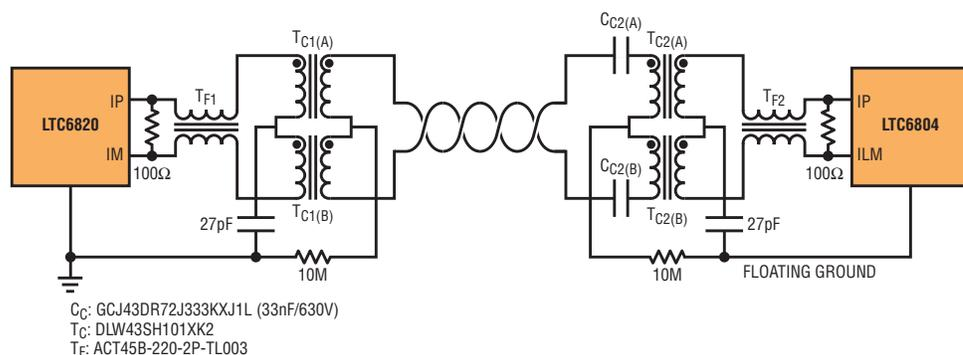
Figure 4. Complete high voltage isoSPI point-to-point link
