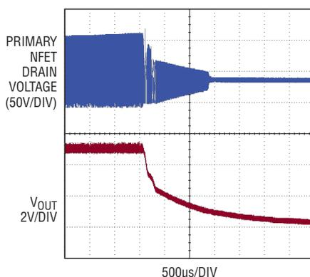
Figure 4. Shutdown waveforms of circuit in Figure 5 showing soft-stop in action
