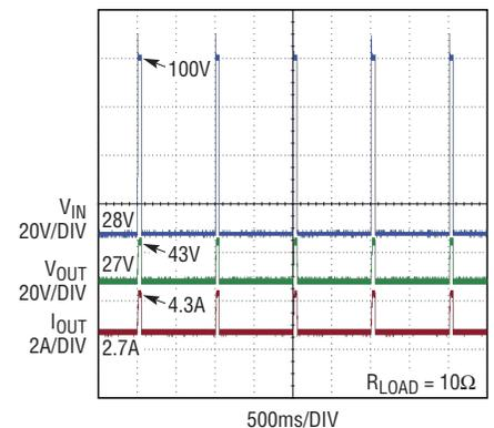
Figure 7. MIL-STD-1275D 100V/50ms surge repeated five times
