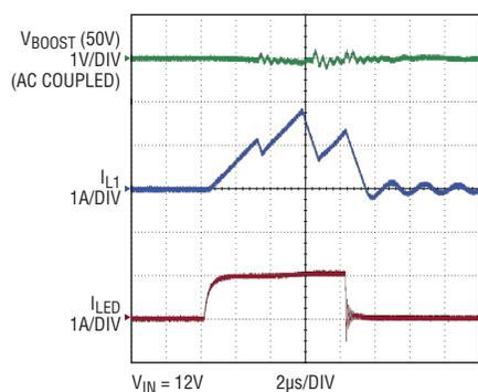
Figure 4. Dual boost-then-buck mode LED driver PWM dimming waveform. 1000:1 dimming at 120Hz.
