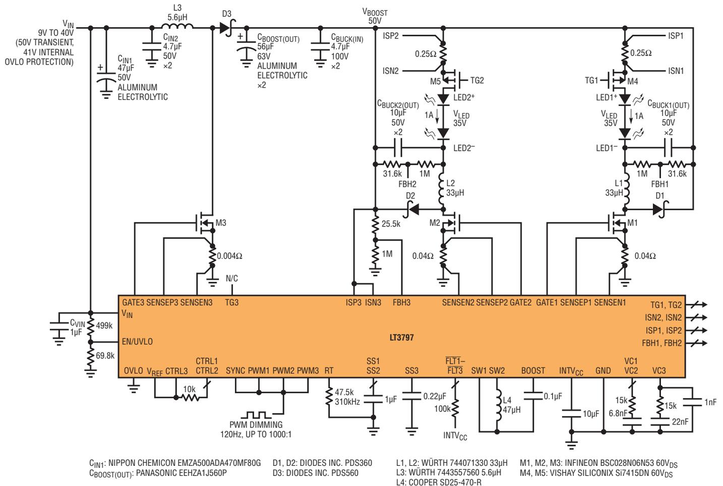
An extra benefit of the boost-then-buck mode driver is the reduced conducted EMI versus a similarly rated buck-boost regulator. Boost converters typically have lower conducted EMI around the AM band than buck converters due to the location of the main inductor in series with the input. In a boost-then-buck scheme, the inductor is in series with the input, versus a buck-boost single inductor between the buck and boost stages.
