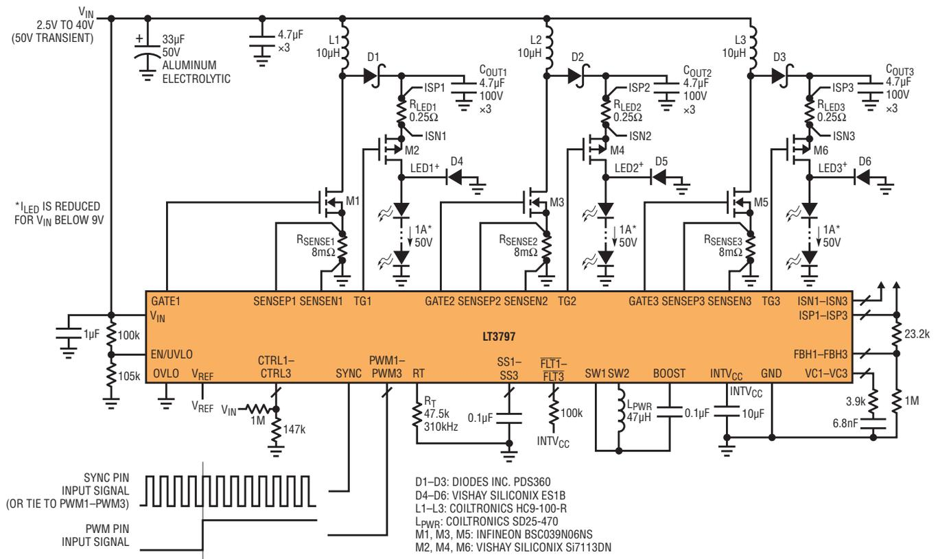
Higher PWM dimming ratios can be achieved by a buck LED driver than by a boost mode driver. To achieve high LED dimming ratios from a wide-ranging input, low input voltages can be boosted to an intermediate voltage with a preregulator. The intermediate, boosted output serves as input to buck-mode LED drivers. Figure 2 shows a boost-then-buck scheme achieved using a single LT3797.
