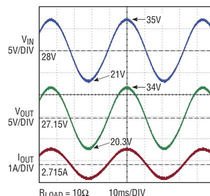
Figure 10. 14V<sub>p-p</sub> input ripple condition
