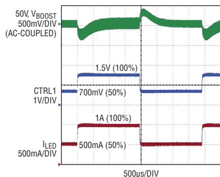
Figure 3. Analog dimming transient from 50% (500mA) to 100% (1A) full-scale current shows high bandwidth of buck mode, even as the boost stage recovers at its own, regular speed.
