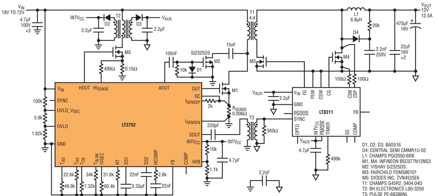
In an active volt-second clamp scheme, the accuracy of  $V_{OUT}$  depends heavily on the accuracy of the volt-second clamp. Competing volt-clamp solutions use an external RC network which suffers from a number of error sources. To ensure accurate regulation part to part, the LT3752, LT3752-1 and LT3753 feature trimmed timing capacitor and comparator thresholds.
