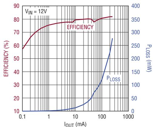
The LTC3245 achieves efficiency of 80% when delivering 5V, 100mA from a 12V source, significantly higher efficiency than an LDO, making it possible to avoid the space and cost requirements of an LDO with a heat sink.
