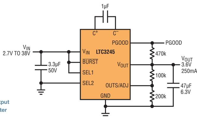
Figure 5. A 3.6V output buck-boost converter
