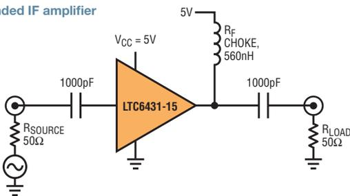
Noise (characterized by NF) limits an amplifier's sensitivity at low input signal amplitudes, while linearity (characterized by OIP<sub>3</sub>) limits sensitivity at high input amplitudes. Taken together, these two metrics, NF and OIP<sub>3</sub>, define the amplifier's useful dynamic range for a signal.
