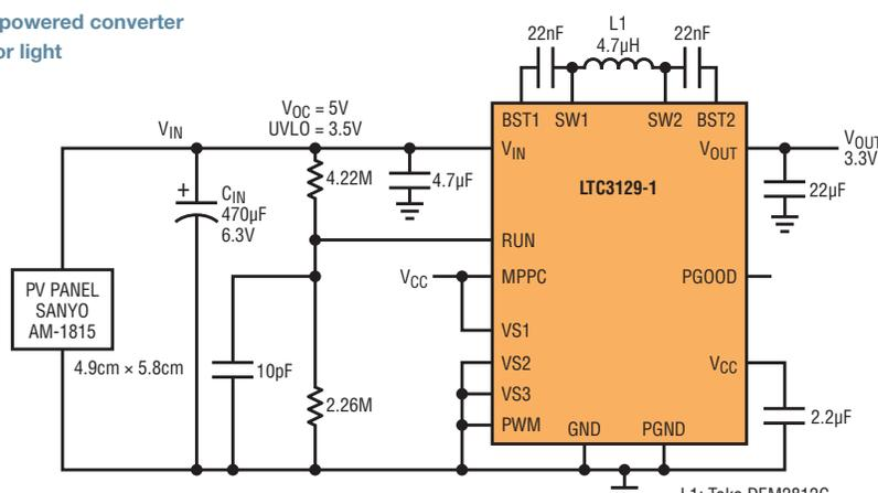
The LTC3129 and LTC3129-1 can start up and operate from an input power source as weak as 7.5 microwatts—making them capable of operating from small (less than 1in<sup>2</sup>), low cost solar cells with indoor light levels less than 200-lux. This enables such applications as indoor light powered wireless sensors.
