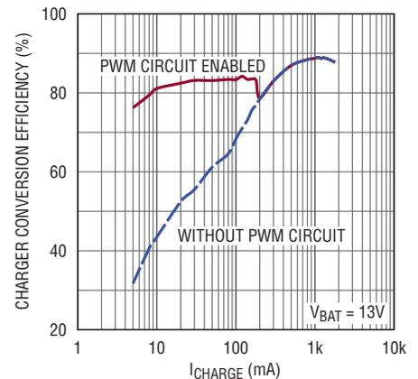
Figure 7. Efficiency curve for circuit in Figure 6
