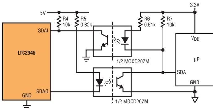
Figure 9 Opto-isolation of a 1.5kHz I<sup>2</sup>C interface between the LTC2945-1 and a microcontroller
