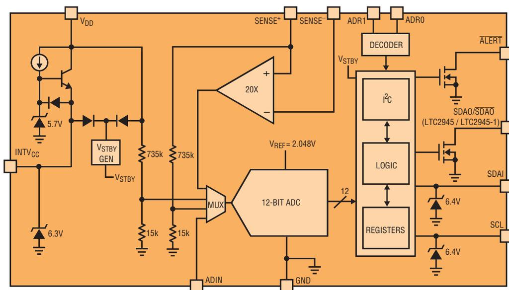
The LTC2945 is a highly integrated power monitor that easily fits into a wide range of systems. It offers a 0V to 80V common mode range, 2.7V to 80V operating range,  $\pm 0.75\%$  accurate voltage and current measurements, and an on-chip digital multiplier that computes power.
