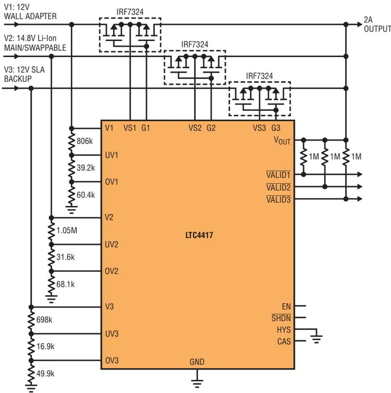
**PRIORITY SWITCHING FROM 12V MAIN SUPPLY TO 14.8V BATTERY BACKUP**
