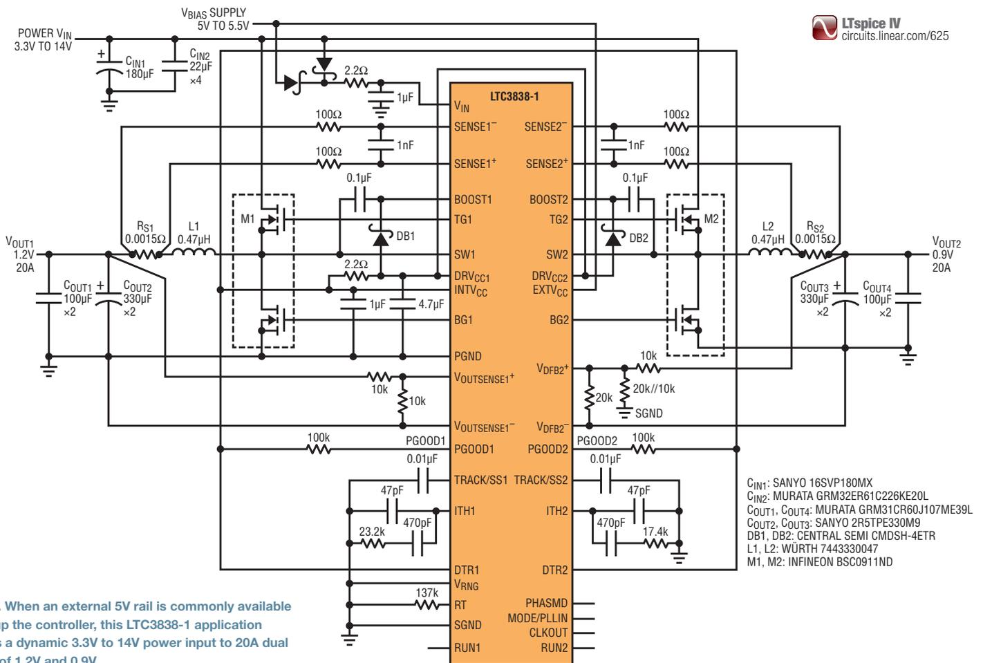
Figure 5. When an external 5V rail is commonly available to bias up the controller, this LTC3838-1 application converts a dynamic 3.3V to 14V power input to 20A dual outputs of 1.2V and 0.9V.
