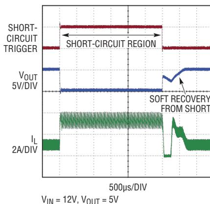
Figure 3. Short-circuit operation including soft recovery from short
