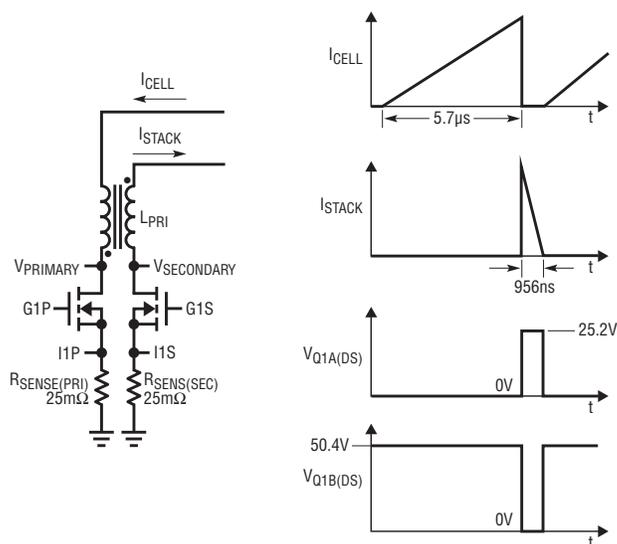
Figure 2. Discharge mode of a single cell in the stack
