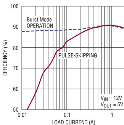
Figure 1. LTC3864 pulse-skip and Burst Mode efficiency
