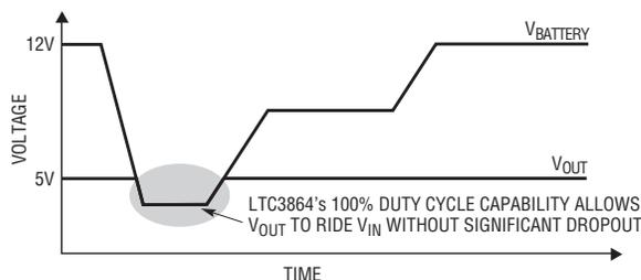
dropout during a cold crank condition. Figure 2 shows how the regulated 5V output drops out and recovers during a cold crank condition. The output simply tracks the input voltage under the output regulation voltage. The output quickly recovers to the regulated 5V once the cold crank condition is over.
