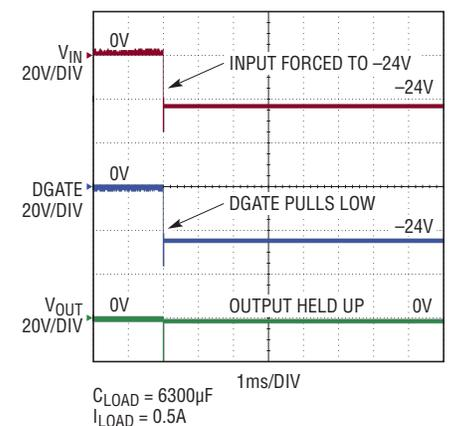
The LTC4364 also guards against overloads and short circuits, withstands output voltage reversal, holds off the MOSFETs in input undervoltage conditions and inhibits turn-on or auto-retry in input overvoltage conditions. A shutdown mode reduces the supply current to as low as 10 $\mu$ A.
