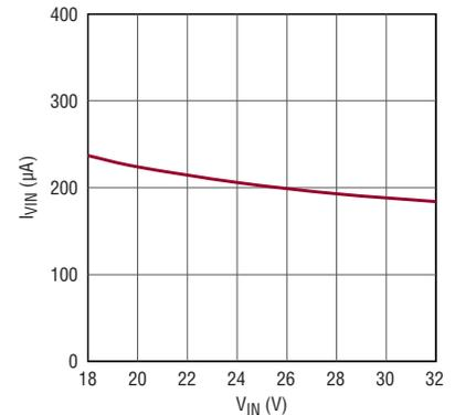
Figure 9. No-load input standby current of the 3.3V application in Figure 8
