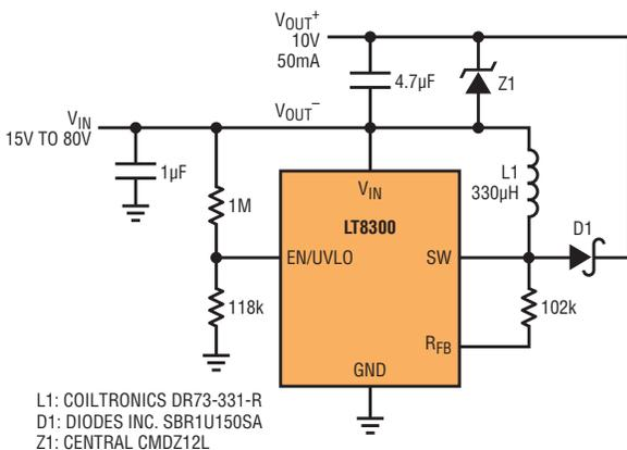
Figure 11. A  $v_{IN}$  to  $(v_{IN} - 10V)$  micropower converter
