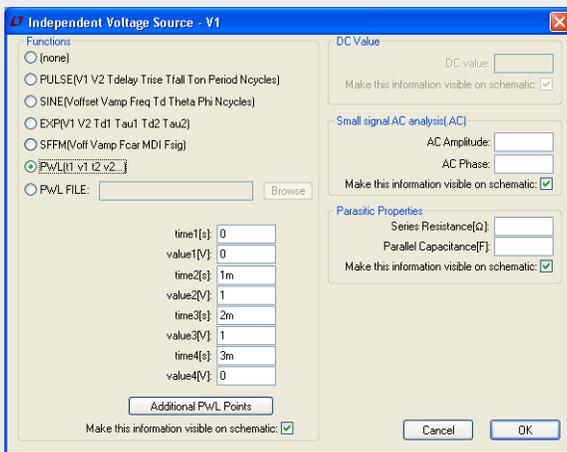
The list of two-dimensional points that represent time and value data pairs can be encapsulated in a file and used in a PWL statement:
