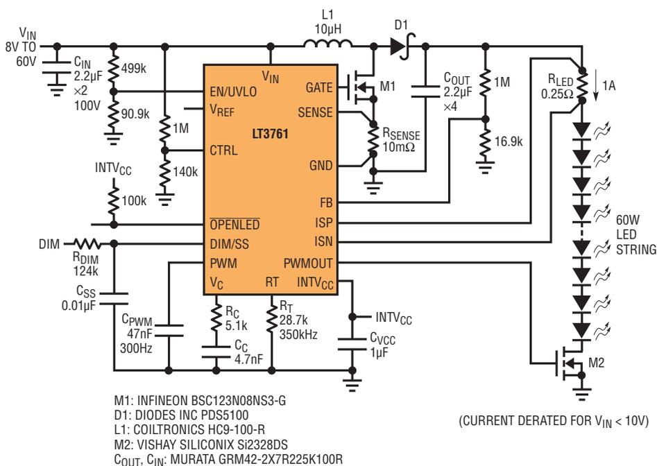
The LT3761 generates its own PWM signal to achieve accurate PWM dimming, but with the simple control of analog dimming. High dimming ratios are possible by adjusting a simple DC signal at its dimming input—no additional PWM-generating microcontrollers, oscillators or signal generators are required.
