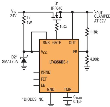
The LT4356 has a rated maximum of 100V with an operating voltage range of 4V to 80V, but a little extra circuitry enables it to protect against transients as high as 300V.
