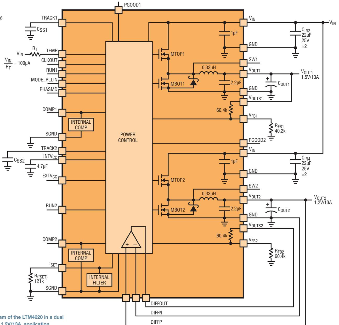
Figure 4. Block diagram of the LTM4620 in a dual output, 1.5V/13A and 1.2V/13A, application
