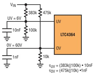
Figure 7. LTC4364 input protection:
