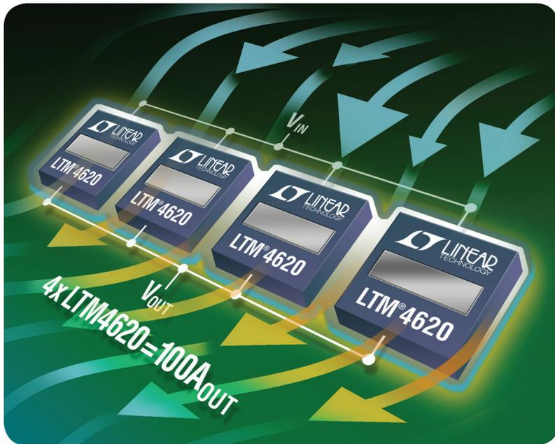
The LTM<sup>®</sup>4620  $\mu$ Module<sup>®</sup> regulator enables high current power supplies to fit tight spaces. Thermal management is built into the package to prevent hot spots on the board, a common problem with POL power supplies.
