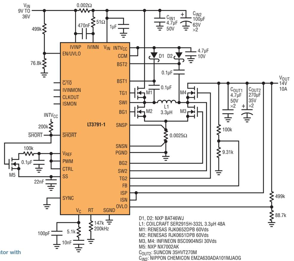
Figure 3. 140W (14V, 10A) CCM buck-boost voltage regulator with 9V-56V input has output OVLO for transient protection.
