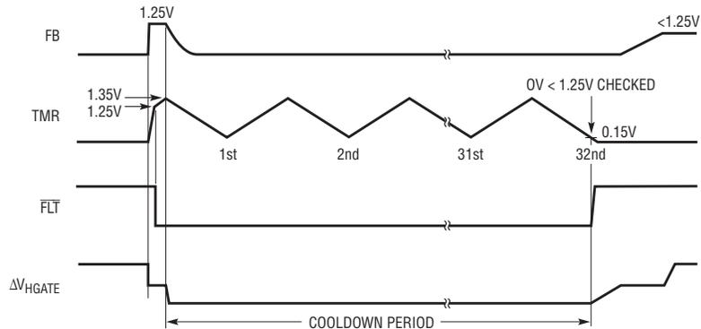
output short-circuit condition lasts for a shorter time interval than a brief, minor overload, helping ensure the MOSFET operates within its safe operating area.
