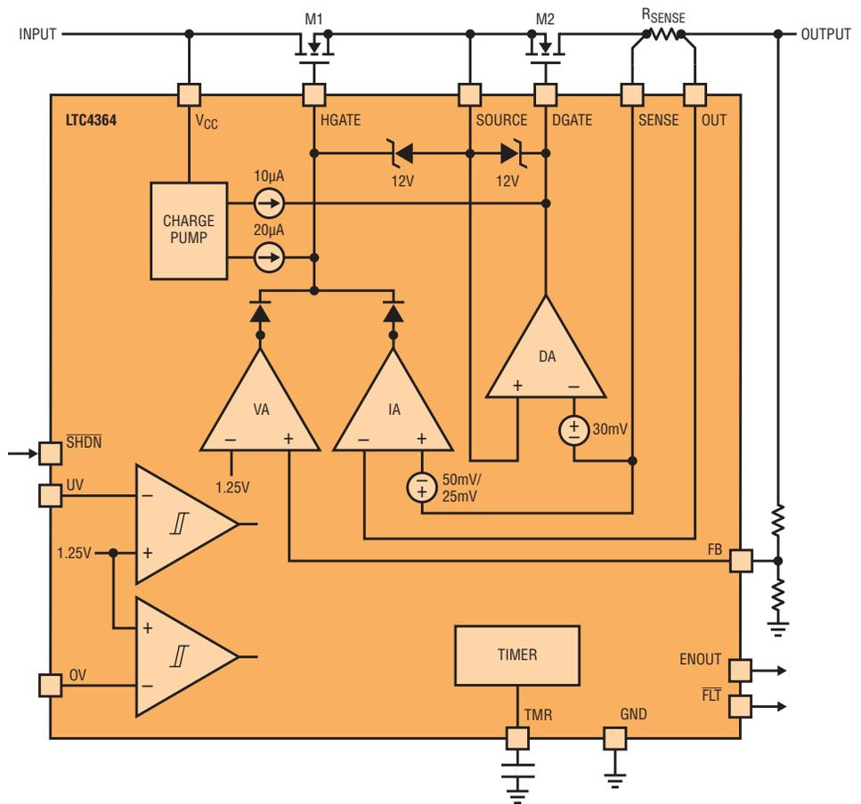
Figure 1. Simplified block diagram of the LTC4364
