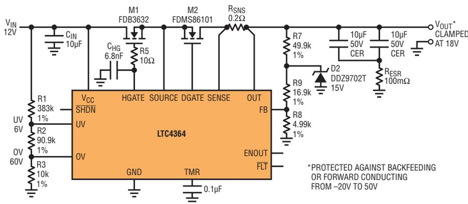
Figure 8. LTC4364 offers built-in output port protection against overvoltage, short or reverse voltage.
