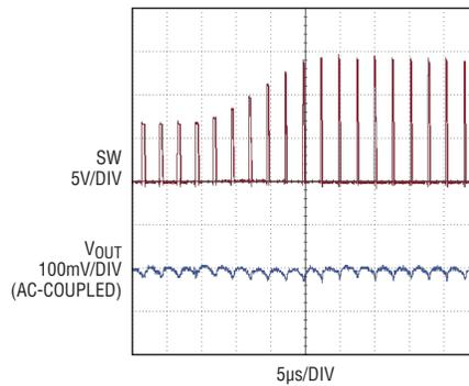
**Figure 7.** Through its VINSNS pin, the LTC3860 provides line feedforward compensation, preventing steady state and dynamic variations in V<sub>OUT</sub> when V<sub>IN</sub> is not constant.
