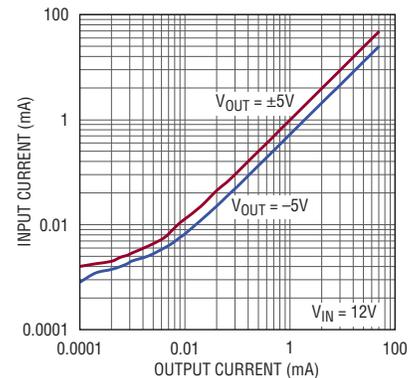
The LTC3388-1 and LTC3388-3 are high efficiency step-down regulators that draw only 720nA (typ) of DC current at no load while maintaining output regulation. They are capable of supplying up to 50mA of load current and contain an accurate undervoltage lockout (UVLO) feature to maintain a low quiescent current when the input is below 2.3V.
