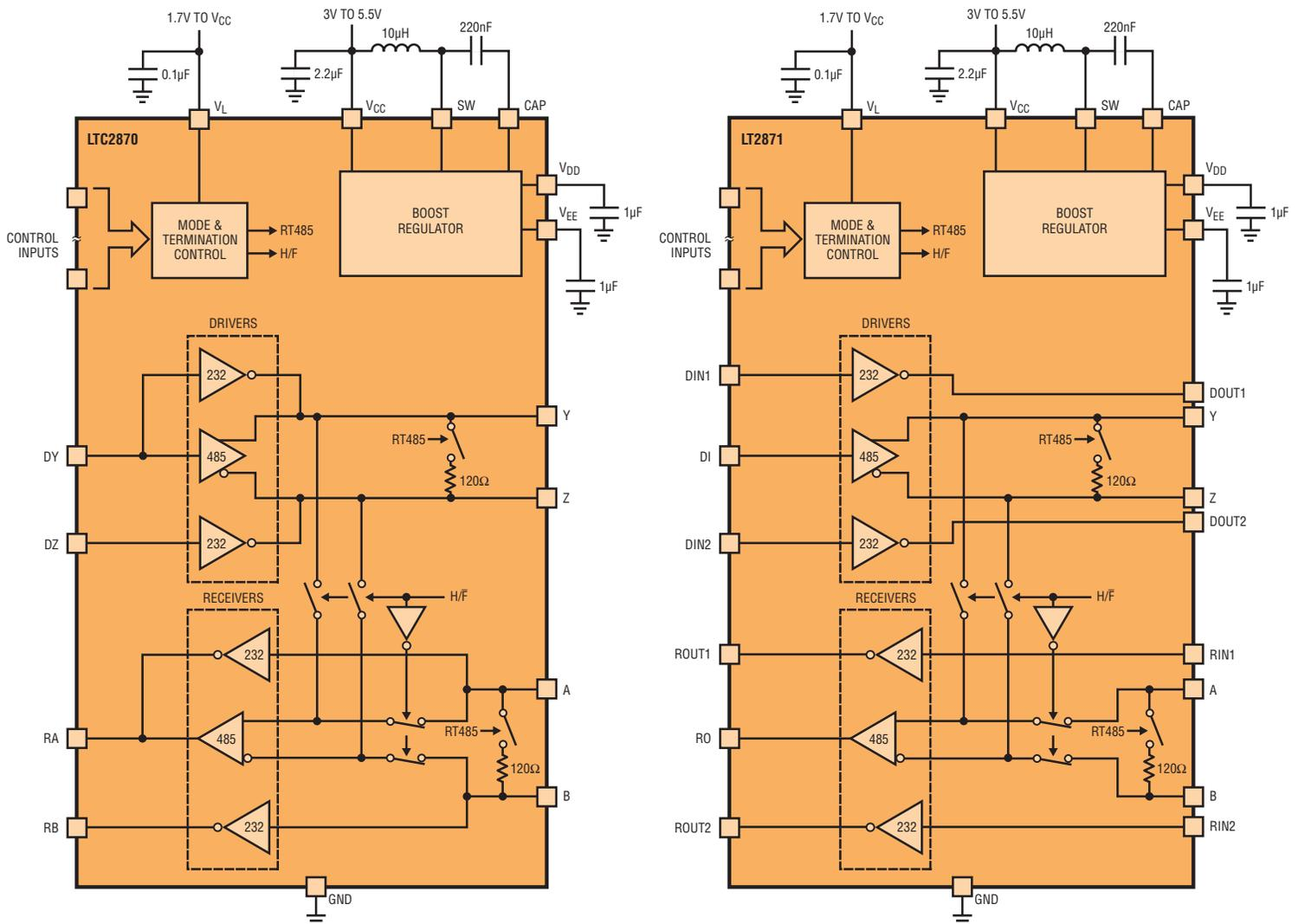
Figure 3. The LTC2870 configured for RS232 (a) or RS485 (b) communications. The RS485 configuration also shows the RS485 termination resistors optionally switched in with the TE485 pin tied high.
