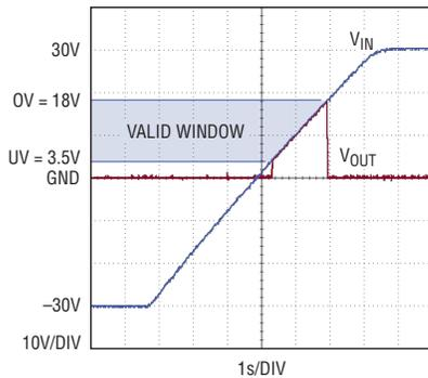
Figure 2. Load protection as  $V_{IN}$  is swept from -30V to 30V
