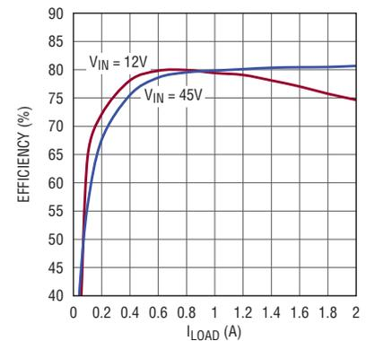
Figure 5. Efficiency of the converter in Figure 4
