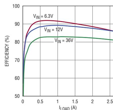
Figure 3. Switching regulator efficiency
