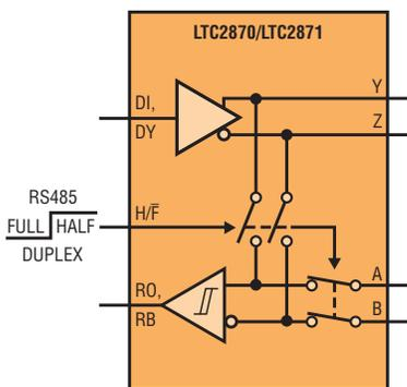
Figure 14. Logic loopback control in the LTC2871. Loopback works whether or not the drivers are enabled.
