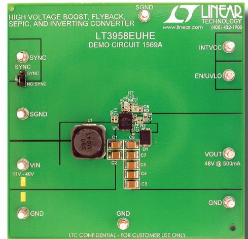
Figure 1. A 10V–40V input, 48V output boost converter board
