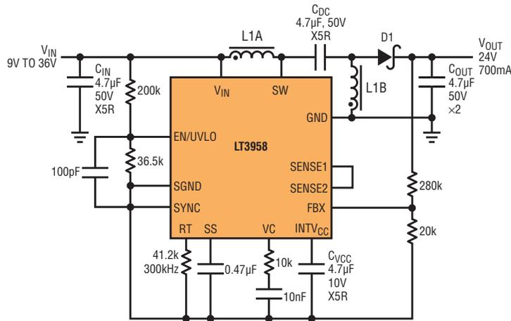
C<sub>IN</sub>, C<sub>OUT</sub>, C<sub>DC</sub>: MURATA GRM32ER71H475KA88L
