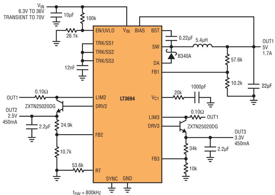
The LT3694/LT3694-1 combines a 2.6A switching regulator and two 500mA low dropout linear regulators in a compact 4mm × 5mm QFN package or a thermally enhanced TSSOP.
