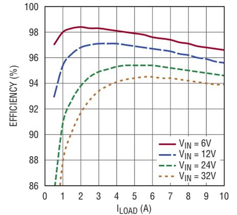
Figure 6. Efficiency of the 5V, 10A converter
