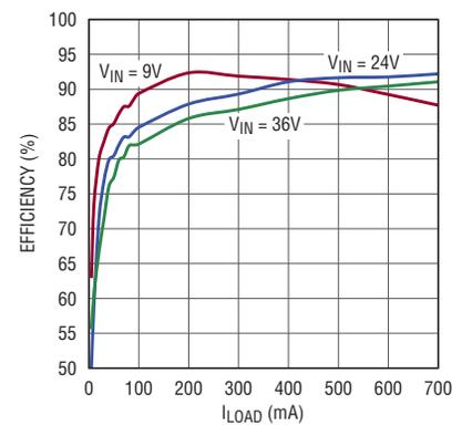
Figure 7. Efficiency of the converter in Figure 6.
