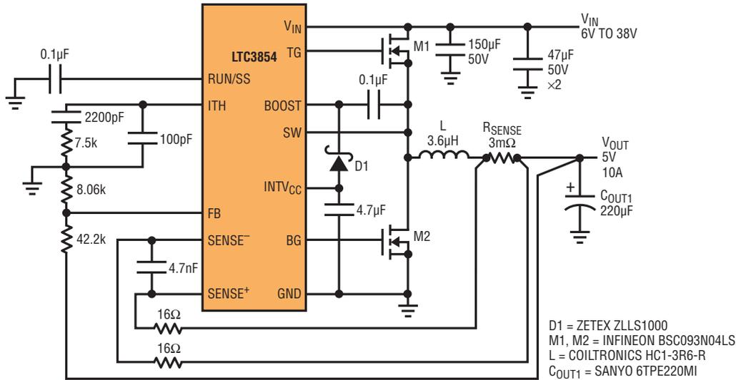
Figure 5. 5V, 10A converter with a 6V to 38V input voltage range
