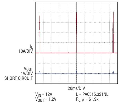
**Figure 8.** Short circuit behavior of the LTC3860
