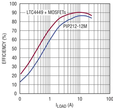
**Figure 6.** The circuit of Figure 5 shows improved efficiency compared with a typical DrMOS solution. The compromise is in board space—a DrMOS occupies 36mm<sup>2</sup> or 64mm<sup>2</sup>, and the driver and three MOSFETs occupy 101mm<sup>2</sup>, excluding the traces connecting the components.
