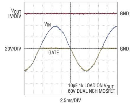
Figure 4. 36ms recovery timer blocks 28V, 60Hz AC line voltage
