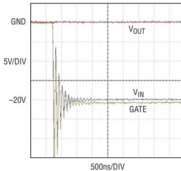
Figure 3. Hot swapping  $V_{IN}$  to -20V
