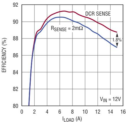
Figure 3. Efficiency of the converter with a sense resistor versus efficiency with DCR sensing. By eliminating the sense resistor, the full load efficiency goes up by almost 2%.
