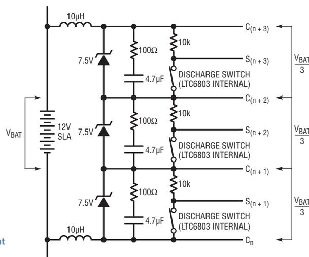
Figure 2. Voltage-divider structure for each 12V battery measurement
