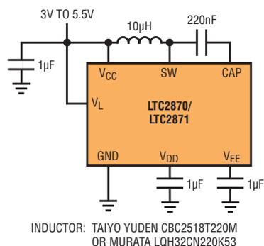
Figure 9. Typical supply connections with external components shown
