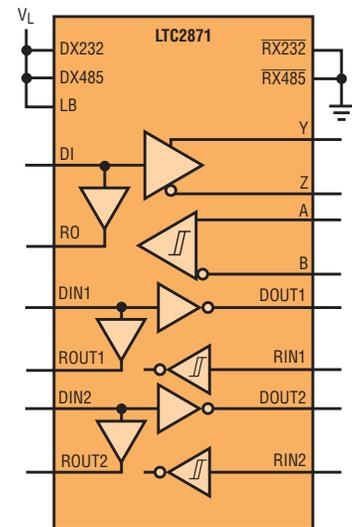
The LTC2870 and LTC2871 multiprotocol transceivers simplify the design of RS485 and RS232 systems by combining both types of transceivers on a single device. They support data rates as high as 20Mbps for the single RS485 transceiver and 500kbps for two RS232 transceivers.
