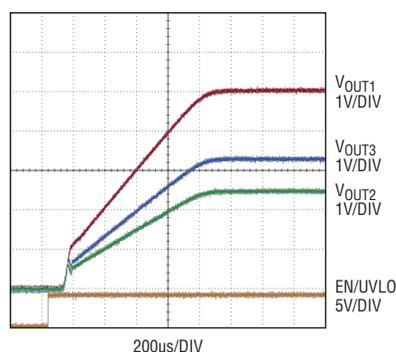
Figure 2. Ratiometric tracking waveforms
