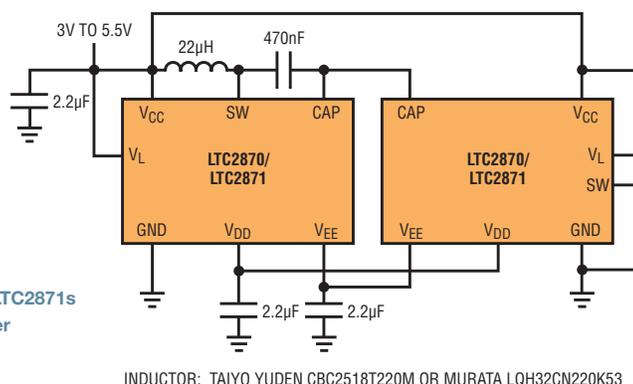
Figure 10. Running two LTC2870s or LTC2871s from a single, shared DC/DC converter
