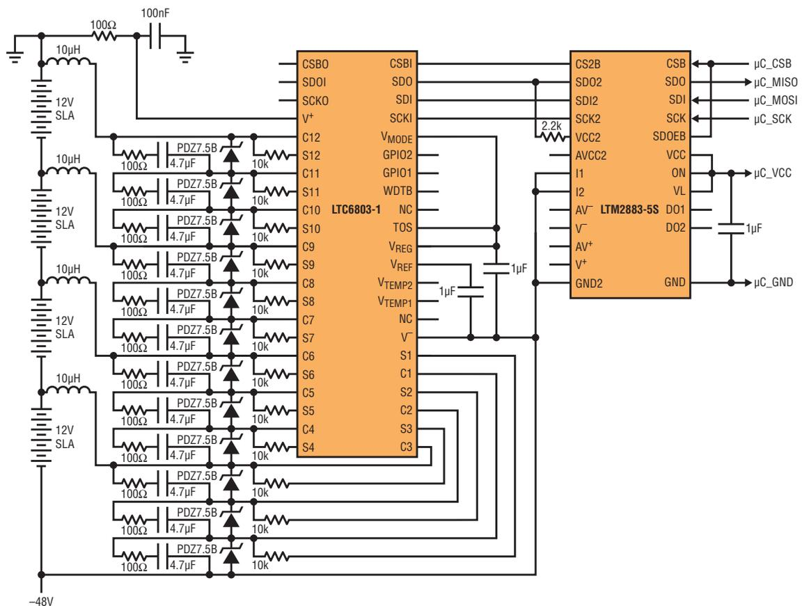
Although the LTC6803 is ostensibly designed to monitor lithium-based battery systems, it can also be used to support traditional –48V lead-acid battery stacks.
