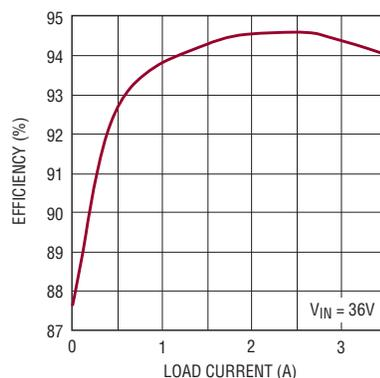
Figure 3. Efficiency of the converter in Figure 1 for the V<sub>OUT2</sub> 8.5V channel
