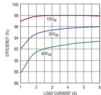
Figure 4. Efficiency of the LTC3890 configured as a 2-phase single output of 8.5V at up to 6A
