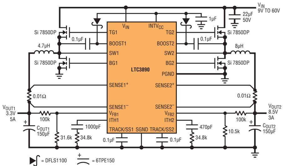
Figure 1. High efficiency dual 8.5V/3.3V output step-down converter
