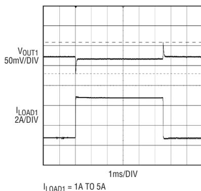
Figure 2. Transient response of 3.3V channel
