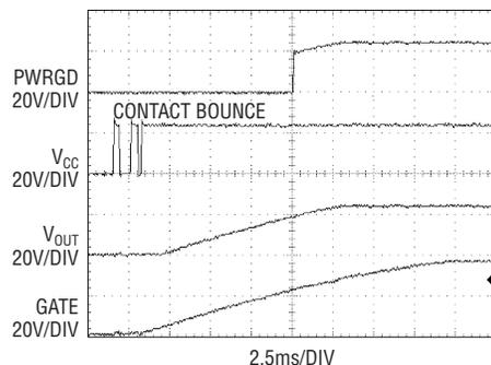
Figure 2. Startup waveforms
