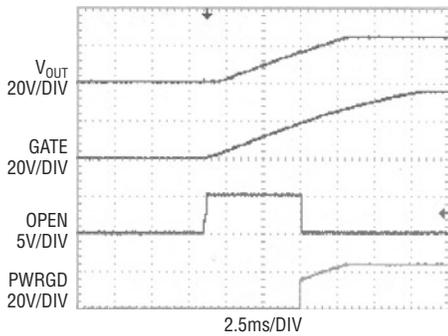
Figure 6. Normal MOSFET start-up waveforms
