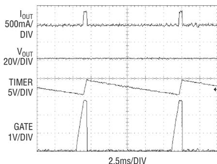
**Figure 4. Retry waveforms**
