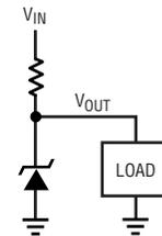
Figure 7. Typical shunt voltage reference configuration
