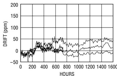
**Figure 2. LT1790S6-2.5V SOT-23 long-term drift (three separate units)**
