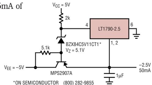
Figure 8. -2.5V negative 50mA series reference
