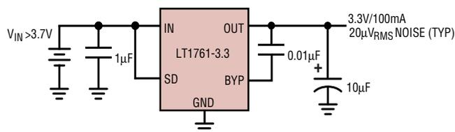
Figure 1. New low noise, low dropout, micropower regulator
