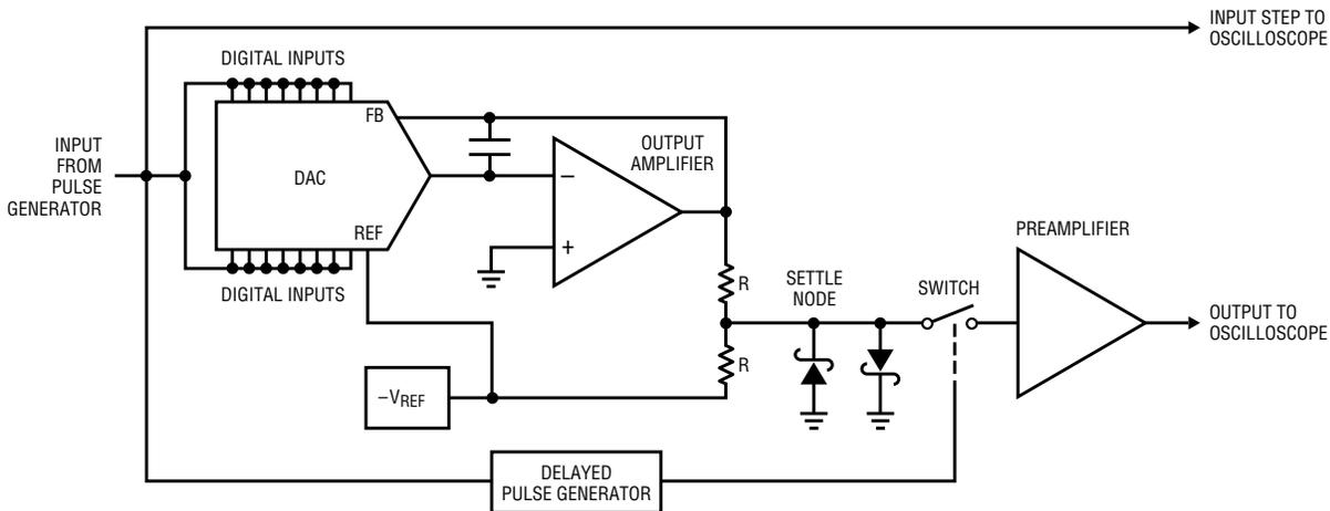
**Figure 3. Conceptual arrangement eliminates oscilloscope overdrive. A delayed pulse generator controls the switch, preventing the oscilloscope from monitoring settle node until settling is nearly complete.**
