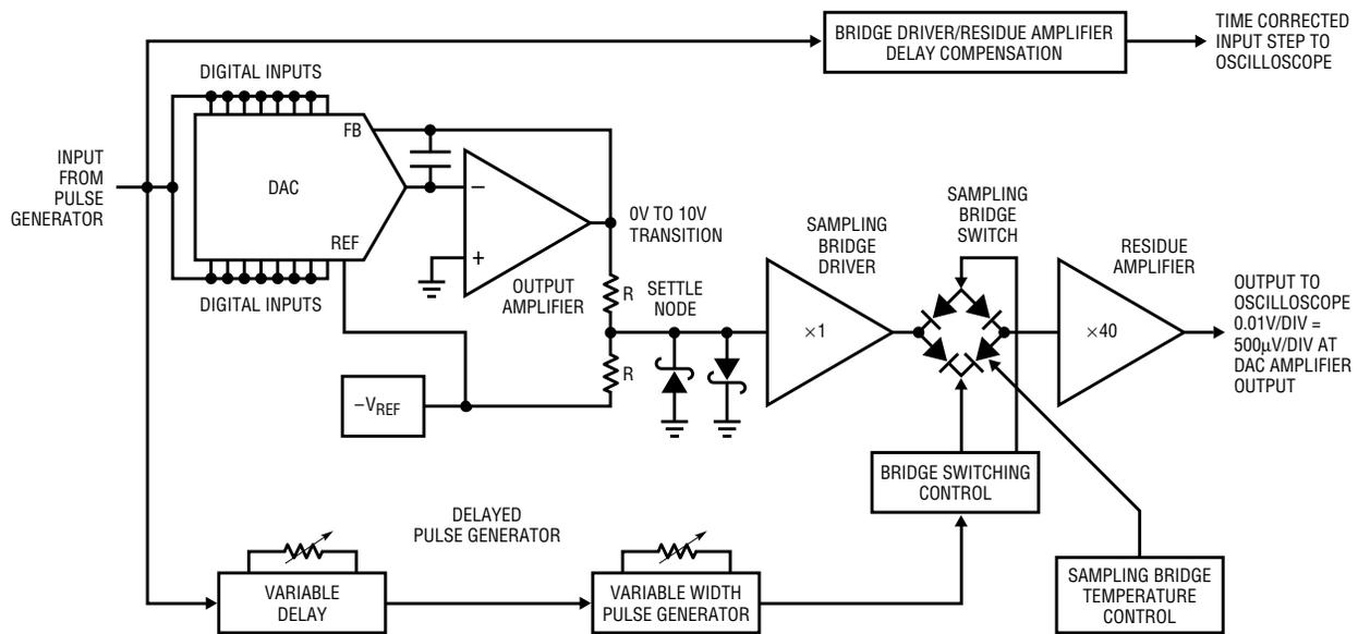
**Figure 4. Block diagram of DAC-settling-time measurement scheme: diode bridge switch minimizes switching feedthrough, preventing residue-amplifier oscilloscope overdrive. Temperature control maintains 10 $\mu$ V switch offset baseline. Input step-time reference is compensated for  $\times 1$  and  $\times 40$  amplifier delays.**
