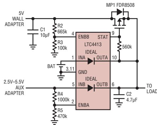
Figure 8. Automatic switchover from a battery to an auxiliary supply or a wall adapter
