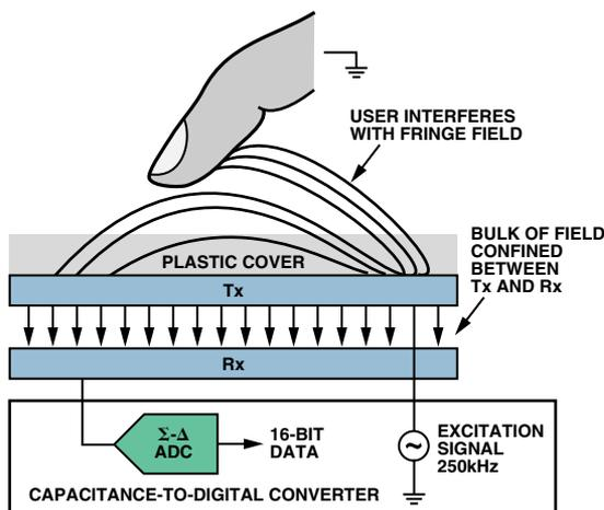
Figure 1. Sensing capacitance.
