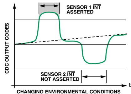
Figure 5. Sensor activation with changing ambient capacitance.
