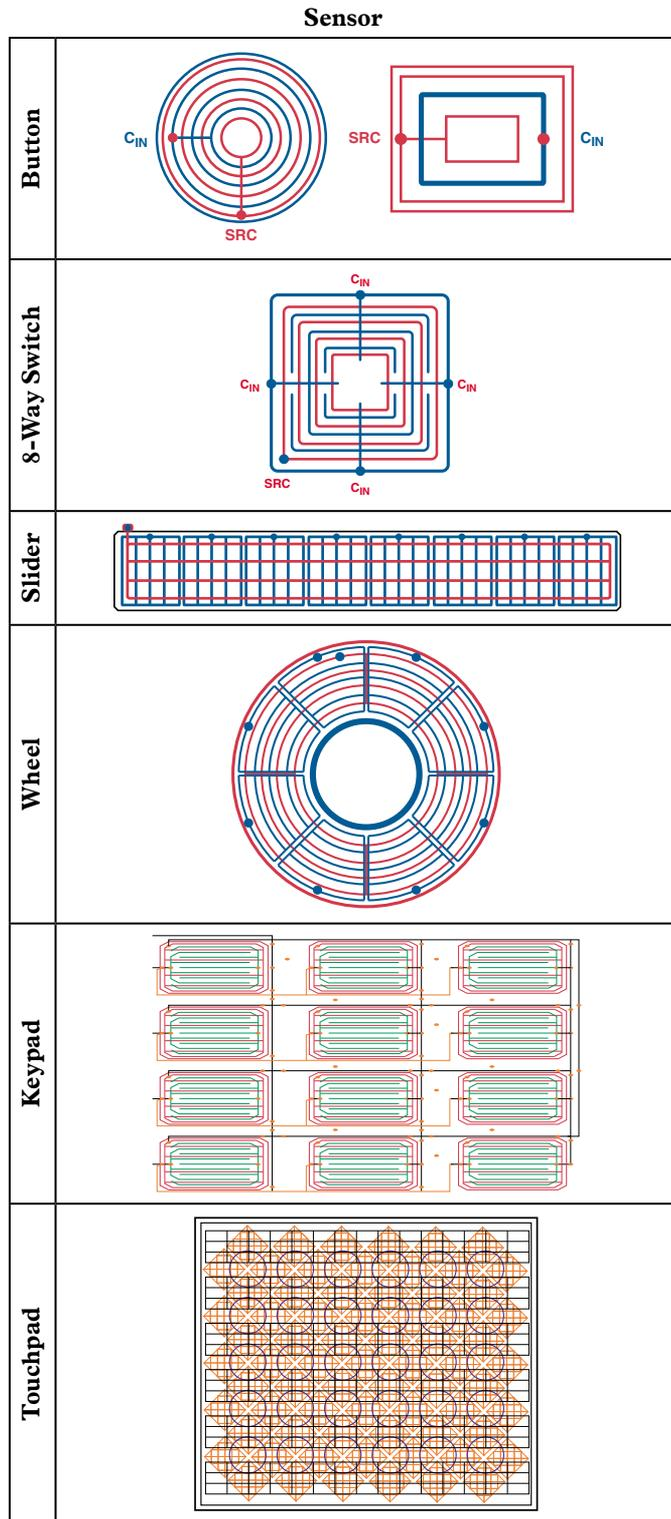
Figure 7. Selection of capacitance sensors.
